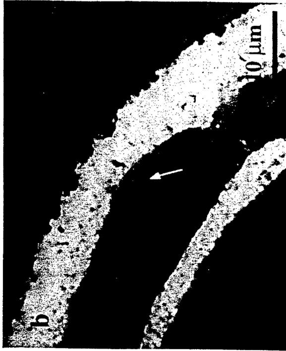
Fig. 2 SEM micrograph of multilayer-coated fiber in as-hot pressed composite.
