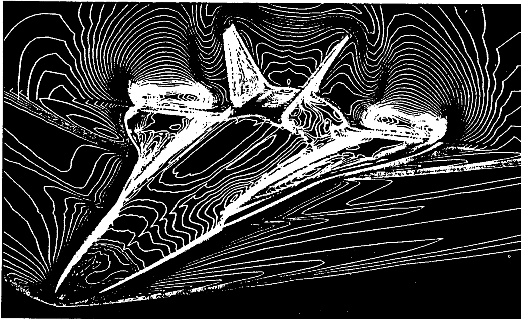
▼Numerically-simulated airflow around a space plane model
