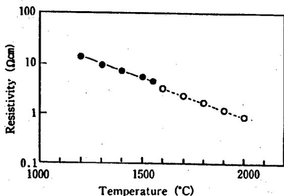
●-●: measured by normal two-probe direct current method.
