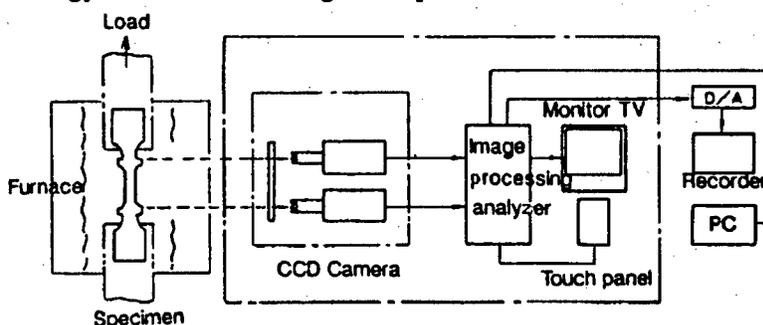
Figure 4. Schematic Illustrations of Strain Measurement Methodology
