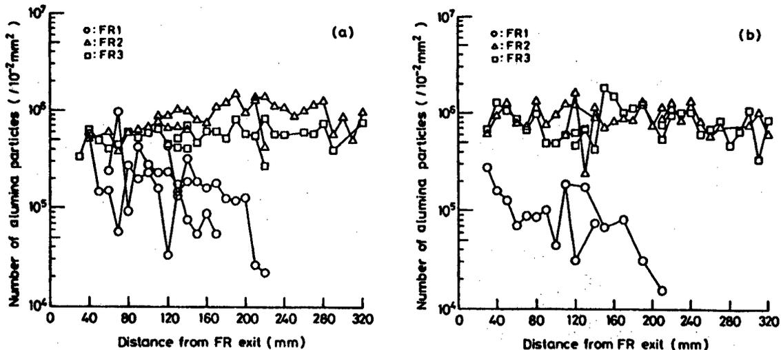
Figure 4. Density of Collected Al<sub>2</sub>O<sub>3</sub> Fine Particles (diameter: D ≤ 0.1 μm) Vs. Distance From the Feed Ring Exit (The particles are collected at (a) 760 Torr and at (b) 100 Torr.)
