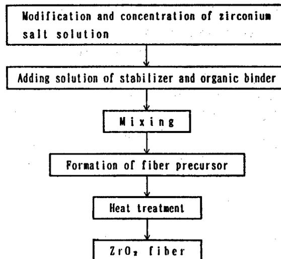
Figure 7. The Producing Process of ZrO<sub>2</sub> Fiber
