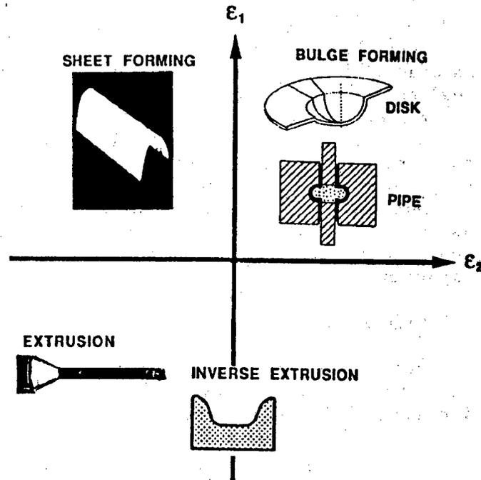
Figure 6. Examples of Superplastic Forming for Y-TZP
