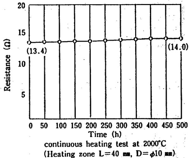
Figure 20. Electric Resistance Variation of the Zirconia Form in Continuous Heating
