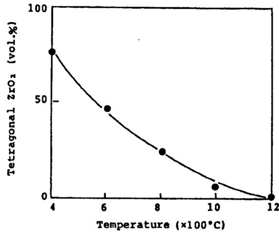
Figure 11. Phase Transformation of Zirconia Fiber Precursor Without Stabilizer
