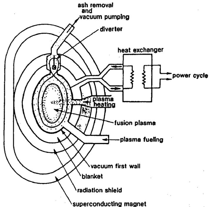
Figure 6. Schematic View of Components for Fusion Reactors
