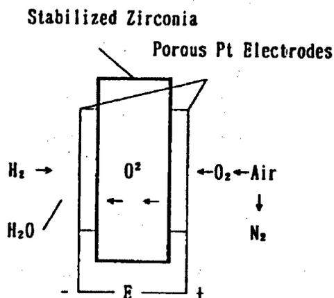
Figure 5. Fundamental Principle of a Zirconia Fuel Cell
