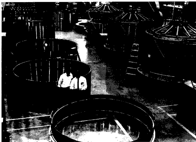
The stainless steel sheets have been welded into bands, which are then welded to each other to form the tank of the Atlas missile. A single band is shown in the foreground; multiple band units are shown behind it. At right are the fixtures that hold the strips rigid until they are assembled into the completed tank. Source: Naval Institute Photographic Library, Annapolis, MD, file "Weapons: U.S.: Missile: Atlas."
