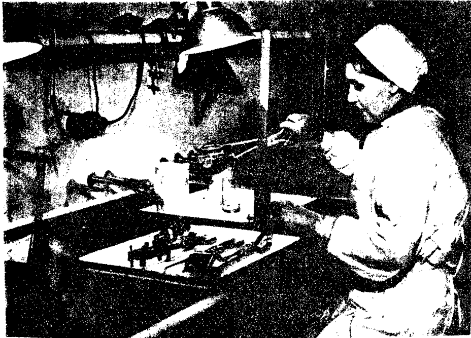
Fig. 9. Experiment with gamma active material. The work is carried out with the remote-control equipment behind a safety lead shield.
