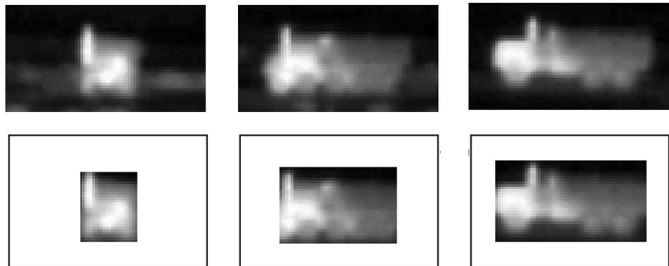
Figure 5. Background clipping of several input images. (Top) Original images of a truck viewed at  $0^\circ$ ,  $45^\circ$ , and  $90^\circ$ , respectively. (Bottom) Corresponding extracted target areas after proper background removal.
