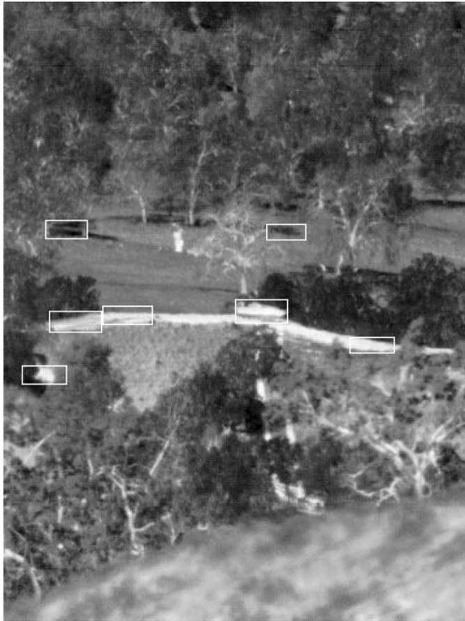
Figure 1. An example FLIR image taken in a typical environment. Boxes indicate potential target areas detected by ARTM algorithm.
