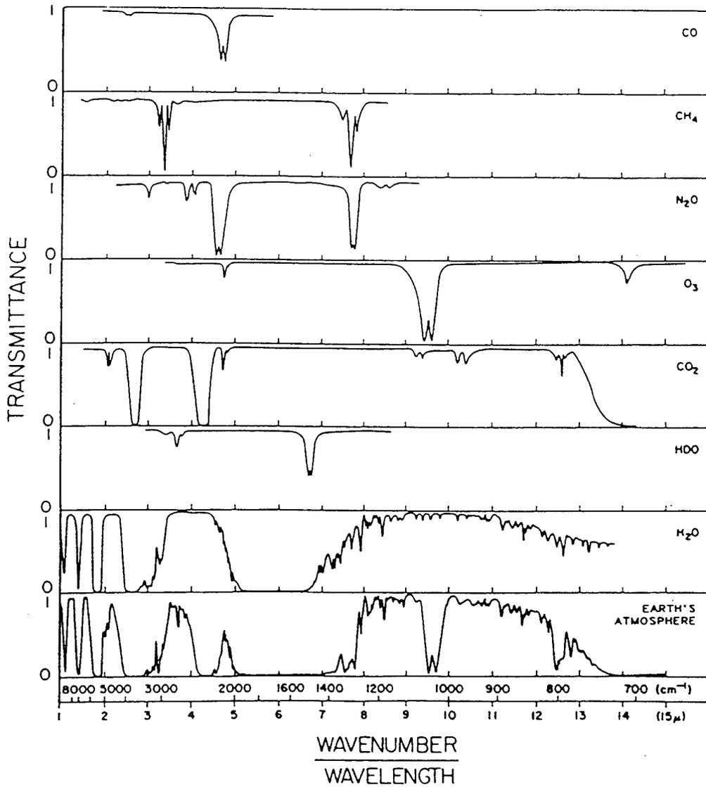
**Figure 10. Infrared Transmittance of Several Gases in the Earth's Atmosphere and Combined Total Atmospheric Transmittance (from Kidder and Vonder Haar, 1995).**
