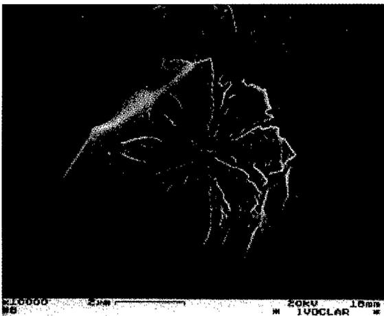
Fig. 3. Crystallization of leucite, originating from a nucleating centre. Petal-shaped growth pattern: SEM.
