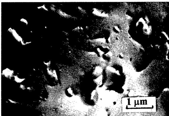
Fig. 6. TEM micrograph of glass 3, containing 30 mol%  $B_2O_3$ , after thermal treatment at 600°C.
