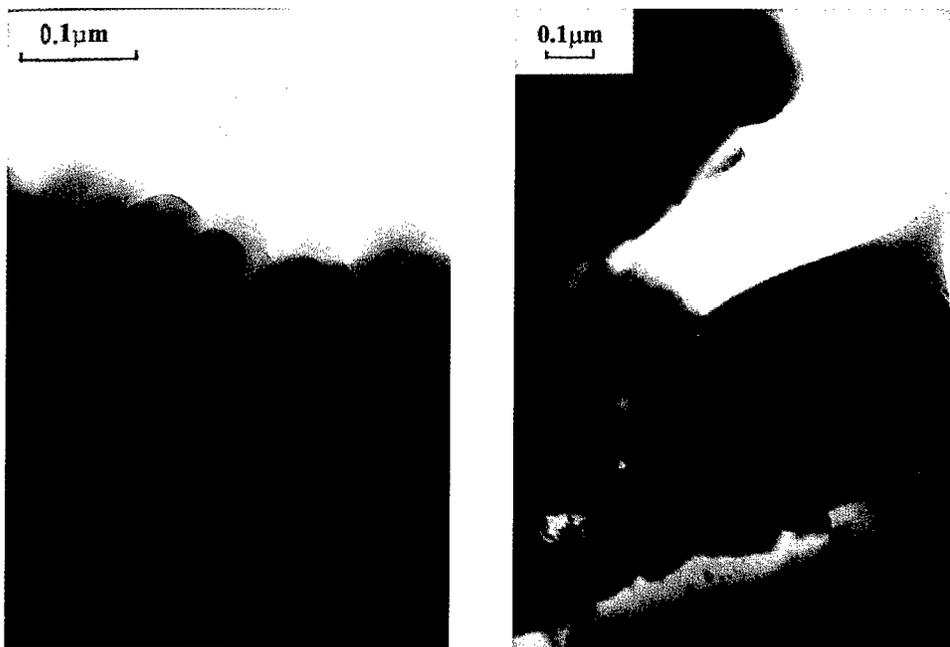
Fig. 1. (Left) TEM micrograph of the  $55\text{B}_2\text{O}_3.45\text{SiO}_2$  gel sample, after heating at  $600^\circ\text{C}$ , and (Right) TEM micrograph of the  $50\text{TeO}_2.10\text{B}_2\text{O}_3.40\text{SiO}_2$  glass sample.
