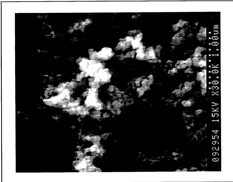
Fig. 2- Shown is a SEM photograph of sample 2, amorphous boron from Krier, with a magnification of 30,000x.
