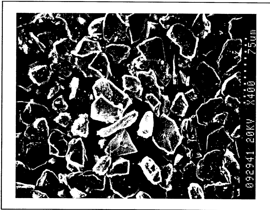
Fig. 7(a)-Shown is a SEM photograph of sample 7, sieved crystalline boron from Krier, with a magnification of 400x.
