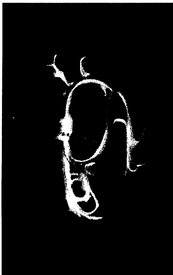
Fig.13. A streamer initiated MW discharge ( p = 75 Torr; E_0 = 2 kV/cm; \tau = 36 \mu s; 2a = 2,5 mm)
