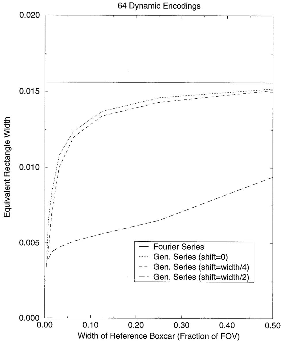
Figure 8: PSF vs Width of Reference Boxcar: This plot shows the relationship between the width of the PSF and the width of the reference boxcar for Fourier-keyhole (or, equivalently, the zero-padded Fourier series) and RIGR for three locations of the point change. The simulations to generate this plot used 64 dynamic encodings.
