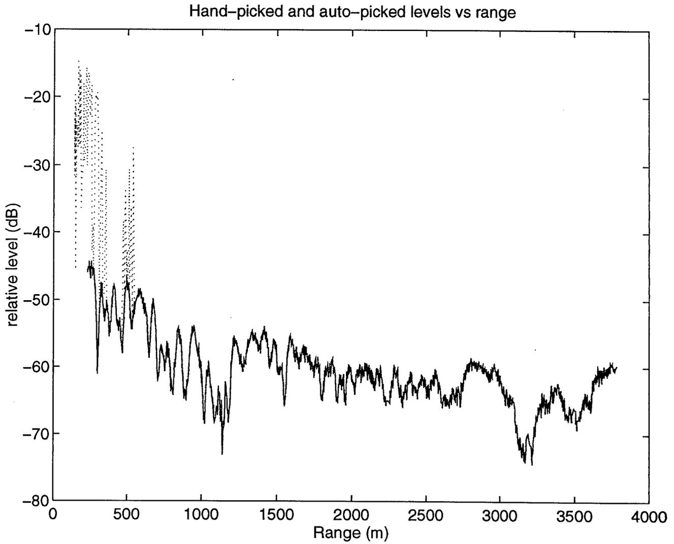
Figure 9. Magnitude of the pressure as a function of range. The lower, black curve is the result of the hand-picked data; the upper (red) curve (noisy near short ranges) is the result of the automatic peak-picker.
