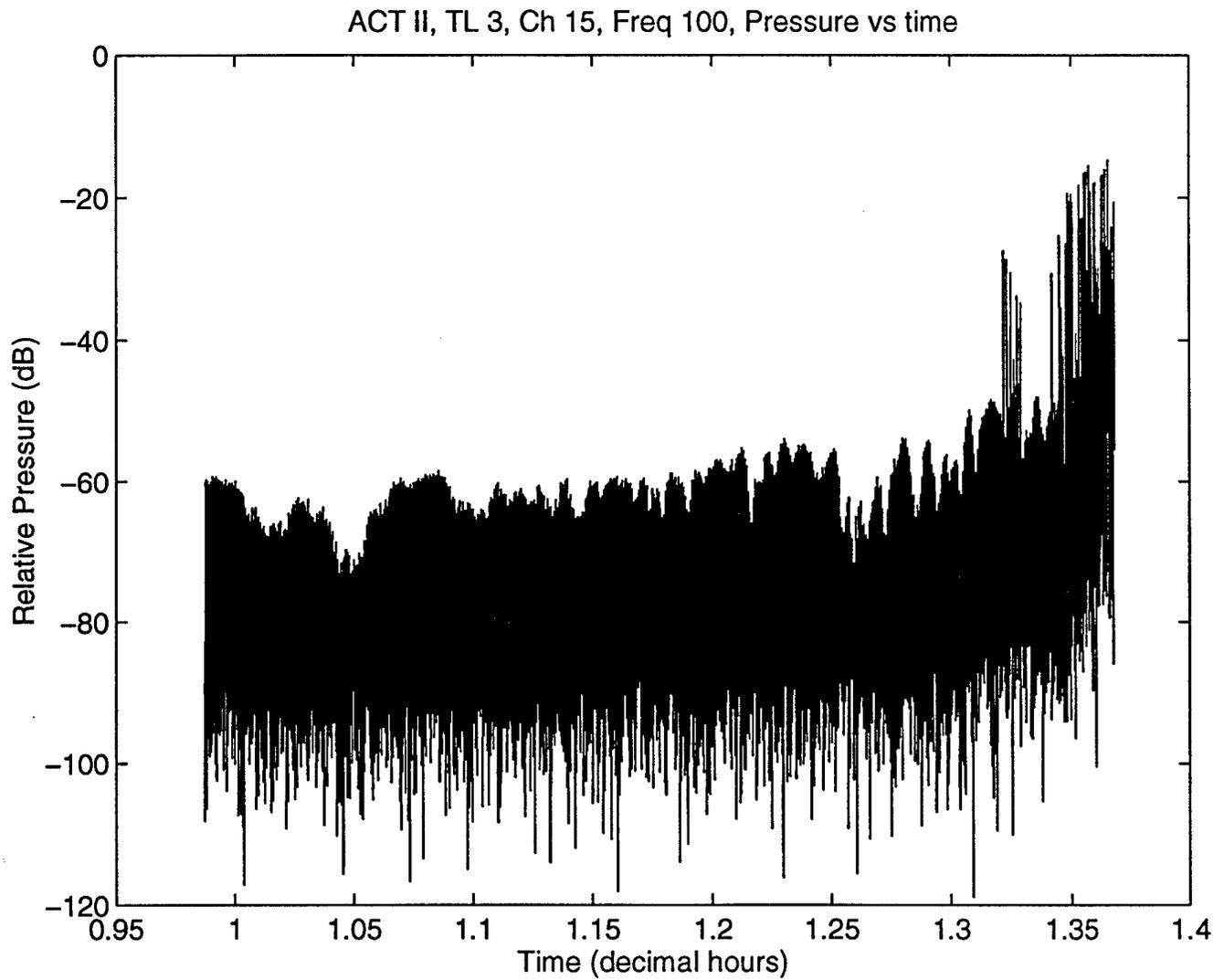
Figure 5. Relative sound pressure level from SEACAL channel 15 at 61.7 meters depth.
