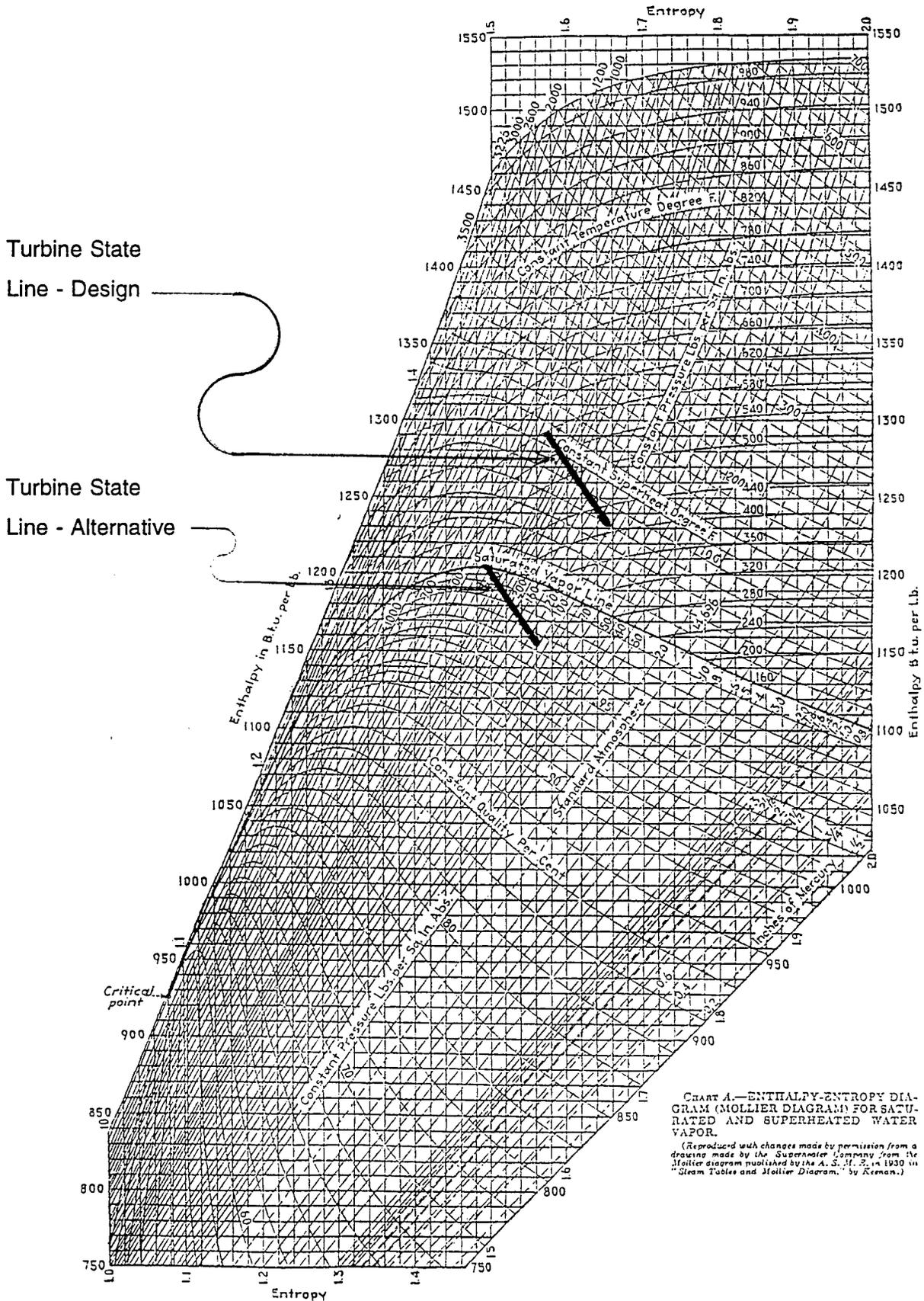
CHART A.—ENTHALPY-ENTROPY DIAGRAM (MOLLIER DIAGRAM) FOR SATURATED AND SUPERHEATED WATER VAPOR.
