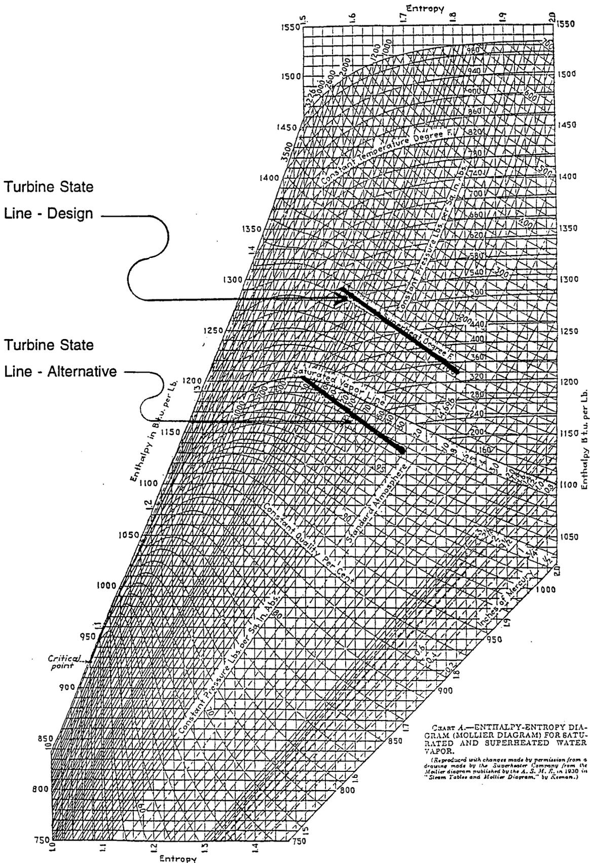
CHART A.—ENTHALPY-ENTROPY DIAGRAM (MOLLIER DIAGRAM) FOR SATURATED AND SUPERHEATED WATER VAPOR.
