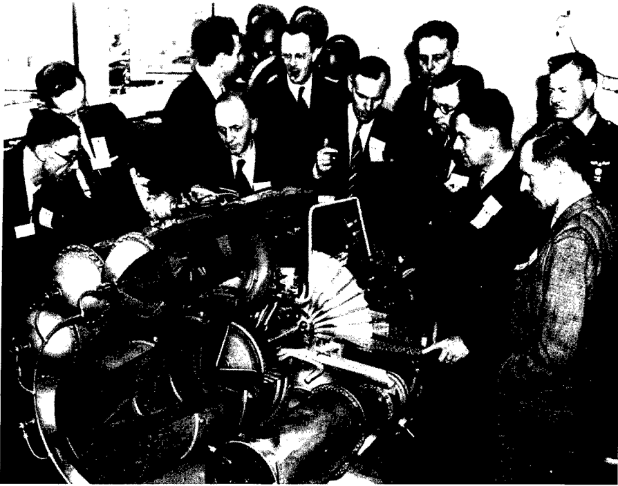
The British get a look at their modified "Whittle" engine, the A-1. GE engineers made a few modifications to the original design that increased efficiency.
