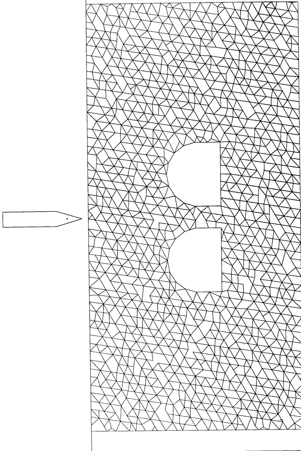
Figure 6. The penetration of a missile at a velocity of 300 meters per second into a blocky rock mass with two tunnels (continued)
