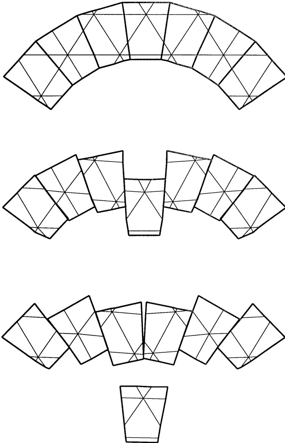
**FIGURE 9.3** The failure of a deformable arch
