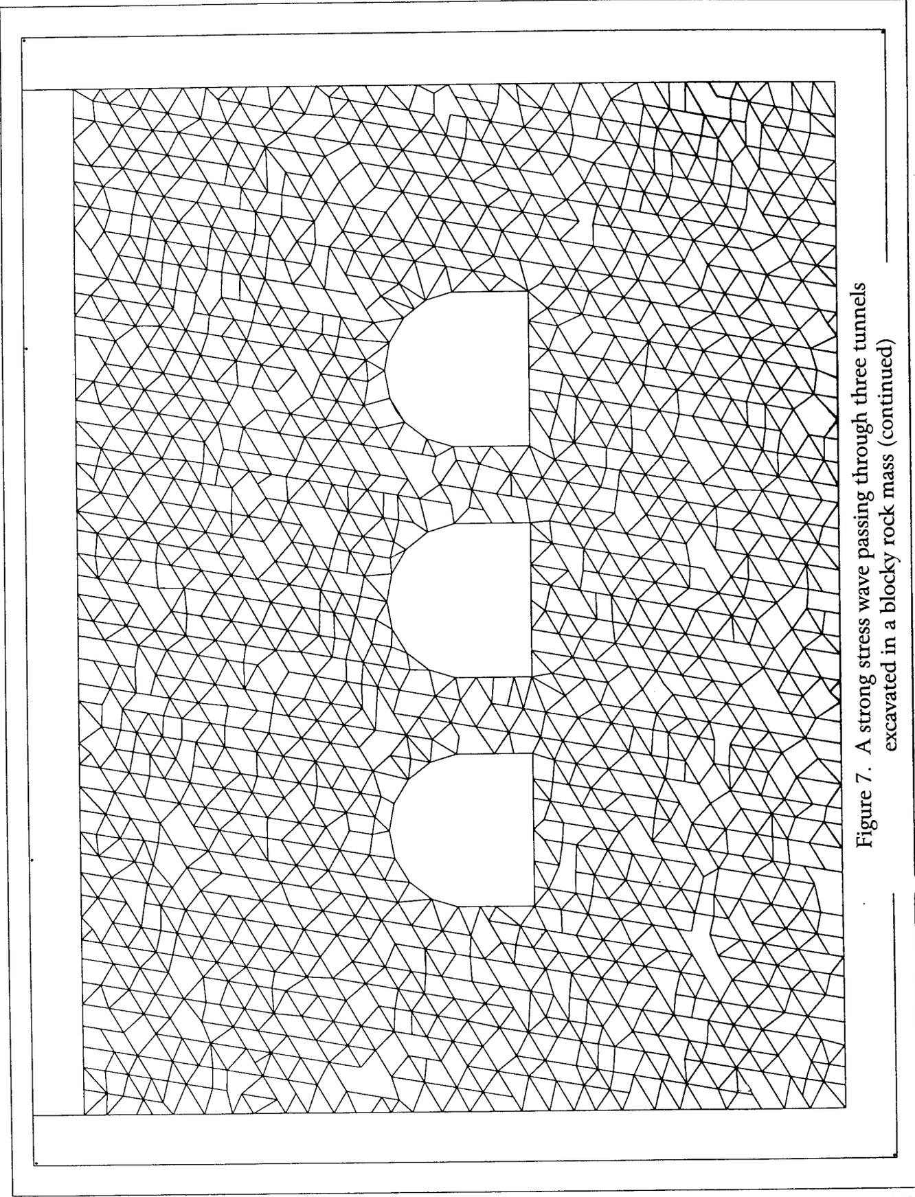
Figure 7. A strong stress wave passing through three tunnels excavated in a blocky rock mass (continued)
