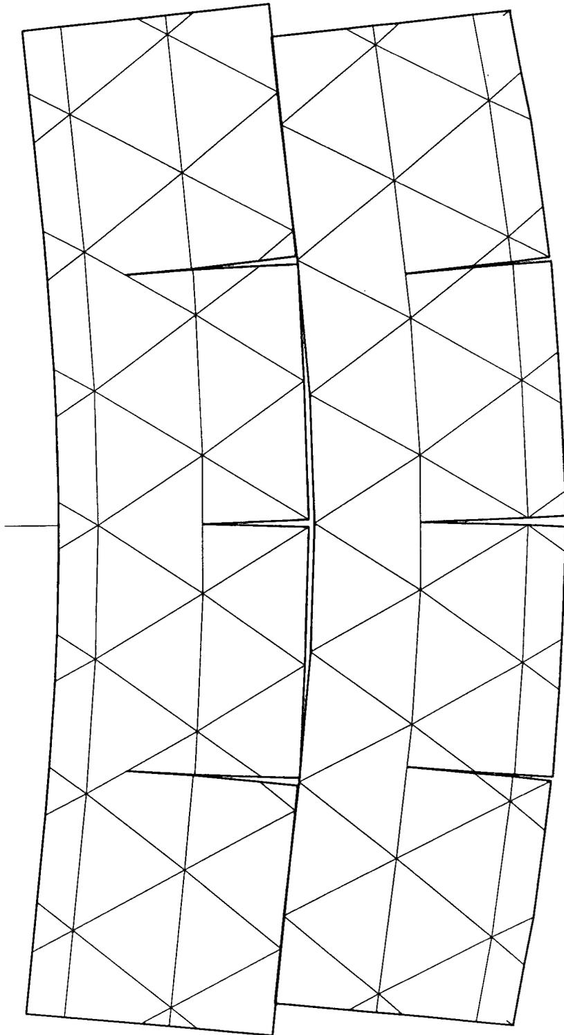
FIGURE 9.7 Deformation of double simply supported beams
