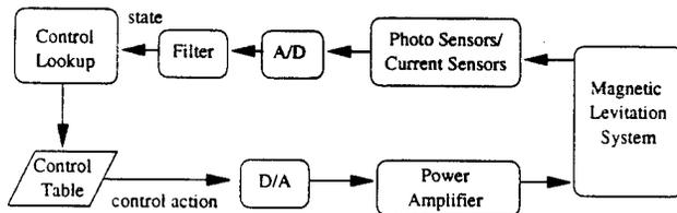
Figure 4: Block diagram for the maglev control system.
