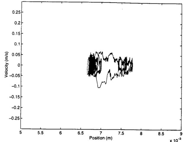
Figure 8: A sample maglev control trajectory shown in phase space (position  $\times$  velocity). The equilibrium point (0.0066, 0) is inside the dense region covered by the orbit. Notice that the global controller is able to bring the trajectory back to equilibrium after an initial disturbance.
