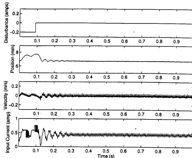
Figure 9: Experimental data from the maglev system: (a) Disturbance introduced at the beginning. (b) Air gap  $x$  vs. time. Notice that the system stabilizes after the initial disturbance. (c) Velocity  $v$  vs. time. (d) Control  $I$  vs. time. The global, phase-space controller is activated whenever the position or velocity of the ball deviates from the desired value significantly. When the system is within the capture region of the local control, the controller switches to the local control.
