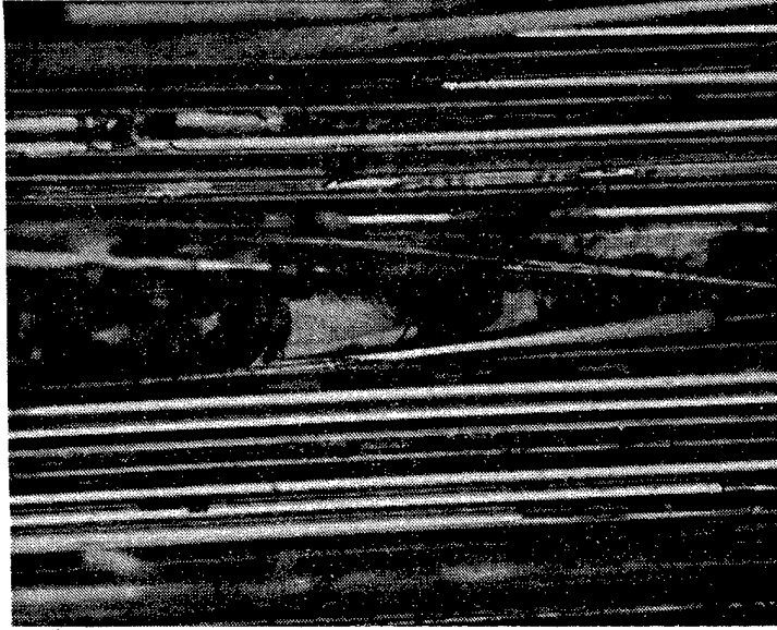
Figure 3.3-5. Optical Fractographs of PMR-15/AS4 Interlaminar Mode II (Shear) Fatigue, Room Temperature, High Stress
