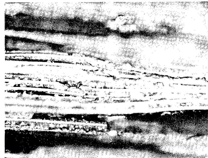
Figure 3.4-7. Optical Fractographs of a APC-2/AS4 Interlaminar Mode I (Tensile) Fatigue Fracture Surface, 250° F
