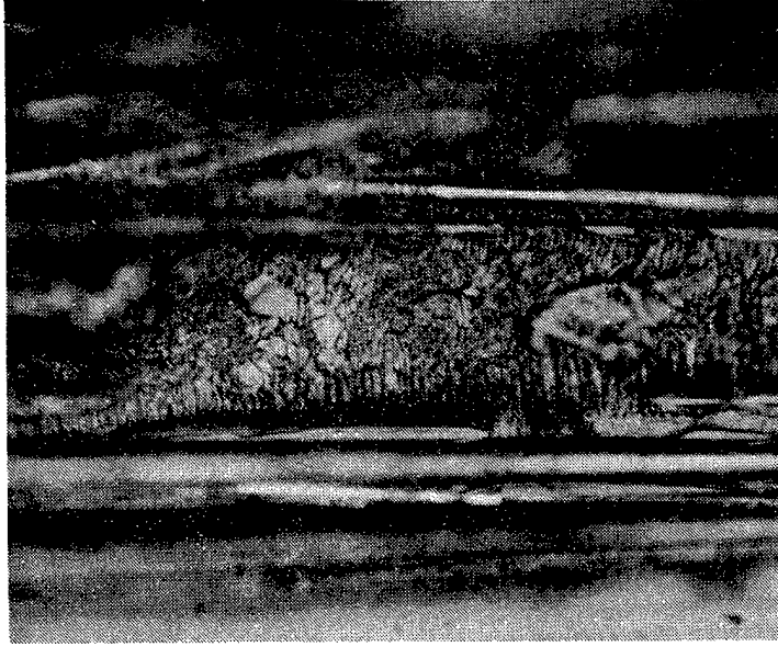
Figure 3.2-15. Optical Fractographs of KIII/AS4 Interlaminar Mode II (Shear) Fatigue, Room Temperature, High Stress
