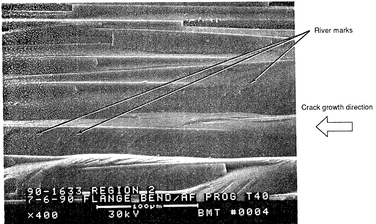
Figure 15. SEM Micrograph of a Mode I-Type (Tension) Fracture Surface in Region 2
