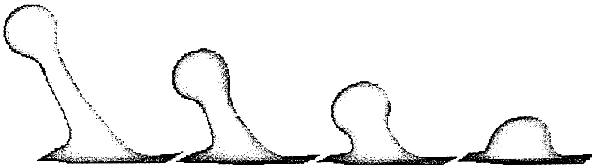
Figure 3. The results from a simulation of a vortex ring colliding with a fluid interface to form a "finger" of one fluid penetrating far into the other fluid. The shape of the fluid interface is shown at four times, with time increasing to the left.
