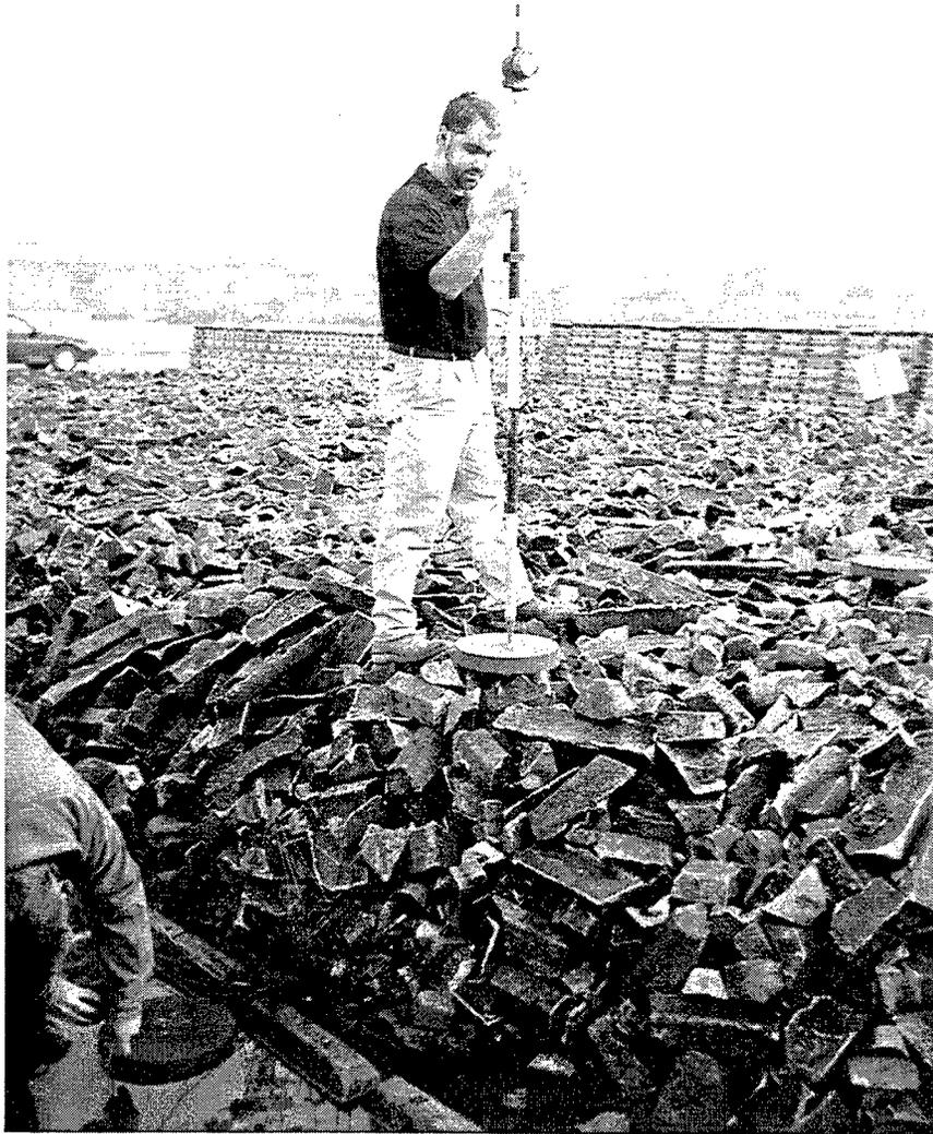
Figure 6. Elevation measurement at a microgravity station
