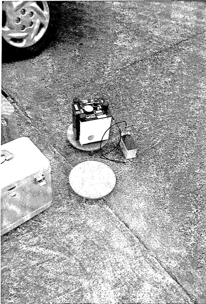
Figure 2. LaCoste and Romberg Model D gravity meter
