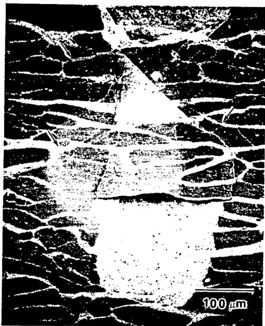
Fig. 8. Indentation fracture in an alumina/(alumina + zirconia) fibrous monolith. Viewed normal to the hot-pressing direction. Indentation (400-N load) diagonals oriented at  $45^\circ$  to the hot-pressing direction. Arrows indicate cracks from the indentation. The cell boundaries appear bright in the SEM micrograph.
