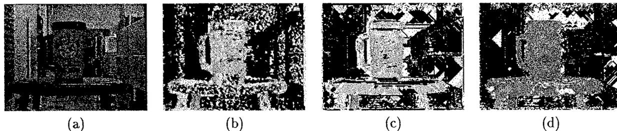
Figure 1: *Example of depth maps using fixed and adaptive block sizes: (a) intensity reference frame; (b) matching with fixed  $9 \times 9$  blocks; (c) matching with adaptive blocks; and (d) combining multiple local depth maps. The colors in (c) and (d) represent low confidence matches resulting from different artifacts as described in [1].*
