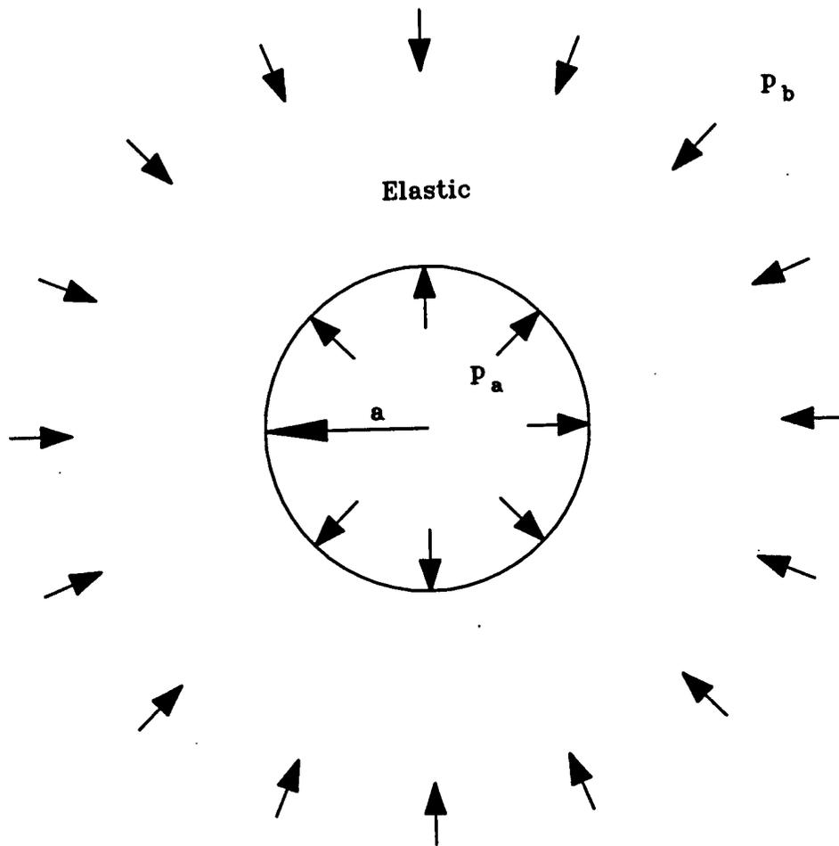
Figure 3-1. Phase 1 conditions for Cases Ia and Ib.
