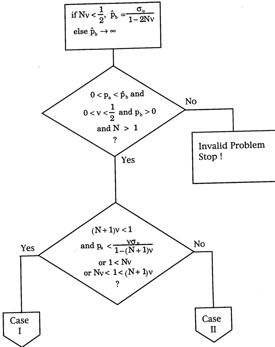
Figure 5-1. Flowchart for determining solution case.
