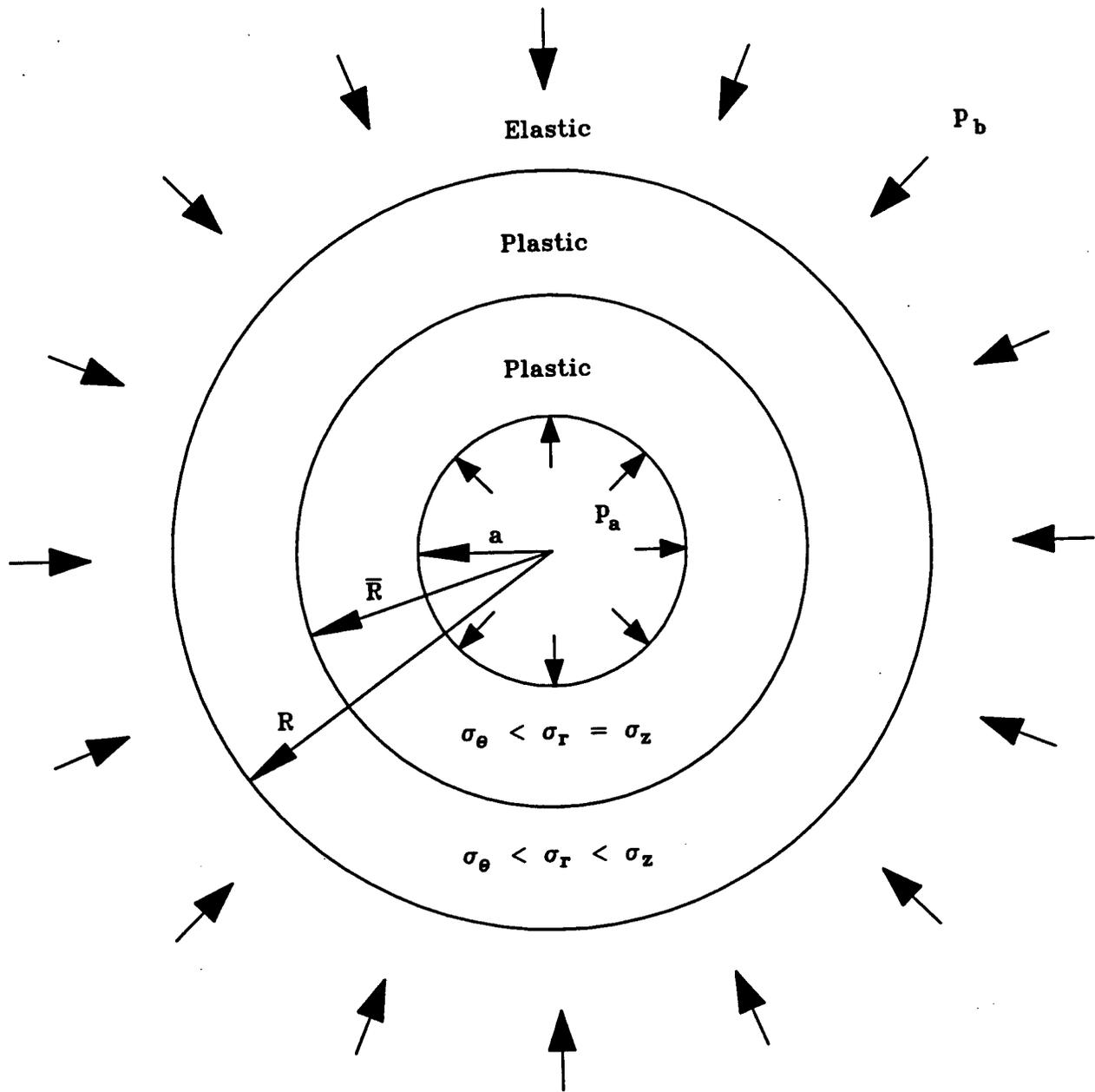
Figure 4-3. Phase 3 conditions for Case IIa.
