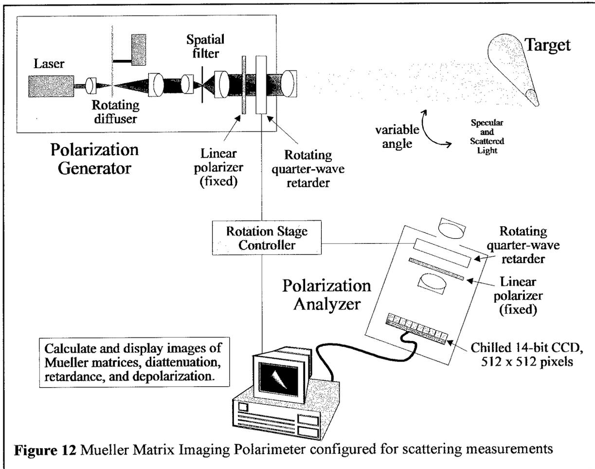
**Figure 12** Mueller Matrix Imaging Polarimeter configured for scattering measurements
