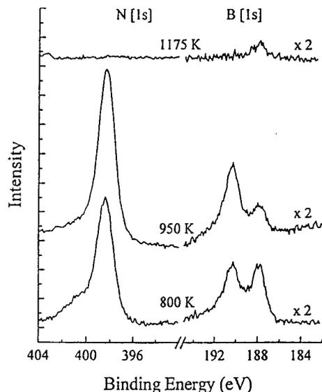
Fig. 4. N[1s] and B[1s] X-ray photoelectron spectra obtained after BN growth on Ni(100) at various substrate temperatures. Growth conditions were:  $1 \times 10^{-7}$  Torr  $\text{NH}_3$ ,  $1 \times 10^{-8}$  Torr  $\text{B}_2\text{H}_6$ , and the growth time was 30 min.
