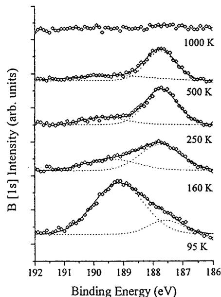
Fig. 2. X-ray photoelectron spectra for 15 L  $\text{B}_2\text{H}_6$  adsorbed onto Ni(100) at 95 K. B[1s] spectra were taken after heating the crystal to the indicated temperature for several s.
