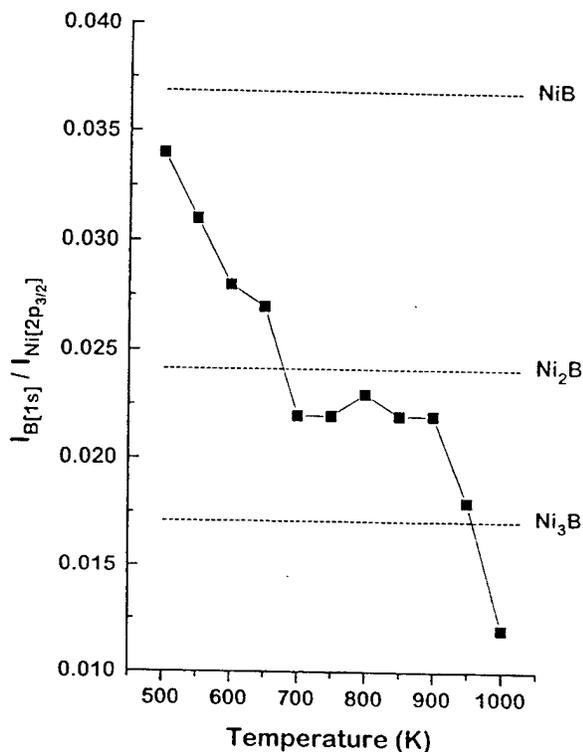
FIG. 6. Ratio of B [1s] peak height to Ni [2p<sub>3/2</sub>] XPS intensities as a function of annealing temperature. The initial surface was prepared by dosing 150 L  $B_2H_6$  onto the Ni(100) surface at 500 K.
