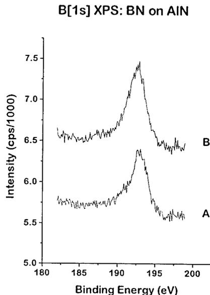
Fig. 3. a) XPS of the B[1s] level after exposure of the AlN surface to a mixture of  $10^{-8}$  Torr  $B_2H_6$  and  $10^{-7}$  Torr  $NH_3$  at 1050K for 10 min. b) Further exposure of the same surface to the same mixture for an additional 20 min. No further increase in the BN coverage is observed.
