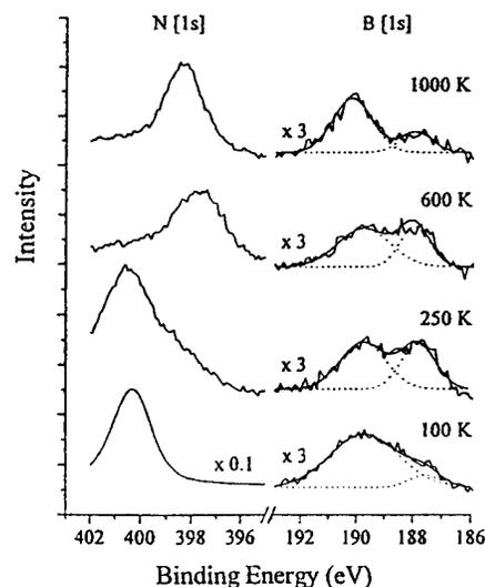
Fig. 3. N[1s] and B[1s] X-ray photoelectron spectra from the coadsorption of 5 L ND<sub>3</sub> followed by 15 L B<sub>2</sub>H<sub>6</sub> on Ni(100) at 100 K. Spectra were taken after heating the sample to 250, 600 and 1000 K.
