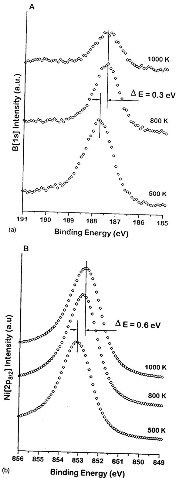
FIG. 7. (a) B [1s] and (b) Ni [2p<sub>3/2</sub>] XP spectra for a boron saturated surface prepared by dosing 150 L B<sub>2</sub>H<sub>6</sub> at 500 K. The spectra were taken after heating the sample to the indicated temperature.
