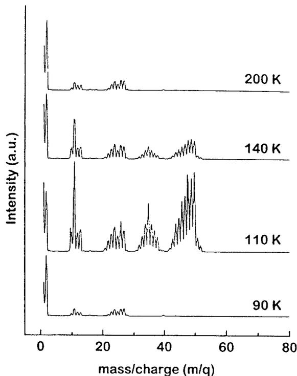
FIG. 3. Mass spectra for a 125 L exposure of  $B_2H_6$  adsorbed on Ni(100) at 85 K followed by heating at 1 K/s. While the sample was heated, the spectra were acquired at 90, 110, 140, and 200 K. Each spectrum required 7 s to acquire.
