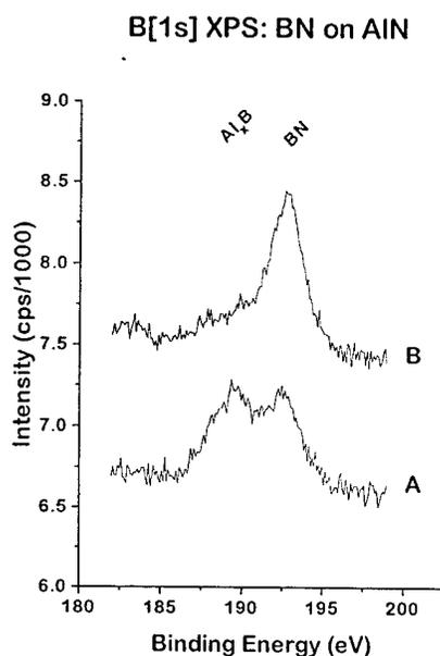
Fig. 2. a) XPS of the B[1s] level after exposure of the AlN surface to  $B_2H_6$  at  $10^{-8}$  Torr for 30 min. at 950K. The two species are assigned to an aluminum boride and BN. b) Exposure of this surface to  $NH_3$  results in the conversion of the aluminum boride to BN.
