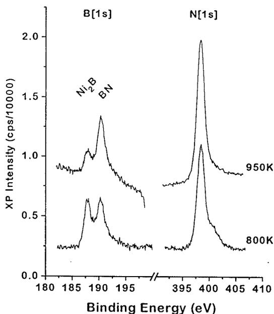
Figure 1. XP spectra observed after exposing the  $\text{Ni}(100)$  surface to  $\text{NH}_3$  and  $\text{B}_2\text{H}_6$  at various temperatures. BN has peaks clearly distinguishable from peaks associated with N and B bonded to nickel.
