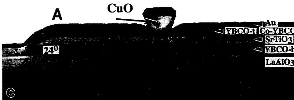
*Figure 5.* Cross-sectional TEM of an HTS edge junction, showing a CuO "boulder" growing in the top YBCO layer. The presence of such outgrowth in the bottom YBCO layer would typically cause a short through the insulator.
