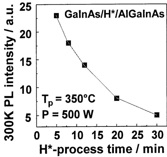
Fig. 1: 300K PL intensity of GaInAs regrown on H\*-treated  $\text{Al}_{0.16}\text{Ga}_{0.32}\text{In}_{0.52}\text{As}$  as a function of H\*-exposure time.
