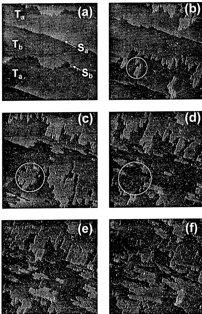
Fig.: STM images ( $2900 \times 2900 \text{ \AA}$ ) of the growth of Si on Si(100) at 725K. Images a-f were recorded at 0.22, 0.53, 0.94 and 1.14 layers Si coverage respectively. In (b-d) an island is indicated where the  $(2 \times 1)$  reconstruction is out of phase with the upper terrace. This induces nucleation of islands upon coalescence of this island with the upper terrace.
