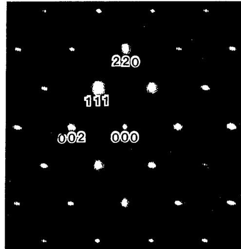
Fig. 2. TED pattern from the  $(1\bar{1}0)$  cross-section of the IPSSL grown on a substrate tilted at  $1.5^\circ$ .
