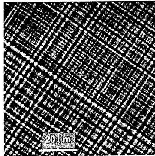
Fig. 2. AFM micrograph of the surface of a  $\text{In}_{0.5}\text{Ga}_{0.5}\text{As}/\text{GaAs}$  MQW (with mean composition  $x=0.34$ ) grown on top of a linearly graded  $\text{In}_x\text{Ga}_{1-x}\text{As}$  buffer ( $0 < x < 0.41$ ). The buffer and the MQW were grown by MBE and ALMBE, respectively, at  $400^\circ\text{C}$  with a  $\text{As}_2$  beam. The surface roughness (along the (110) directions) has a rms value of 4 nm and a period of  $\sim 2 \mu\text{m}$ .
