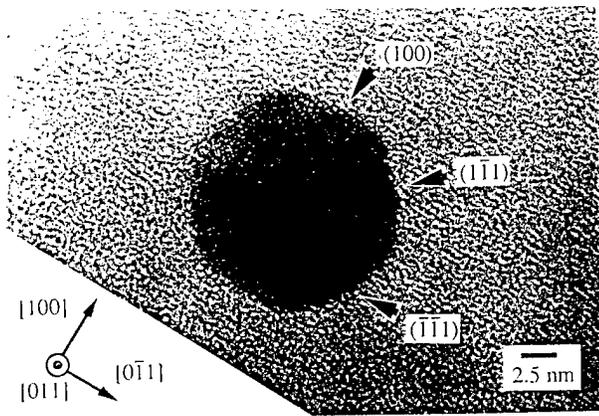
FIG. 3. Higher magnification of a Si nanoparticle of  $d \approx 14$  nm. Note the (100) and (111) facets appear as opposed to thermodynamically allowed crystal structure having only (111) and (311) facets.
