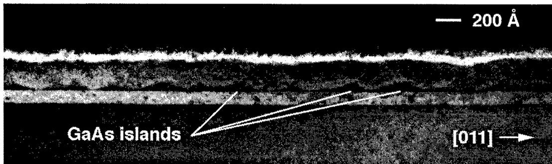
Transmission electron micrograph of GaAs quantum well island layer (dark) in  $\text{Al}_{0.5}\text{Ga}_{0.5}\text{As}$ . The islands are trapezoidal in cross-section and have a width of 200-400 Å at the base.
