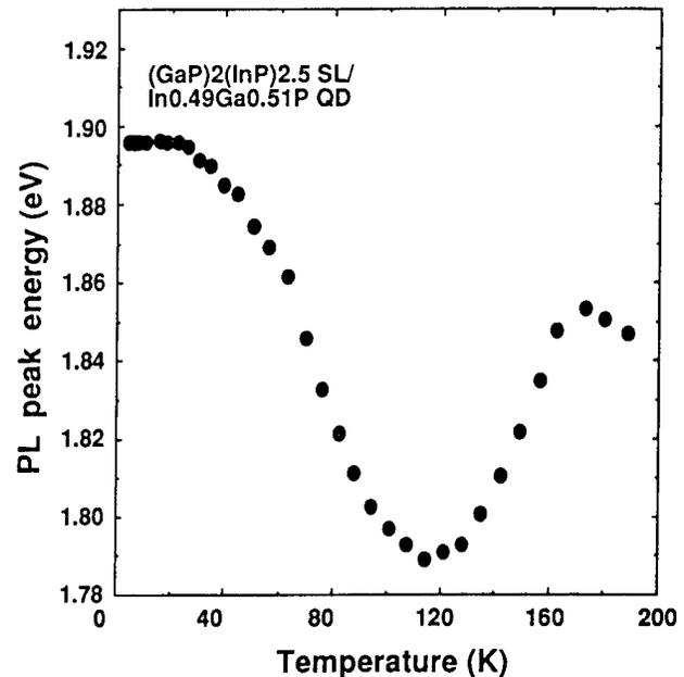
Fig. 4 Temperature dependence of PL peak energy for the  $(\text{GaP})_2(\text{InP})_{2.5}$  SL/ $\text{In}_{0.49}\text{Ga}_{0.51}\text{P}$  quantum dot structure grown on GaAs (311)A. Temperature dependence of PL peak energy shows an anomalous behavior in the range 125-170 K.
