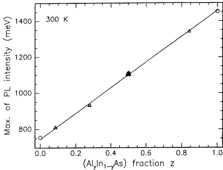
Fig. 1: Maximum of the PL intensity at room temperature plotted vs. the (Al<sub>0.48</sub>In<sub>0.52</sub>As) fraction  $z = r_2/(r_1+r_2)$  in the quaternary layer.
