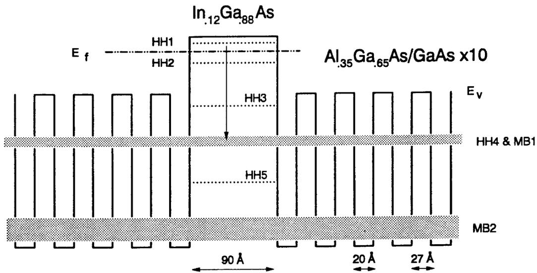
Figure 1. Schematic Energy Band Diagram and Intersubband Transition.
