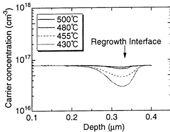
Fig. 4 C-V profile near n-GaAs/n-GaAs regrowth interface.
