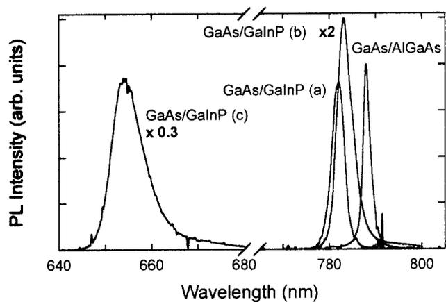
**Fig.1:** 10K photoluminescence data from GaAs/GaInP and GaAs/AlGaAs MQW structures. For the GaInP-based structures; (a)= optimised interface, (b)= as (a), but with AlInP cap, (c)= (non-intentional) GaAsP/GaInP graded MQW.
