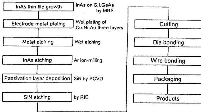
Fig.1, Fabrication process of the InAs Hall element
