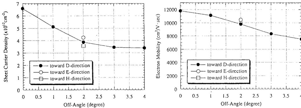
Fig.4 Properties of InAs thin films grown on GaAs substrates with various tilted angles and tilted directions of misorientation by MBE
