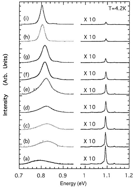
Figure 1 - PL spectra of Sample A as a function of annealing temperature and time -  $\text{Si}_{1.7}\text{Ge}_{0.3}$  alloy layer on a p-Si substrate; (a) As grown (b)  $800^\circ\text{C}$  - 30 min. (c)  $800^\circ\text{C}$  - 60 min. (d)  $900^\circ\text{C}$  - 30 min. (e)  $900^\circ\text{C}$  - 60 min. (f)  $1000^\circ\text{C}$  - 30 min. (g)  $1000^\circ\text{C}$  - 60 min. (h)  $1100^\circ\text{C}$  - 30 min. (i)  $1100^\circ\text{C}$  - 60 min.
