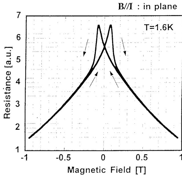
Figure 2: Magneto-resistance curve of a 1000 nm-thick  $(\text{Ga}_{1-x}\text{Mn}_x)\text{As}$  ( $x=0.05$ ) film measured at 1.6K. The magnetic field was applied in-plane, along the [110] axis of GaAs (and GaMnAs). The current was also along the [110]. The clear hysteresis behavior indicates ferromagnetic ordering.
