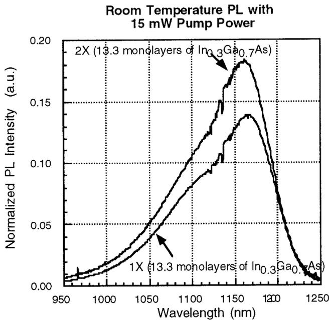
Figure 3: Two layers of quantum dots have an increased RTPL intensity compared to a single layer. These dots are formed by depositing 13.3 monolayers of  $\text{In}_{0.3}\text{Ga}_{0.7}\text{As}$ . The single dot layer sample also shows stronger band-filling as indicated by the more pronounced high energy shoulder.
