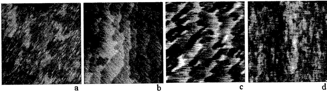
Fig.1. Atomic force microscopy images ( $2\ \mu\text{m} \times 2\ \mu\text{m}$ ) of the cap layer surfaces of the quantum well layer system prepared at different growth conditions.  $T_s$  and BEP ratios of arsenic-to-gallium were  $640^\circ\text{C}/10$  (a),  $610^\circ\text{C}/10$  (b),  $610^\circ\text{C}/30$  (c) and  $550^\circ\text{C}/10$  (d). Substrates were unintentionally misoriented by about  $0.03^\circ$ - $0.05^\circ$  towards (011).
