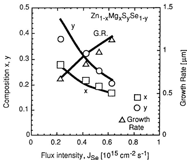
Figure 4 Se flux intensity dependence of the mole fraction and the growth rate of experimental values (symbol) and calculated ones (curve) of ZnMgSSe.  $J_{Zn}$ ,  $J_{Mg}$ ,  $J_S$  are 0.88, 0.12, 0.19 [ $10^{15} \text{ cm}^{-2} \text{ s}^{-1}$ ], respectively.
