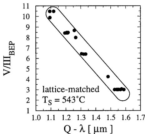
Fig. 2: High quality GaInAsP layers we obtained at  $T_S = 543 \text{ }^\circ\text{C}$  when the  $V/III_{\text{BEP}}$  ratio is controlled closely in a narrow window. With increasing Ga and As contents the  $V/III_{\text{BEP}}$  - ratio has to be lowered.
