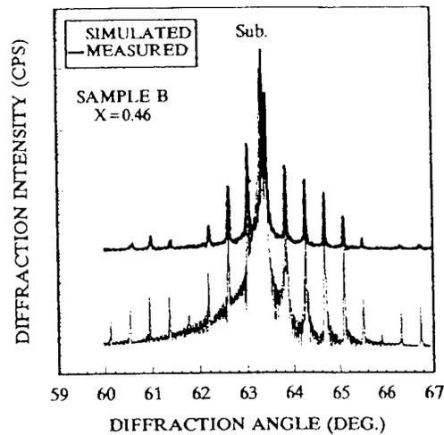
FIG.2 Double crystal rocking curve for sample B.
