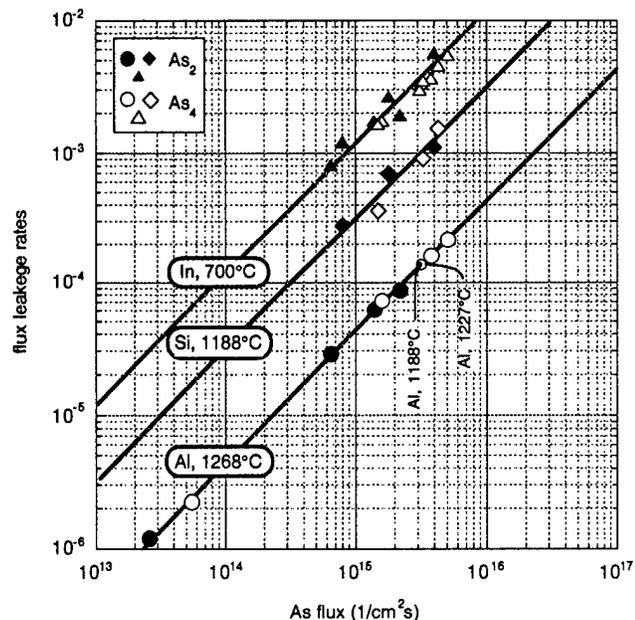
Flux leakage rate is defined here as the ratio of the flux incident on the wafer with the cell shutter closed to the nominal flux with the cell shutter open. It has intuitive meaning of the "effective transparency of the shutter."
