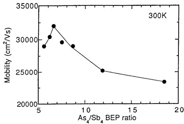
Fig. 2. Room temperature mobility for InAs DQWs as a function of As<sub>4</sub>/Sb<sub>4</sub> BEP ratio.
