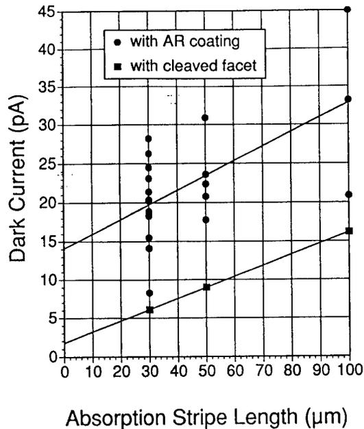
Fig.3 Dark current of the waveguide photodiodes at the reverse bias voltage of -3V.
