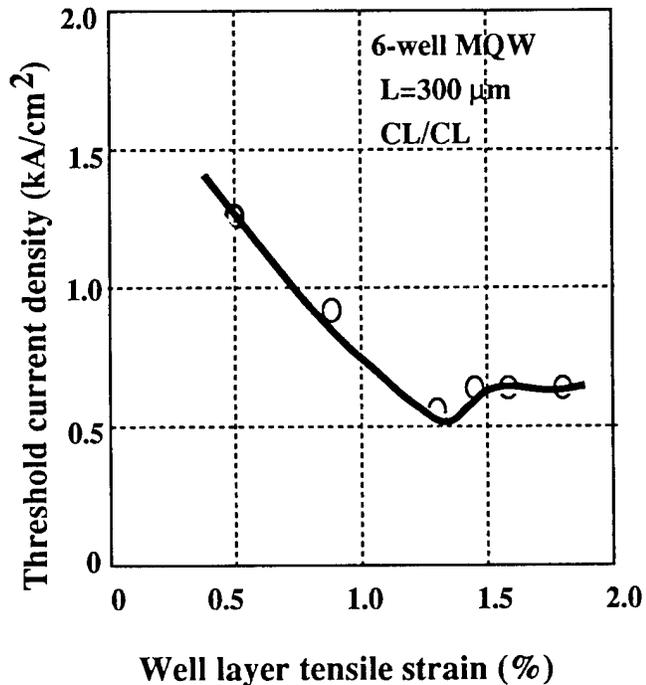
Fig. 4 Relation between the threshold current density  $J_{th}$  and well layer tensile strain.  $J_{th}$  decreases with increase in strain, to a minimum  $J_{th}$  of 0.6 kA/cm<sup>2</sup> at 1.3% strain.
