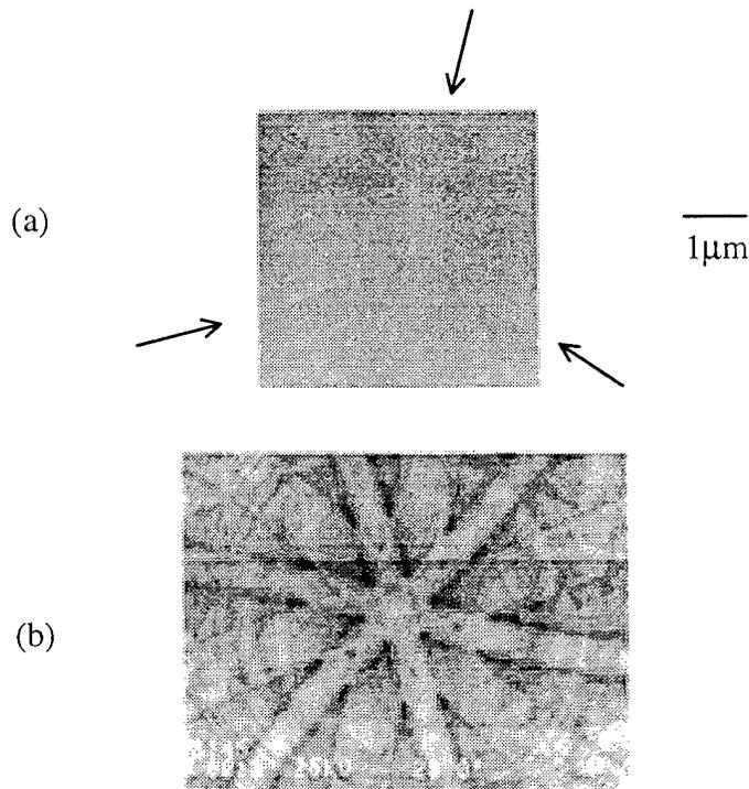
(a) SEM micrograph of a 13µm InSb/BaF<sub>2</sub>/CaF<sub>2</sub>/Si(111) film revealing shallow triangular steps believed to be related to {100}<110>-type glide steps and (b) Corresponding ECP pattern showing the presence of (111)-related 6-fold symmetry.
