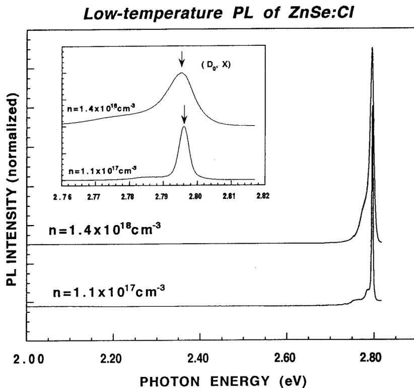
Fig.2 Low-temperature PL of ZnSe: Cl with different carrier concentrations of  $1.4 \times 10^{18} \text{ cm}^{-3}$  (upper spectrum) and  $1.1 \times 10^{17} \text{ cm}^{-3}$  (lower spectrum). The samples were excited by a He-Cd laser at about 2K.
