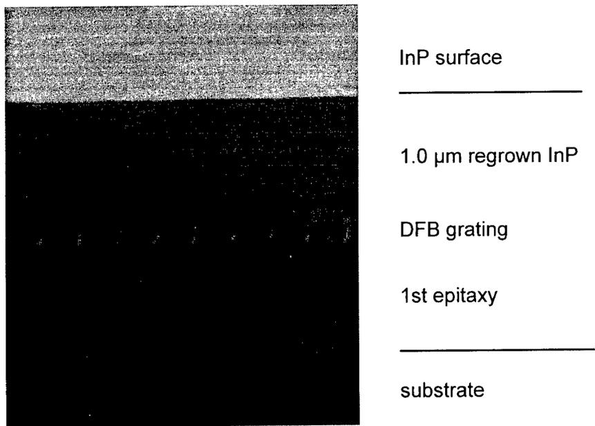
Fig. 2: REM of a tilted stained cross-section of a 1.5  $\mu\text{m}$  thick InP layer regrown on a 195 nm deep DFB grating defined by RIE.
