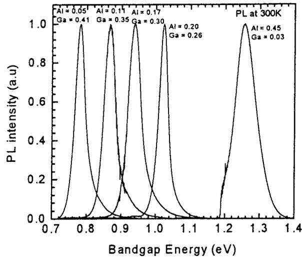
Fig.1 PL spectra of bandgap engineered InGaAlAs epilayers
