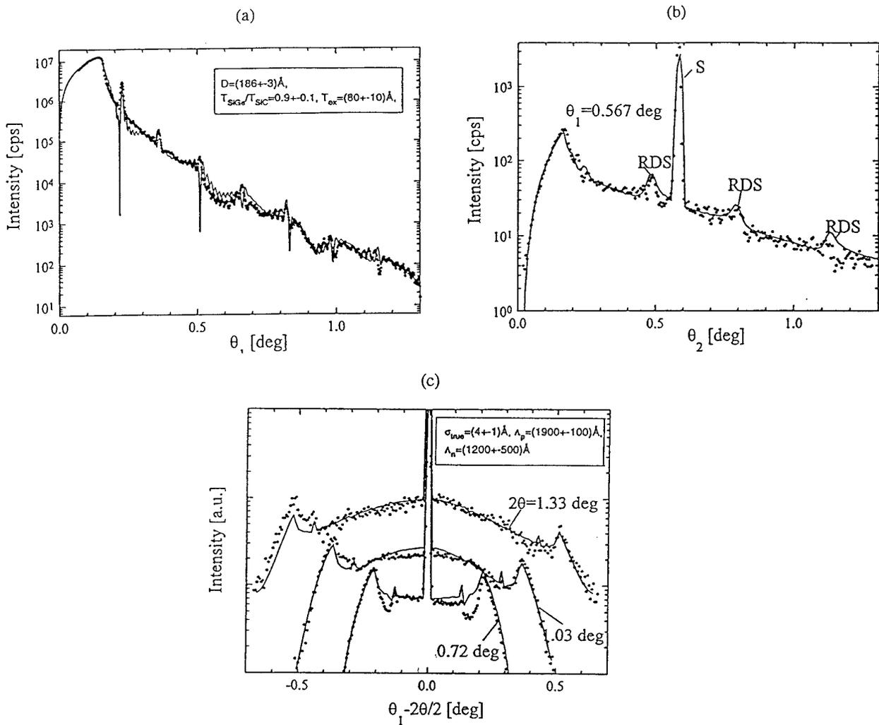
Figure 1: (a) Measured and simulated specular reflectivity ( $\omega$ - $2\theta$ -scan)
