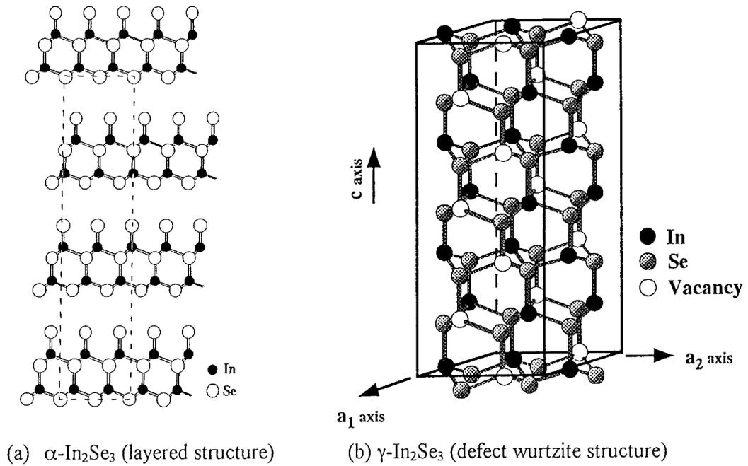
Fig.1 Crystal structure of  $\alpha$ - and  $\gamma$ - $\text{In}_2\text{Se}_3$ .
