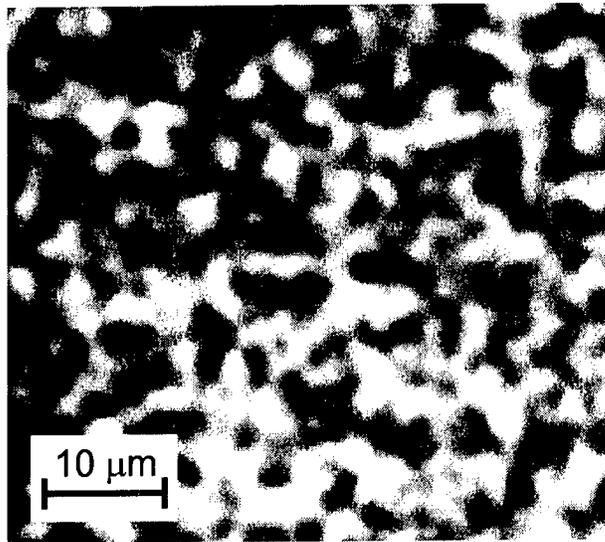
Figure 1) The room-temperature cathodoluminescence of a 1  $\mu\text{m}$  ZnSe film grown by MBE on a  $c(4\times 4)$  GaAs buffer layer at a magnification of 1700. The defect density is  $>10^6 \text{ cm}^{-2}$ . The electron probe parameters were: 30nA, 20kV.
