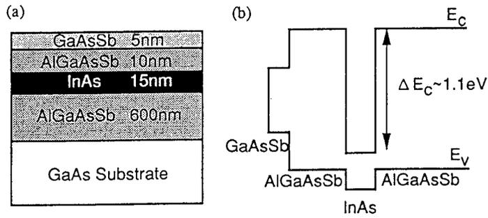
Fig. 1. (a) Schematic cross section and (b) energy band diagram of InAs/Al<sub>0.5</sub>Ga<sub>0.5</sub>AsSb DQWs.
