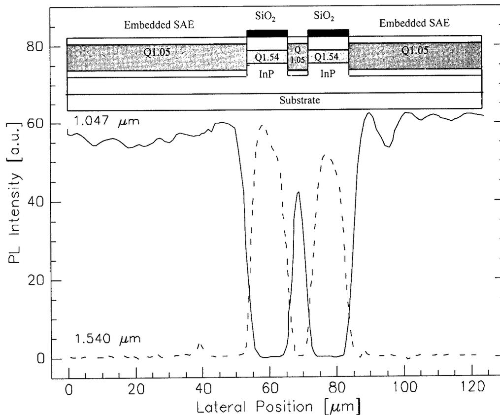
Fig. 2: PL spatial linescans across a structure as in Fig. 1, but SAE infill using GaInAsP with  $\lambda_g = 1.047 \mu\text{m}$  (see insert; lateral heterojunction achieved by embedded SAE; the quaternary layers are indicated by Q1.05 ( $\lambda_g = 1.047 \mu\text{m}$ ) and Q1.54; all other layers are InP).
