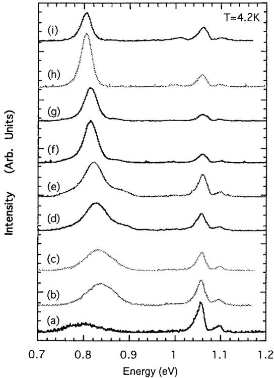
Figure 2 - PL spectra of Sample B as a function of annealing temperature and time -  $\text{Si}_{1.7}\text{Ge}_{0.3}$  alloy layer on unimplanted BESOI substrate; (a) As grown (b)  $800^\circ\text{C}$  - 30 min. (c)  $800^\circ\text{C}$  - 60 min. (d)  $900^\circ\text{C}$  - 30 min. (e)  $900^\circ\text{C}$  - 60 min. (f)  $1000^\circ\text{C}$  - 30 min. (g)  $1000^\circ\text{C}$  - 60 min. (h)  $1100^\circ\text{C}$  - 30 min. (i)  $1100^\circ\text{C}$  - 60 min.
