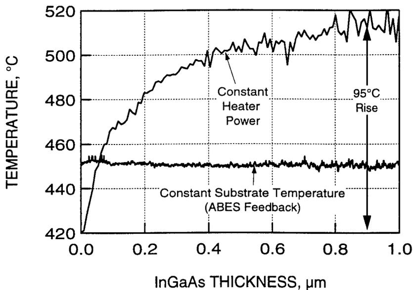
Figure 2. ABES data show that the true substrate temperature rises by 95-100°C during the growth of  $\text{In}_{.53}\text{Ga}_{.47}\text{As}$  on InP, at constant heater power (or constant thermocouple temperature). By using ABES sensor feedback, the spurious temperature increase due to InGaAs growth can be completely eliminated. Constant substrate temperature is advantageous in the growth of HBTs and other devices based on lattice-matched InGaAs on InP.
