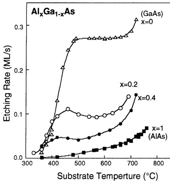
**Fig. 1** The variation with temperatures in the etching rates of  $\text{Al}_x\text{Ga}_{1-x}\text{As}(100)$  at an  $\text{AsBr}_3$  flow rate of 0.080 sccm and a concomitant  $\text{As}_4$  flux of 1.5 ML/s. The etching rate is determined from the period of the RHED oscillations.
