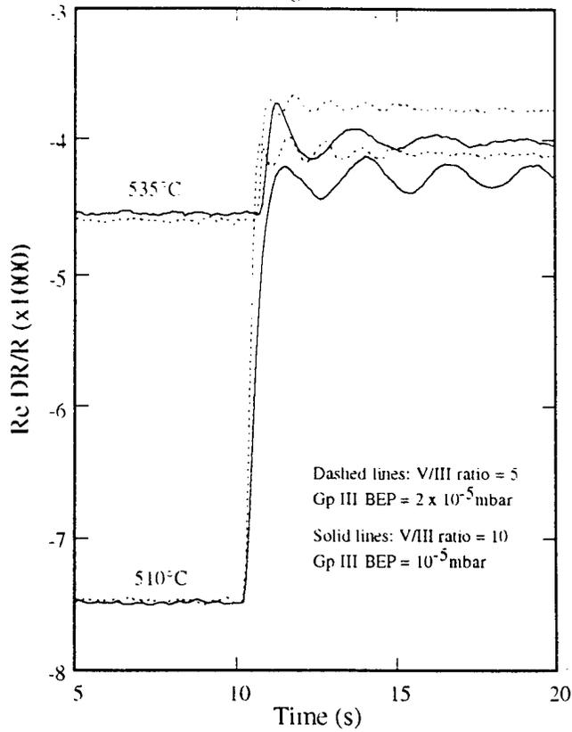
Figure 2 Dependence of the surface transient state on precursor pressure
