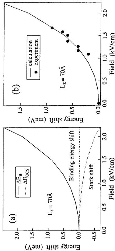
FIG.2. Field dependence of FE binding energy and QCS shifts. Left: calculation. Right: Experiment (line is the fit).
