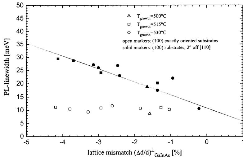
Fig.2 Photoluminescence linewidth of the GaInAs quantum well peak as a function of the lattice mismatch  $(\Delta d/d)_{\perp}$  of the GaInAs layers for off-oriented and exactly oriented (100) InP substrates.
