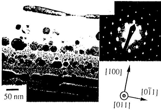
FIG. 1. Stratified SiO<sub>2</sub> suspension of highly oriented Si nanoparticles. Dark contrast corresponds to Si. Left: Cross section TEM. Right: Selective diffraction of a nanoparticle. Note the ordered crystalline arrangement of nanoparticles.
