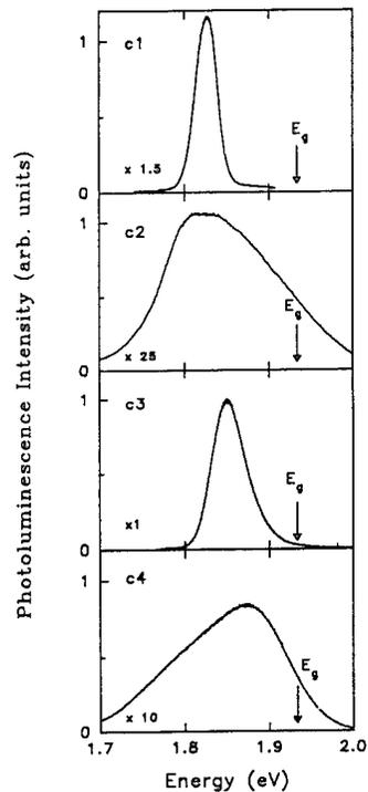
Fig. 4 - Photoluminescence spectra of the (111)A samples listed in Table I measured at 12 K. The PL was excited by the 488 nm laser line with a power density of  $20 \text{ W/cm}^2$ . The relative sensitivity factor is given on the left. The hollow arrows indicate the energy gap ( $E_g$ ) values (see text).
