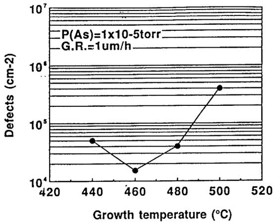
Fig.2 Defect density of 3µm AlGaInAs as a function of growth temperature.
