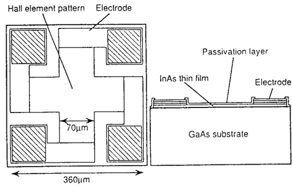
Fig.2 Structure of the InAs Hall element chip
