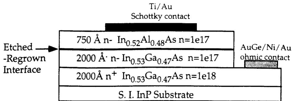
Fig. 1: Schematic of Regrown N-n Heterojunction Capacitor
