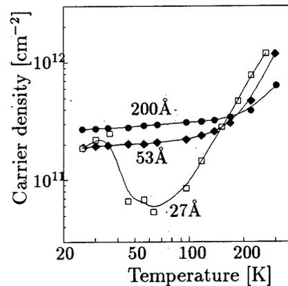
**Figure 4:** Temperature dependence of the samples. For simplicity characteristics of 200Å, 53Å and 27Å samples are shown. Characteristics of 100Å, 40Å and 13Å samples are similar to 200Å, 53Å and 27Å samples, respectively.
