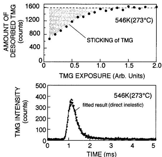
**Fig.1** (a) The amount and (b) the time-of-flight spectrum of TMG scattered from less stabilized GaAs(100)-(1x6) surface. The shaded area in (a) corresponds to the sticking of TMG. The time-of-flight spectrum in (b) is well reproduced by the single component for the scattering without surface residence. This result suggests that TMG molecules are mainly adsorbed with dissociation, although TMG molecules may be trapped in the precursor state.
