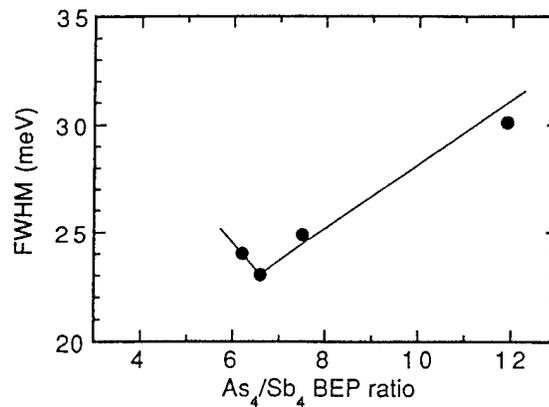
Fig. 4. The FWHM of the PL peak for AlGaAsSb as a function of As<sub>4</sub>/Sb<sub>4</sub> BEP ratio.
