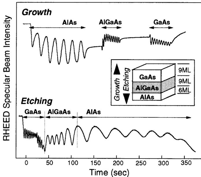
**Fig. 2** The RHEED specular-beam intensity evolution during the growth (upper) and etching (lower) of GaAs(9ML)/ $\text{Al}_{0.2}\text{Ga}_{0.8}\text{As}(9\text{ML})/\text{AlAs}(6\text{ML})$  on GaAs(100) substrate at substrate temperature of 600°C, an  $\text{AsBr}_3$  flow rate of 0.080 sccm and a concomitant  $\text{As}_4$  flux of 1.5 ML/s
