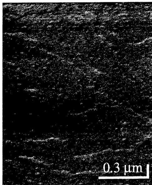
Fig. 2. GaAs (001) surface just after MEE growth (10 ML).
