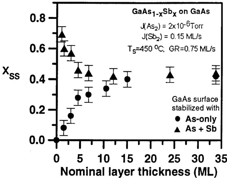
Figure 2. Evolution of Sb surface accumulation ( $x_{ss}$ ) near the normal interface. Prior to  $\text{GaAs}_{0.8}\text{Sb}_{0.2}$  deposition, the GaAs surface is stabilized with  $\text{As}_2$  only (circle), or with both  $\text{As}_2$  and  $\text{Sb}_2$  (diamond).
