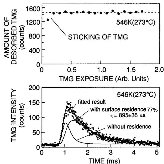
**Fig.2** (a) The amount and (b) the time-of-flight spectrum of TMG scattered from highly stabilized GaAs(100)-(2x4) surface. The shaded area in (a) corresponds to the sticking of TMG. The time-of-flight spectrum in (b) is well reproduced by the sum of two components for scattering with and without surface residence. This result suggests that most of TMG molecules are desorbed without dissociation after a long surface residence in the precursor state.
