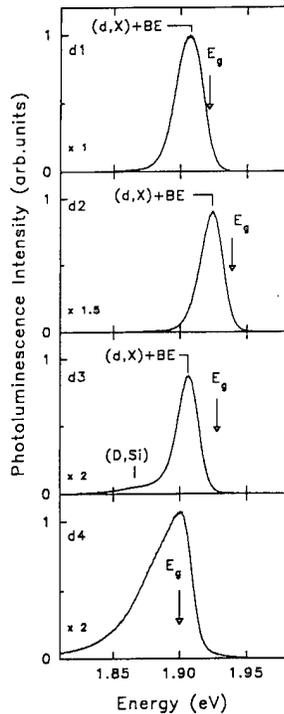
Fig. 3 - Photoluminescence spectra of the (211)A samples listed in Table I measured at 12 K. The PL was excited by the 488 nm laser line with a power density of  $20 \text{ W/cm}^2$ . The relative sensitivity factor is given on the left. The hollow arrows indicate the energy gap ( $E_g$ ) values. The labels on the spectra have the following meaning: BE, bound exciton; (d,X) defect bound exciton; (D,Si), donor to silicon acceptor pair transition
