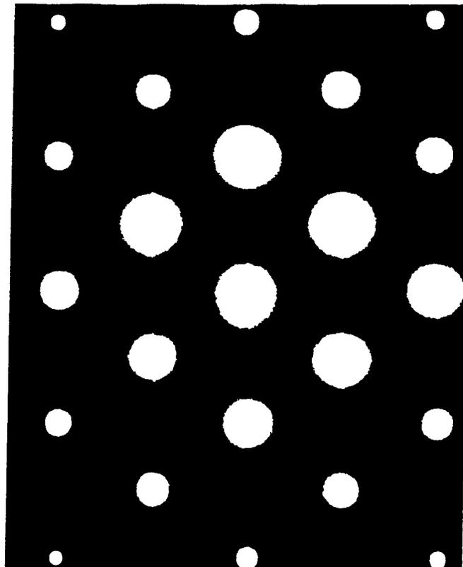
Fig. 2 TED pattern of the  $\text{InAs}/\text{InAs}_{0.76}\text{Sb}_{0.24}$  SL active region in a midwave infrared laser structure.
