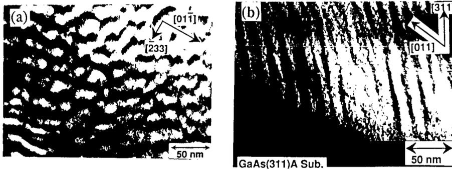
Fig. 1 TEM images for the  $(\text{GaP})_2(\text{InP})_2$  SLs grown on GaAs (311)A. (a) bright-field plan-view TEM image and (b)  $g=002$  dark-field cross-sectional TEM image for (01-1). The columnar structure ordering is oriented along the  $[211]$  direction.
