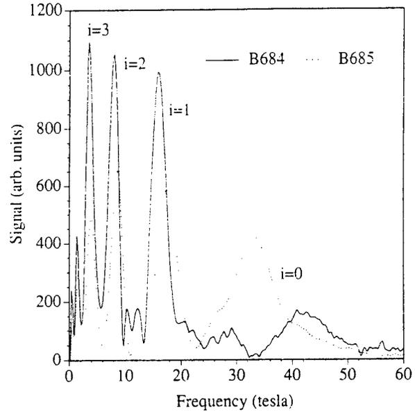
Fig. 3: The amplitude spectra for B684 and B685,  $\delta$ -doped samples with areal Si densities of  $3 \times 10^{12} \text{ cm}^{-2}$ . The tighter confinement of dopant atoms in B684 is again reflected through the higher frequency of the  $i=0$  peak compared with that of B685, and a shift to low frequency for the  $i \geq 1$  peaks. The spreading in B685 is  $\approx 40$  ML.
