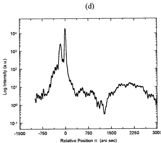
Double axis X-ray scans of InGaAs epilayers in tensile (c) and compressive strain (d). The epilayers have similar mismatch, however, the compressively strained layer exhibits greater decay in the pendollosung X-ray fringes, due to misfit dislocations and mosaic tilts in the epilayer.
