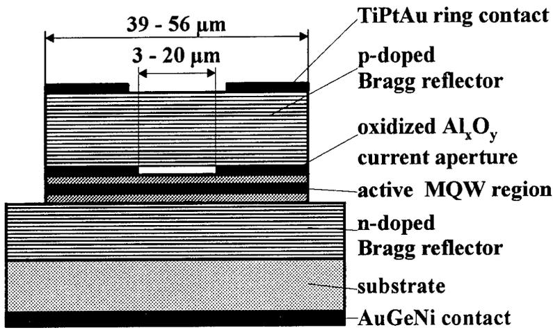
Fig. 1: Schematic of top emitting VCSEL
