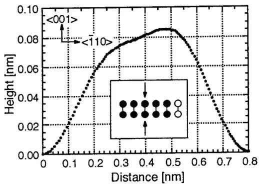
Fig.1 Cross-section of S dimer in (2x6)-S.
