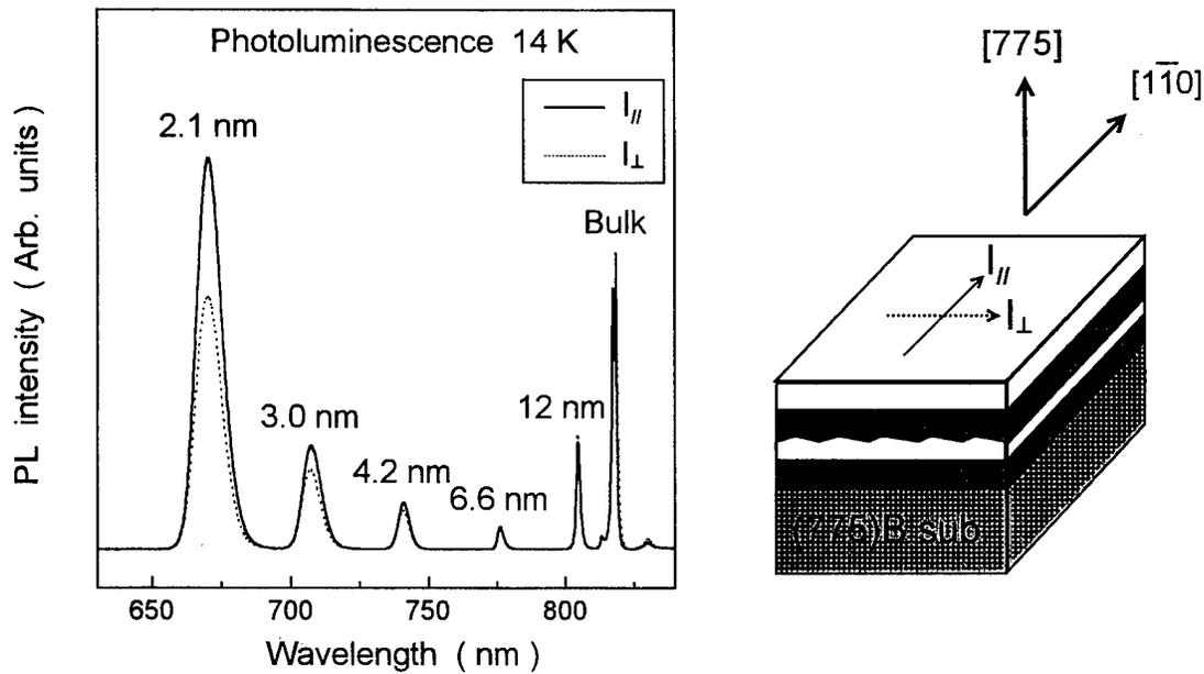
Fig. 3 : Polarized PL spectra from GaAs/ $(\text{GaAs})_2(\text{AlAs})_2$  QWRs grown on (775)B GaAs substrate.
