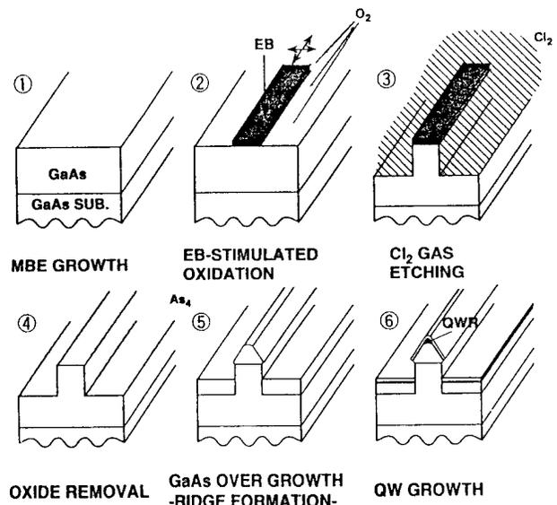
**Fig. 2** Process sequence of *in situ* patterning and regrowth used to define the first array of quantum wires. This first array of wire structures was buried in a 500nm thick GaAs layer. Then, the second array of wire structures was successively formed by a second pattern and regrowth process using steps (2) to (6).
