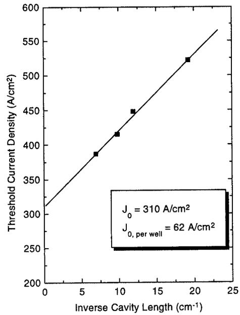
Fig. 2 Threshold current density plotted against inverse cavity length.
