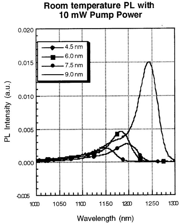
Figure 2: 9 nm of GaAs grown at 515°C gives the best room temperature PL results. Thicker layers of GaAs lead to reduced PL intensity. Quantum dots are 17.7 monolayers of  $\text{In}_{0.3}\text{Ga}_{0.7}\text{As}$
