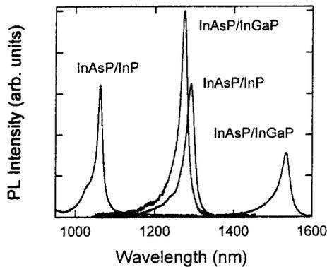
Fig.3: Room temperature photoluminescence data for  $\text{InAsP}/\text{In}(\text{Ga})\text{P}$  MQW structures with  $\lambda \sim 1.06, 1.3$  &  $1.55 \mu\text{m}$ . The PL linewidths are in the range 15-20meV.
