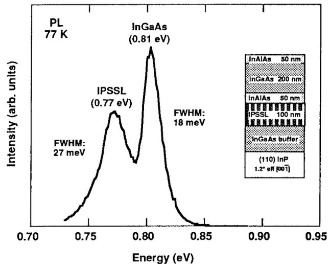
Fig. 4. PL spectrum of the IPSSL sample grown with the  $\text{In}_{0.53}\text{Ga}_{0.47}\text{As}$  alloy on a substrate tilted at  $1.2^\circ$ .
