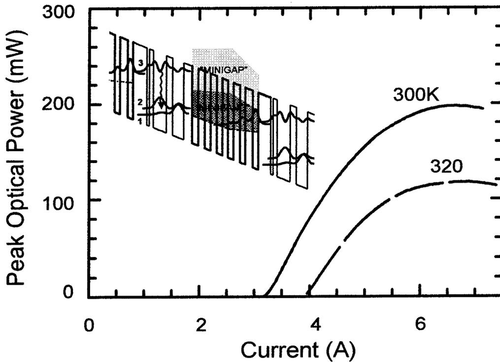
Fig. 1 Pulsed optical output power from a single facet versus injection current for heat sink temperatures of  $T = 300$  K and  $T = 320$  K. The device is 2.9 mm long and 14  $\mu\text{m}$  wide. Inset: Schematic conduction band diagram of a portion of the active region.
