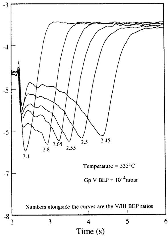
Figure 3 RAS trace of the transient surface state for different precursor pressures and temperatures
