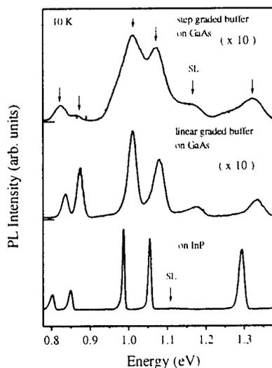
**Fig. 4.** PL spectra of the samples studied with five quantum wells lattice matched on InP and with lattice relaxed linear and step graded buffer on GaAs. From left to right the arrows indicate the well widths 20, 10, 4, 3, and 1nm, respectively. The luminescence of the superlattice grown before the quantum well layer sequence is denoted by SL.
