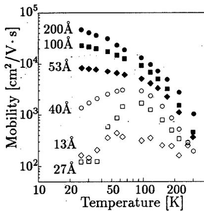
**Figure 3:** Temperature dependence of the samples grown by the present technique with varied channel width  $W$ . In  $W=200\text{Å}$  sample mobility up to  $\sim 50000\text{cm}^2/\text{Vs}$  is achieved at 25K.
