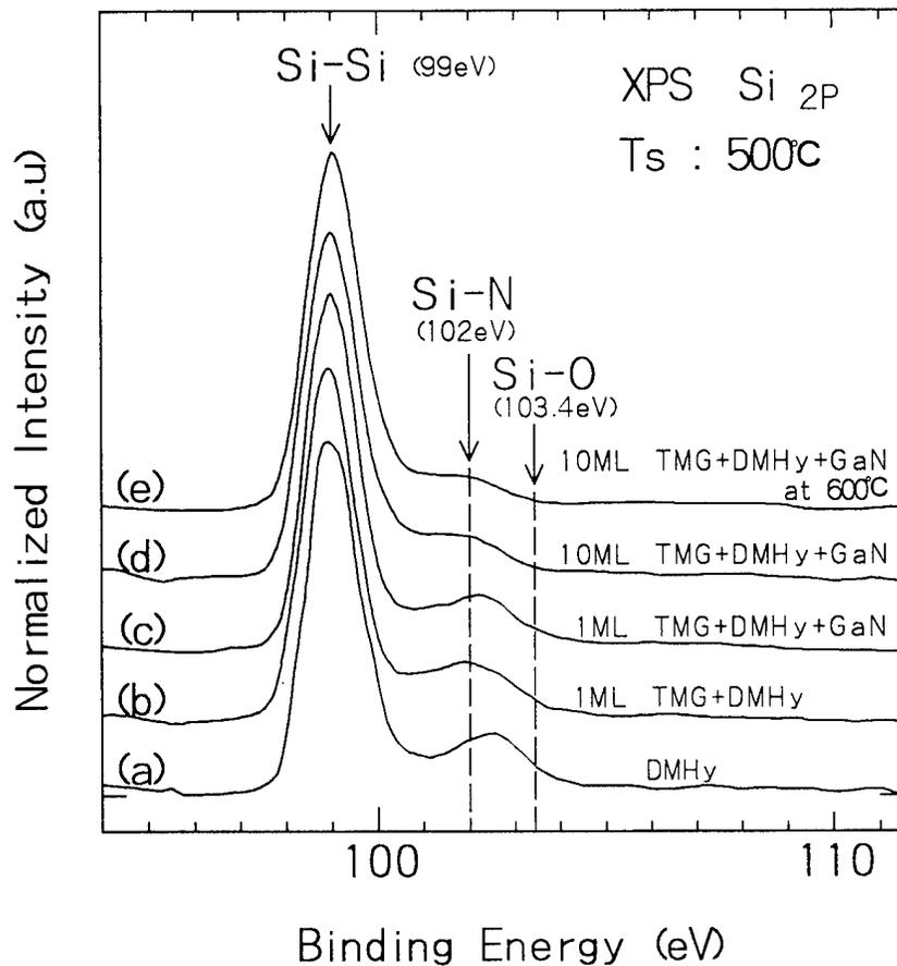
Fig. 1. Si<sub>2p</sub> XPS spectra corresponded to the various initial growth conditions.
