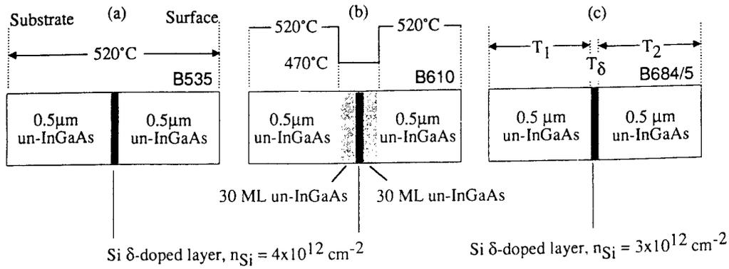
Fig. 1: (a) B535,  $\delta$ -doped structure grown entirely at 520 °C: (b) B610, 0.5  $\mu\text{m}$  undoped InGaAs grown at 520 °C, 30 ML -  $\delta$ -doping - 30 ML deposited at 470 °C, 0.5  $\mu\text{m}$  undoped InGaAs grown at 520 °C: (c) B684,  $T_1$  and  $T_\delta$  both set to 520 °C,  $T_2 = 470$  °C; B685,  $T_1$  and  $T_\delta$  both set to 470 °C,  $T_2 = 520$  °C.
