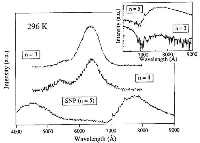
FIG. 4. Room temperature photoluminescence spectra of Si nanoparticles (bottom). The upper traces are luminescence of Si slab embedded in SiO<sub>2</sub>.
