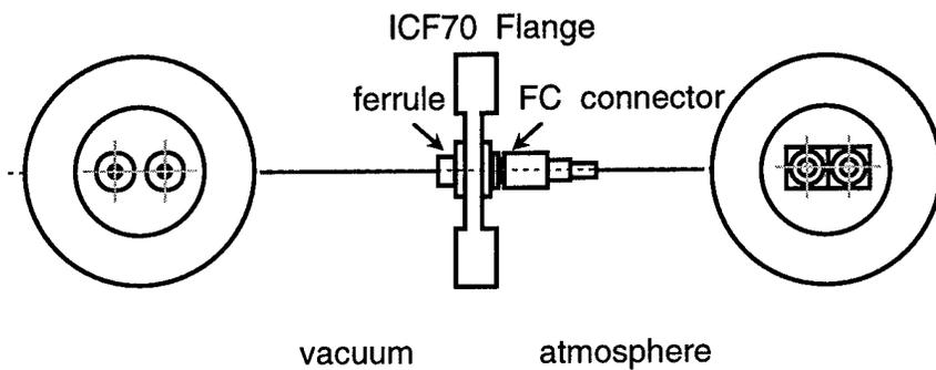
Fig.2 : UHV flange with optical fiber feedthrough.
