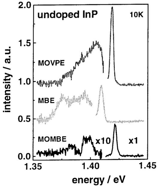
Fig. 2: Comparison of typical 10K PL spectra of MOMBE, MOVPE and MBE InP layers. The energetic shift of the dominant excitonic emission of the MBE InP grown at  $420^\circ\text{C}$  from a GaP source is indicative of As-incorporation while the slightly enhanced FWHM is related to a  $10^{15}\text{ cm}^{-3}$  residual carrier background.
