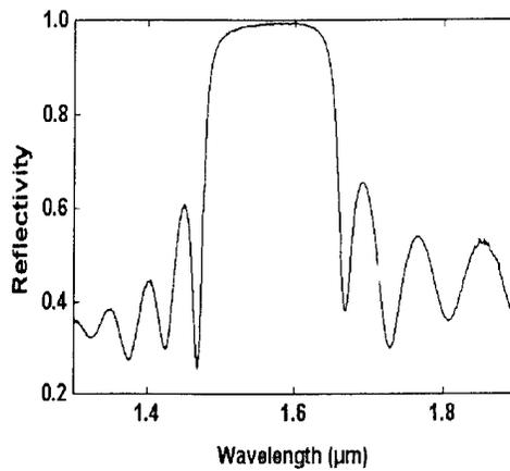
Fig. 4. Spectral reflectivity of a 20 periods  $Al_{0.1}Ga_{0.9}As_vSb_{(1-v)}$  /  $AlAs_xSb_{(1-x)}$  distributed Bragg mirror. The reflectivity is 0.995 at  $1.58\mu m$
