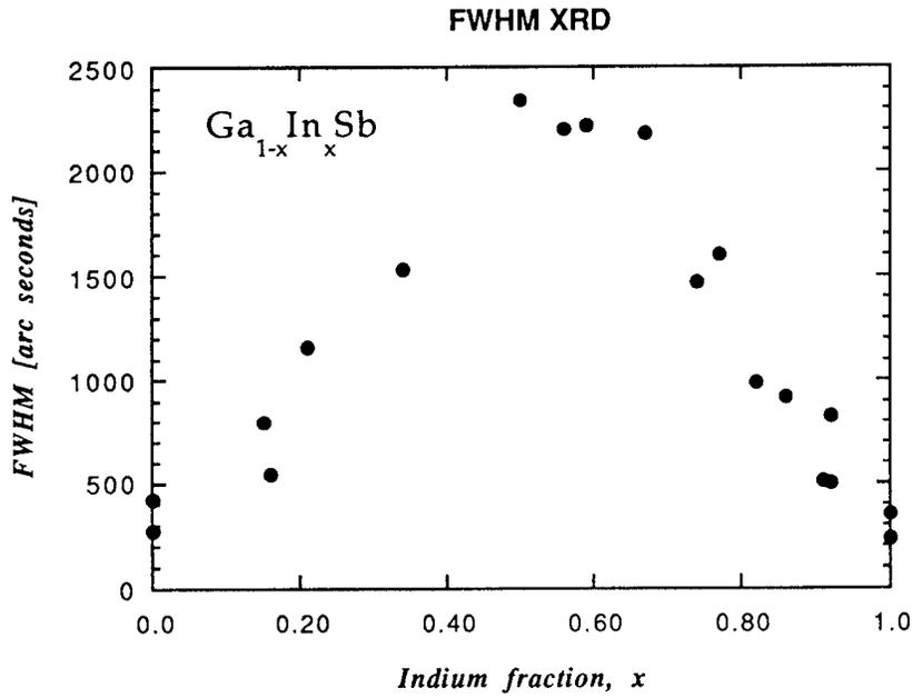
**Figure 1.** Full width at half maximum of the  $\text{Ga}_{1-x}\text{In}_x\text{Sb}$  peak in X-ray diffraction as a function of the In molar fraction  $x$ . The figure indicates that the broadening is related to disorder in the alloy.
