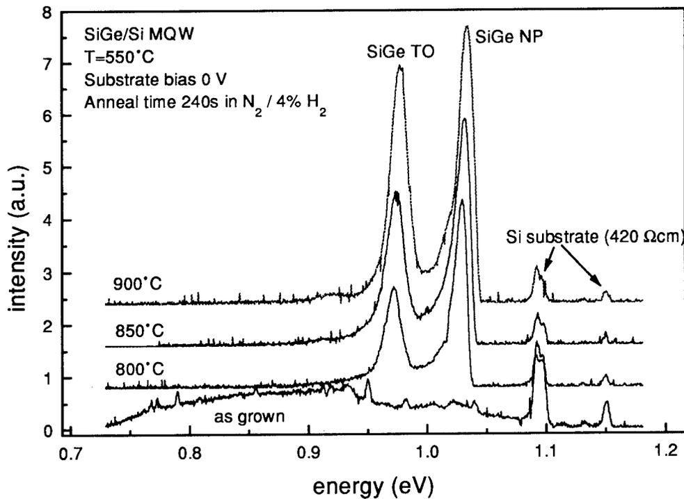
Fig.2: Photoluminescence (4K) spectra of a Si<sub>0.83</sub>Ge<sub>0.17</sub>/Si MQW grown without substrate bias and annealed at same conditions as the sample shown in Fig.1.
