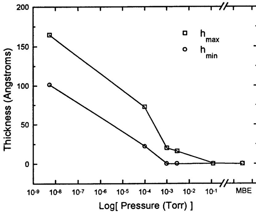
Minimum and maximum epitaxial thicknesses obtained from Si films grown by pulsed laser deposition at 3.0 J/cm<sup>2</sup> on dihydride-terminated Si(001) at 200 °C.
