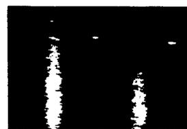
**Fig. 4** Spatially resolved CL images showing the emission from the first ( $\lambda = 790\text{nm}$ ) and second ( $\lambda = 804\text{nm}$ ) array of wire structures.
