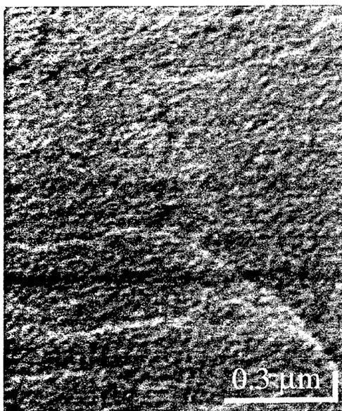
Fig. 3. GaAs (001) surface just after MBE growth (10 ML).
