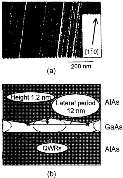
Fig. 1 : (a) AFM image of a GaAs surface of GaAs/AIAs QWRs grown on (775)B GaAs substrate.
