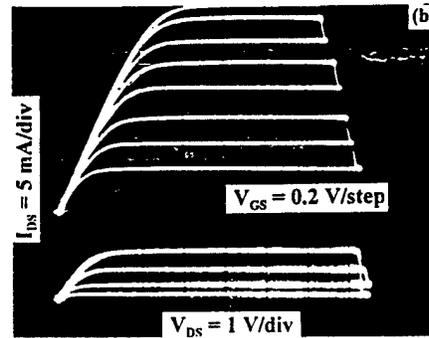
[Fig.3] (a) Forward drain-to-source I-V characteristics with  $V_{gs} = 0 \text{ V}$ . (b) Output I-V characteristics of a  $1 \times 100 \mu\text{m}^2$  TD-HFET. Note that the maximum  $V_{gs}$  is  $+1.4 \text{ V}$ .
