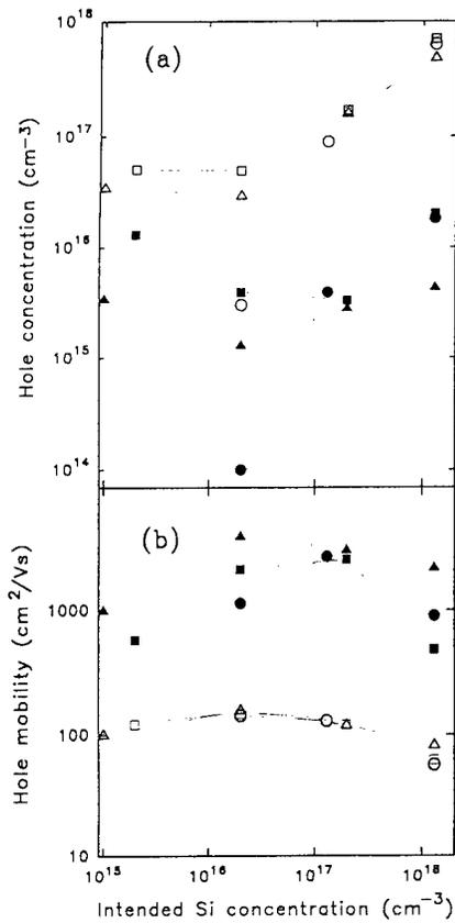
Fig. 1 - Free hole concentration (a) and hole mobility (b) as a function of the intended silicon concentration ( $N_i$ ) for (111)A (dots), (211)A (squares) and (311)A (triangles) samples. The filled and the open symbols refer to 77 K and 300 K data respectively. The (111)A sample with  $N_i = 1 \times 10^{15} \text{ cm}^{-3}$  is almost insulating, but still display a  $p$ -type conductivity. The lines through the data are only guide for the eyes
