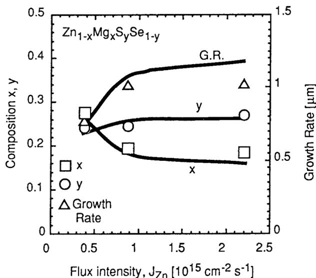
Figure 2 Zn flux intensity dependence of the mole fraction and the growth rate of experimental values (symbol) and calculated ones (curve) of ZnMgSSe.  $J_{Mg}$ ,  $J_S$ ,  $J_{Se}$  are 0.12, 0.19, 0.53 [ $10^{15} \text{ cm}^{-2} \text{ s}^{-1}$ ], respectively.
