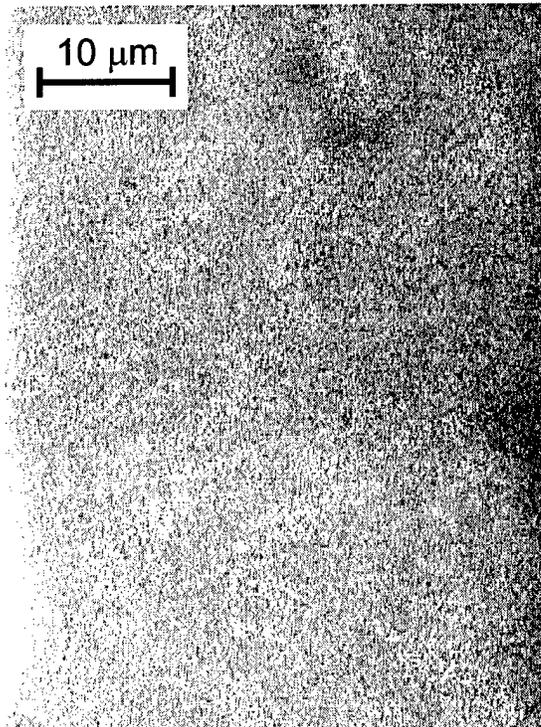
Figure 2) The room-temperature cathodoluminescence of a 1  $\mu\text{m}$  ZnSe film grown by MBE on a Zn-exposed  $(2\times 4)$  GaAs buffer layer at a magnification of 1700. Based on the observation that no defects were detected in the area shown, the defect density is less than  $2\times 10^5 \text{ cm}^{-2}$ . The electron probe parameters were: 30nA, 20kV.
