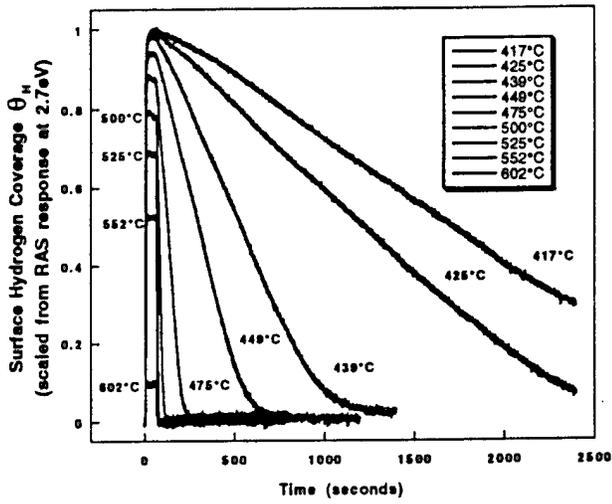
Isothermal H<sub>2</sub> Desorption Measurements
