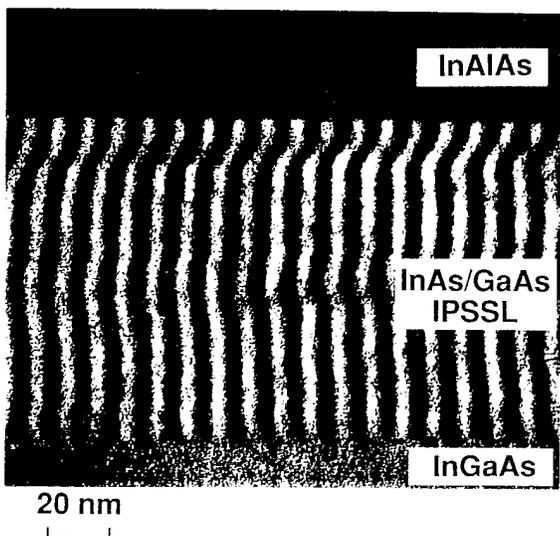
Fig. 3. TEM dark field image of the  $(1\bar{1}0)$  cross-section of the IPSSL grown on a substrate tilted at  $1.2^\circ$ .
