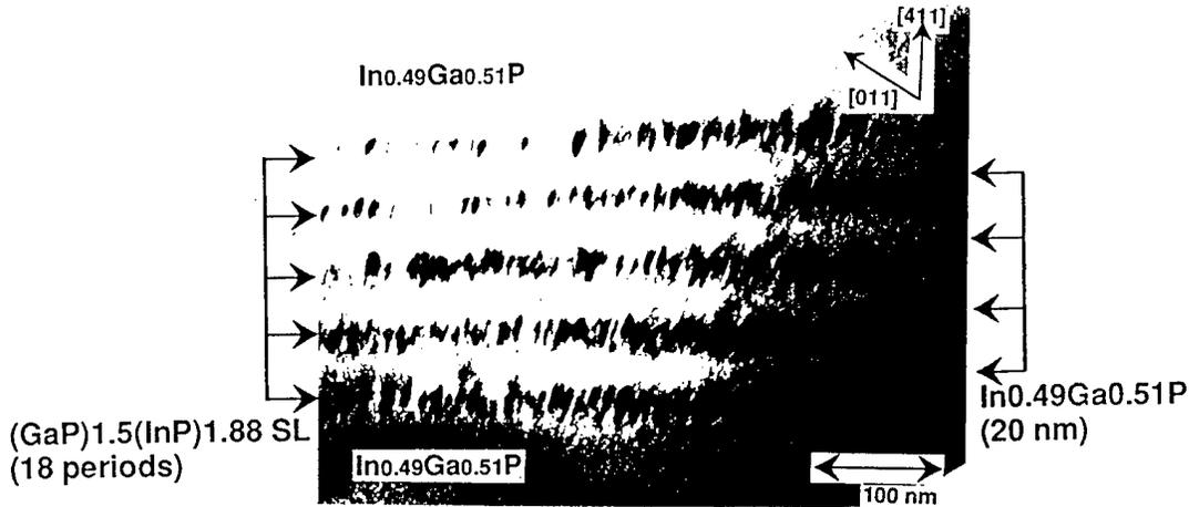
Fig. 2 (01-1) bright-field cross-sectional TEM image of the  $(\text{GaP})_{1.5}(\text{InP})_{1.88}$  SL/ $\text{In}_{0.49}\text{Ga}_{0.51}\text{P}$  quantum dot structure grown on GaAs(411)A. Both (011) and (01-1) cross-sectional TEM images showed the lateral composition modulation in the SL region.
