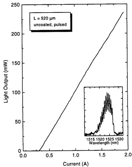
Fig. 3 Light-current curve for an as-cleaved broad-area laser. The inset shows the lasing spectrum at 150 mW.
