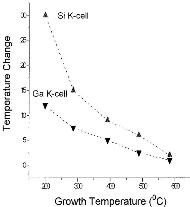
Figure 2. The Ga and Si Knudsen cells induced temperature change at various growth temperatures. The Ga and Si K-cells are at 1020 and 1180°C respectively. Corresponding to a growth rate of 1  $\mu\text{m/hr}$  and doping density of  $5 \times 10^{18}/\text{cm}^3$  respectively.
