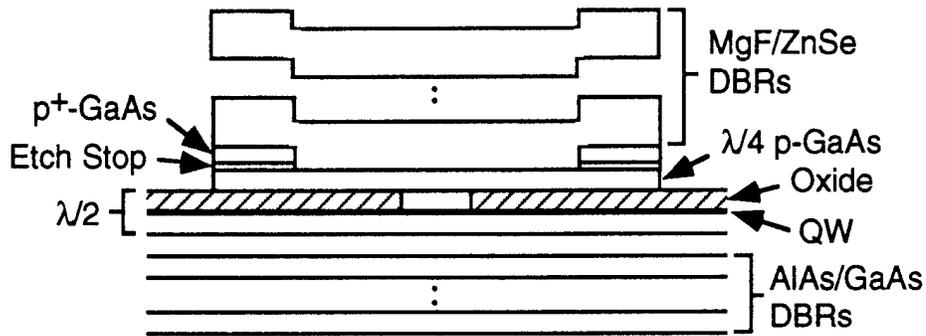
Figure 1: Schematic illustration of oxide VCSEL. The intracavity contact has been improved to remove the p<sup>+</sup>-GaAs contact layer from the cavity region and a low loss MgF/ZnSe DBR is used for the upper mirror.
