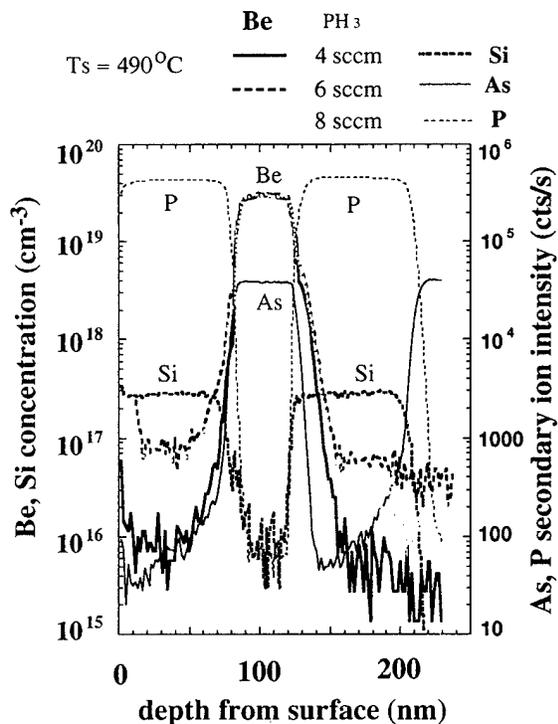
Phosphine flow-rate dependence of Be profiles in InGaAs/InP heterostructures
