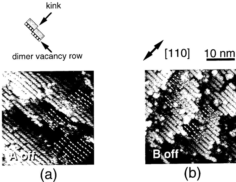
Fig. 1 STM images of vicinal GaAs (001) surfaces. Misorientation is  $1^\circ$  in (a) the [111]A direction and (b) the [111]B direction. Dotted lines are As dimer vacancy rows near the kinks in As dimer rows.
