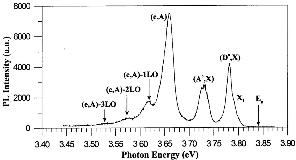
Fig. 3: Photoluminescence Spectrum of ZnS/GaAs at 10K
