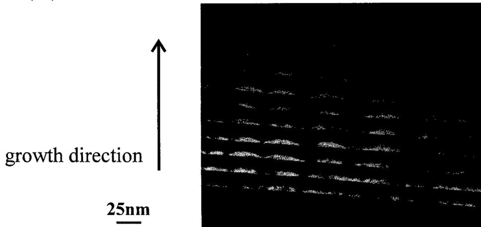
Fig.3 Cross-sectional TEM micrograph of a 10 periods GaInAs/InP MQW with  $x_{\text{Ga}} = 0.70$  grown on a (100) InP substrate  $2^{\circ}$  off towards [110].
