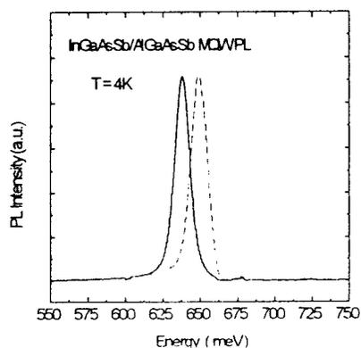
Fig 2. 4K photoluminescence spectra of InGaAsSb/AlGaAsSb MQW materials
