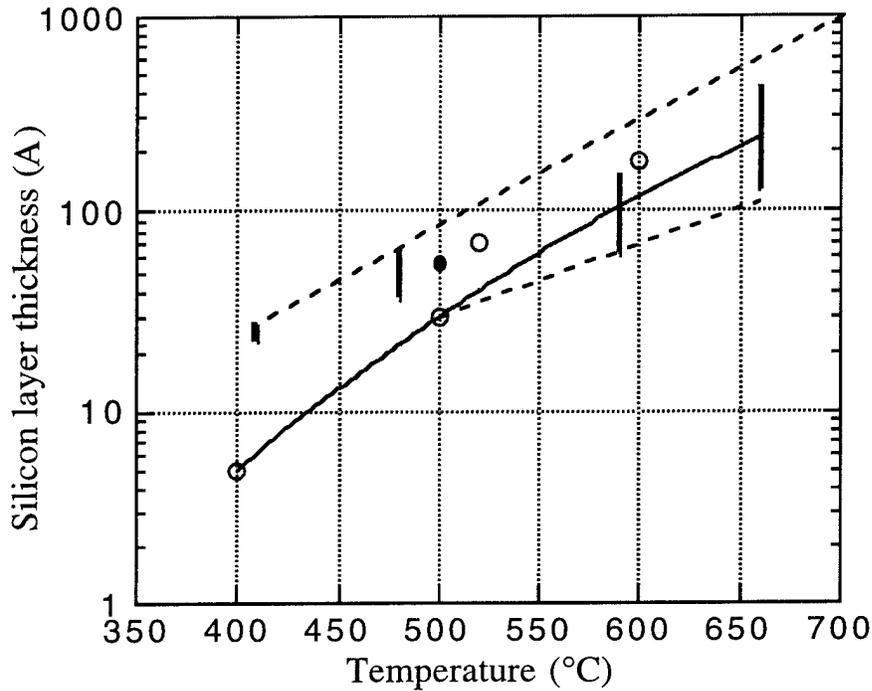
Fig. 1. The Si delta-doping layer thickness as a function of growth/annealing temperature. The thickness is higher for higher doping concentrations and the difference is more pronounced for higher temperatures.
