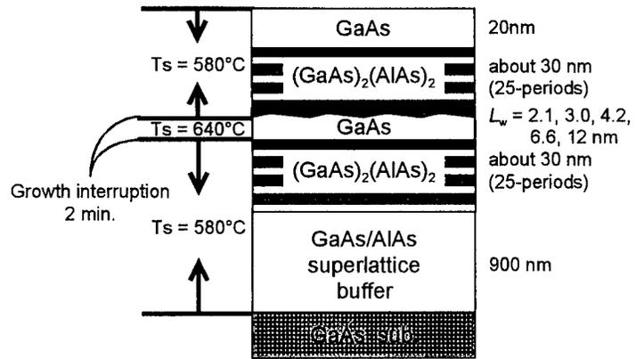
Fig. 2 : GaAs/ $(\text{GaAs})_2(\text{AlAs})_2$  QWRs (QWRs) structure grown on (775)B GaAs substrate.
