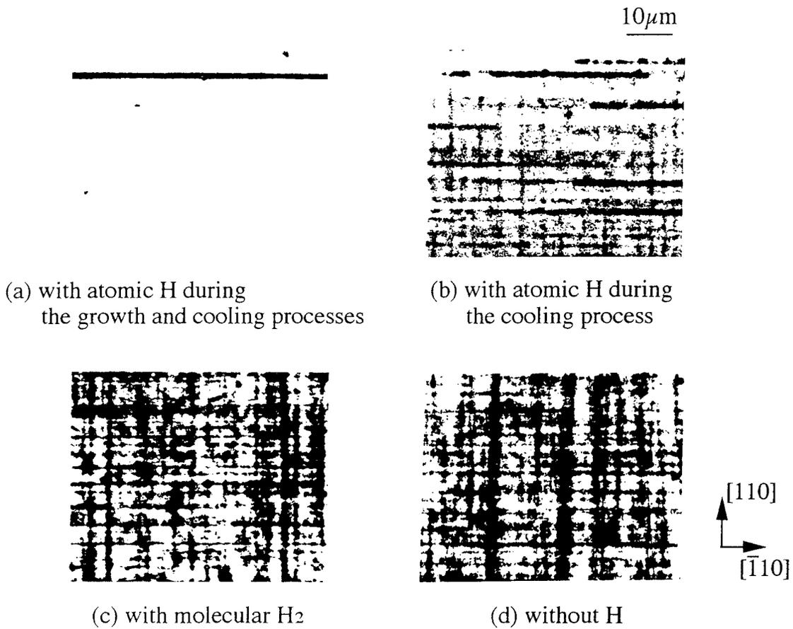
Fig. 3 EBIC images of  $(\text{InAs})_1(\text{GaAs})_4$  SSPS-on-GaAs(001). The dark line density was remarkably decreased by atomic hydrogen irradiation during the growth and cooling process rather than only cooling process, as shown in Figs. 3(a) and (b). On the contrary, the density was not reduced by molecular and no hydrogen irradiation, as shown in Fig. 3(c) and (d).
