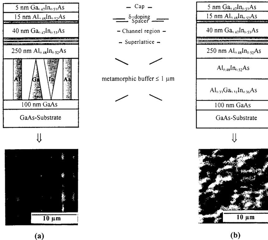
**Fig. 1.** MBE grown  $\text{Al}_{0.48}\text{In}_{0.52}\text{As}/\text{Ga}_{0.47}\text{In}_{0.53}\text{As}$  HEMT and buffer structure for linear (a) and stepwise (b) compensation of the lattice misfit. The Nomarski micrographs are shown underneath each layer structure.
