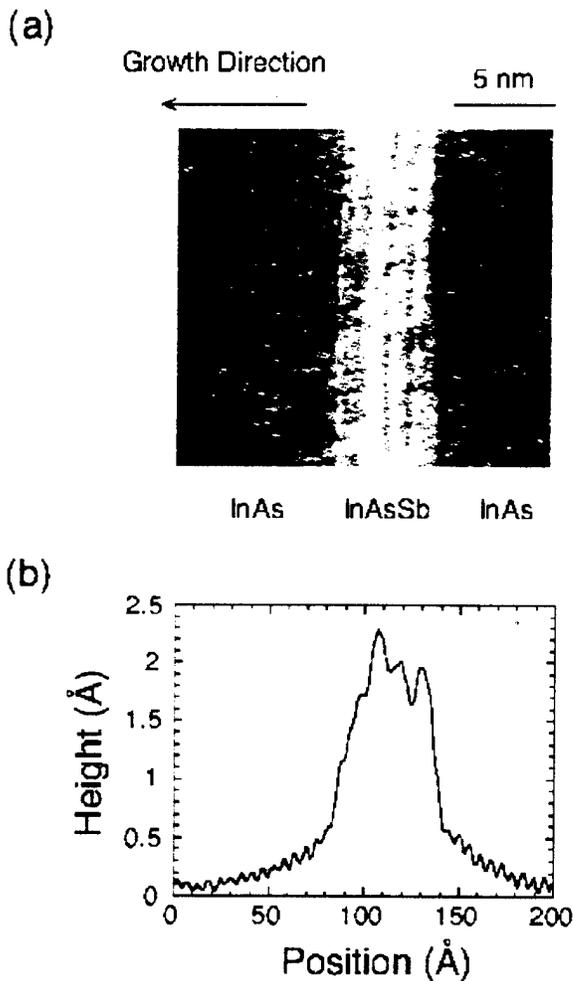
Fig. 1 (a) A high-resolution constant-current cross-sectional STM image of a single  $\text{InAs}_{0.76}\text{Sb}_{0.24}$  ordered-alloy layer surrounded by InAs. (b) An averaged topographic line scan of the layer and the surrounding InAs layers.
