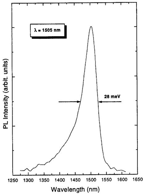
Fig. 1 Room-temperature photoluminescence from the laser structure.
