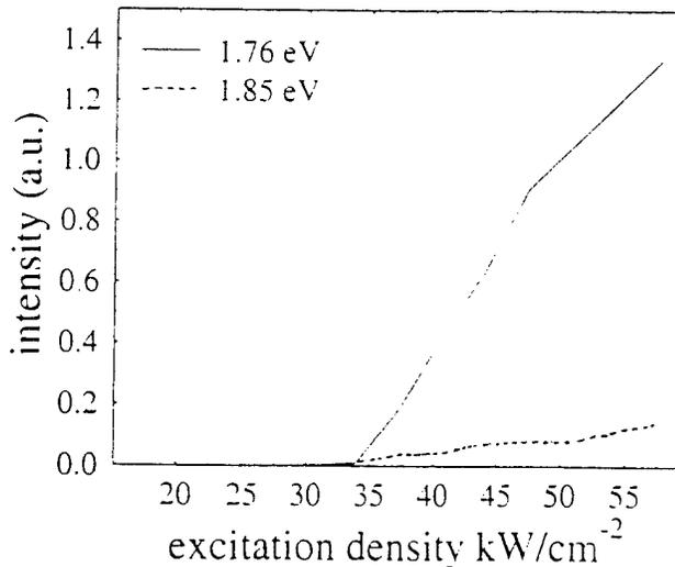
Figure 4: Emission spectrum of the laser structures shown in figure 3 showing the laser lines originating from the wetting layer and the InP quantum dots
