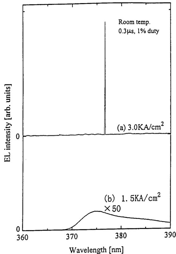
Fig.1 EL spectra from a diode with AlGaIn/GaN/GaInN SCH structure at a forward current of 3KA/cm<sup>2</sup>(a) and 1.5KA/cm<sup>2</sup>(b) , respectively.
