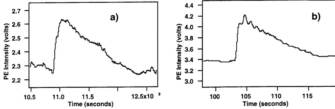
Figure 1. Photoemission oscillations measured during the growth of the GaSb well of an RTD grown on a) GaAs substrate; b) InAs substrate.
