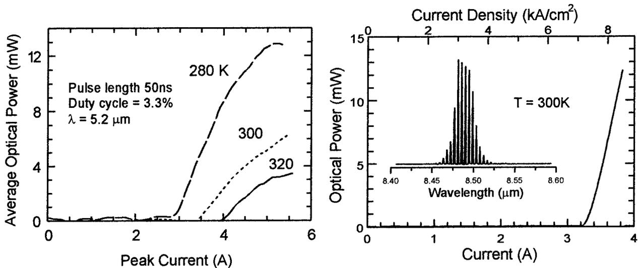
Fig. 2 Average power as a function of current for various temperatures. The pulse length is 50ns and the repetition rate is 670kHz.
