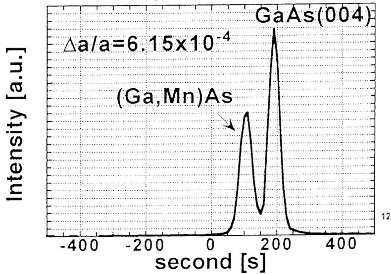
Figure 1: X-ray rocking curve of a  $(\text{Ga}_{1-x}\text{Mn}_x)\text{As}$  ( $x=0.02$ ) film with a thickness of 500 nm grown on a GaAs (001) substrate. The lattice mismatch to the GaAs substrate was 0.0615 %, which linearly increases with  $x$ .
