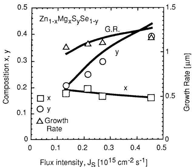
Figure 3 S flux intensity dependence of the mole fraction and the growth rate of experimental values (symbol) and calculated ones (curve) of ZnMgSSe.  $J_{Zn}$ ,  $J_{Mg}$ ,  $J_{Se}$  are 0.88, 0.13, 0.53 [ $10^{15} \text{ cm}^{-2} \text{ s}^{-1}$ ], respectively.
