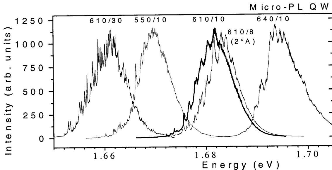
Fig.2. Micro-PL spectra of the quantum well emissions (normalized intensities).  $2^\circ\text{A}$  denotes the miscut of the (001) surface towards (111)Ga. All other substrates were unintentionally misoriented by  $0.03$ - $0.05^\circ$  towards (011).  $T_s$  and BEP-ratio of arsenic-to-gallium are indicated above each spectrum.
