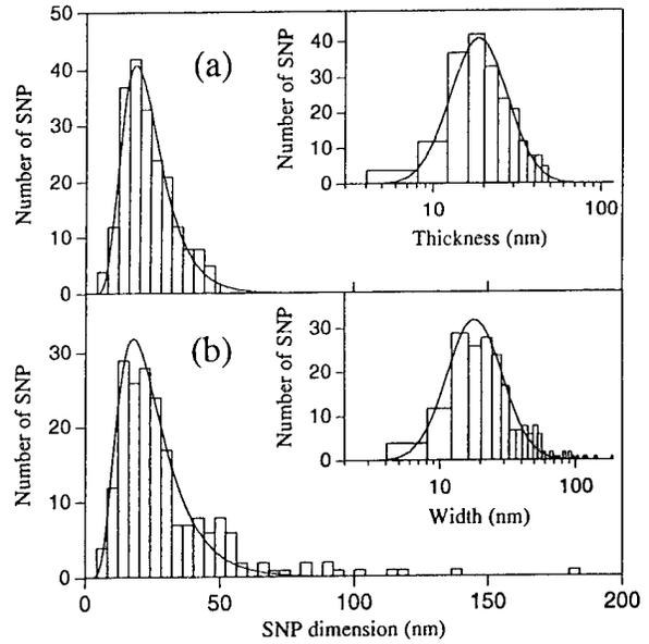
FIG. 2. Log-normal distribution of nanoparticle dimension. The insets are the semilog plots. Upper: Height. Lower: Width. Note the close similarity between the two distributions, and the ceiling over the height.
