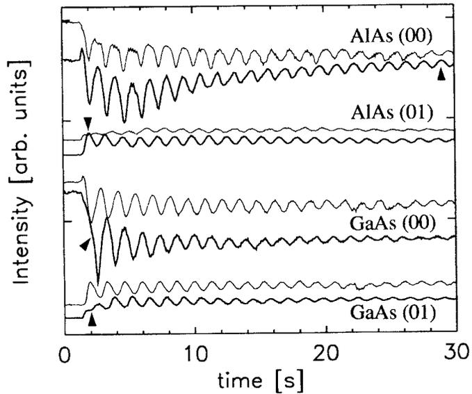
Figure 2: Evolution of the phase shift for the two interfaces on both the (00) and (01) streaks. Homoepitaxial references in green. The saturation distance is very large on the specular spot along  $[\bar{1}10]$ .
