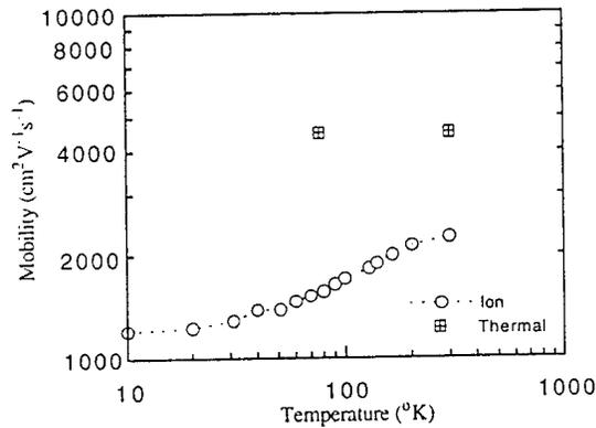
Figure 3. Hall mobility versus temperature for the 25eV Ga<sup>+</sup> FIB grown sample thermally doped with Si at a level of  $1.3 \times 10^{18} \text{ cm}^{-3}$  (note the logarithmic axes). For comparison a conventionally grown MBE n-GaAs sample is also shown. Both samples have a free carrier concentration of  $2.5 \times 10^{17} \text{ cm}^{-3}$
