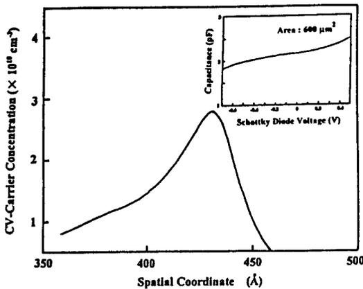
[Fig.2] Carrier concentration of our triple delta-doped epi-layer deduced from C-V measurements. The peak carrier concentration is  $2.8 \times 10^{18} \text{ cm}^{-3}$  and the measured capacitance is also depicted in the inset of figure.
