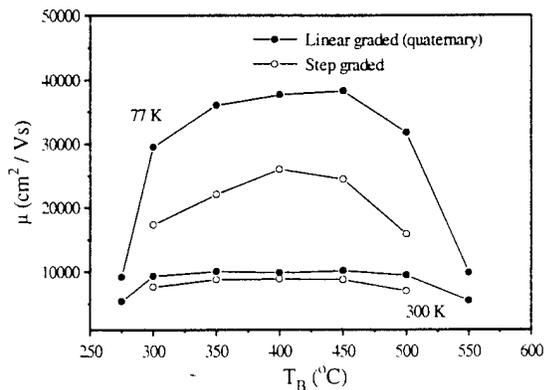
**Fig. 3.** Hall mobilities at 300K and 77K of  $\text{Al}_{0.48}\text{In}_{0.52}\text{As}/\text{Ga}_{0.47}\text{In}_{0.53}\text{As}$  HEMT structures grown on linear and step graded buffers as a function of the buffer growth temperatures.
