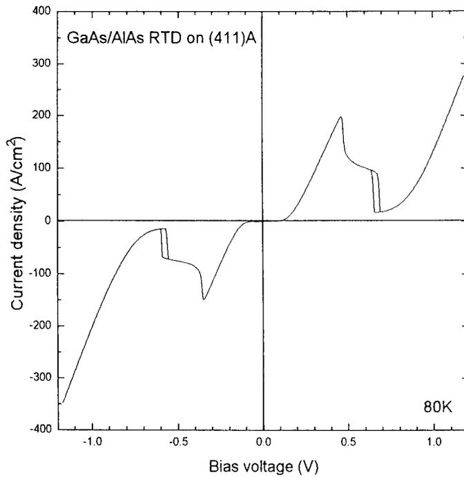
Fig. 1 I-V characteristics of a GaAs/AlAs RTD fabricated on a (411)A GaAs substrate with a contact area of  $120 \mu\text{m}$  in diameter.
