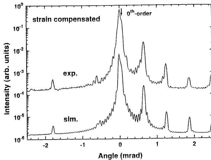
Fig. 1. Experimental and simulated rocking curves of a doped, 10-pair GaAs:C/AlAs:C DBR, which is strain-compensated with respect to the substrate.
