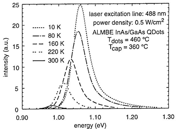
Fig. 4. Photoluminescence spectra at different temperatures of InAs/GaAs QDs grown by ALMBE at 460 °C; the upper confining layer has been grown at 360 °C by ALMBE. The dots have been deposited on a MBE GaAs layer grown at 560 °C, after a 210 s interruption. The spectral resolution is 1 meV.
