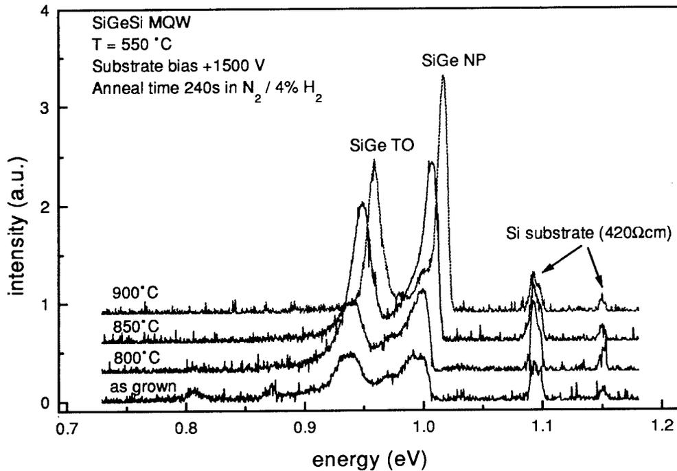
Fig. 1: Photoluminescence (4K) spectra of a Si<sub>0.76</sub>Ge<sub>0.24</sub>/Si multiple quantum well grown with an applied bias of +1500V to substrate. The figure compares the spectrum of the as grown MQW with those observed after rapid thermal annealing at 800, 850 and 950°C.
