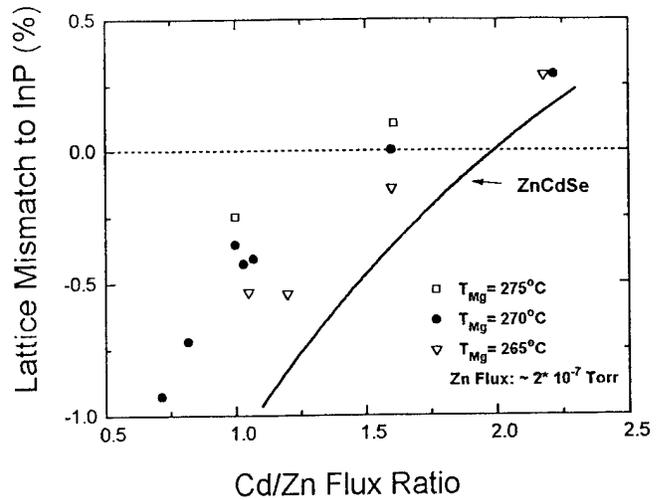
Fig.2. Lattice Constant Dependence on Cd/Zn Flux Ratio
