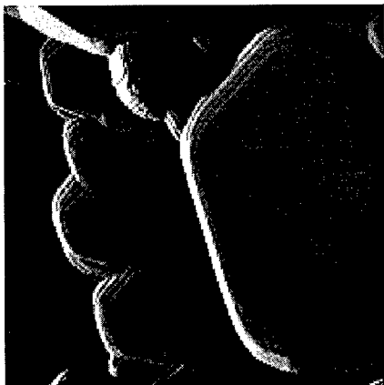
Fig. 9. STM image of a 500 nm x 500 nm area of Pb crystallites electrodeposited onto n-Si(111) from 0.05 M HClO 4 + 1 x 10 -3 M Pb 2+ . The sample and tip potentials were -860 and -340 mV vs. SCE, respectively. The tunneling current was 2 nA. The maximum height difference measured in the image was 90nm.
