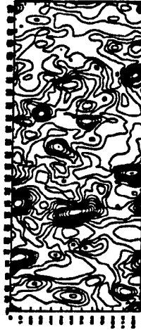
Figure 45: Contour map of the electrostatic potential over the simulation slab showing coherent structure that reflect the presence of strong plasma oscillations.
