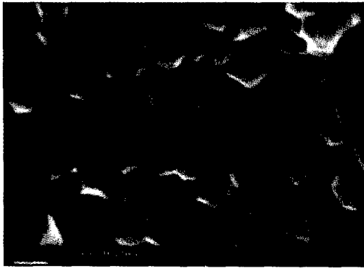
Figure 2. Fracture surface of an MgO-doped \text{Al}_2\text{O}_3 specimen sintered to 99.9% theoretical density in 10 minutes at 1400 °C.
