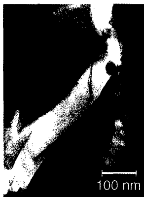
Figure 7 Two failure mechanisms often observed for crazes running parallel to silicate tactoids are shown here. Left: the craze fails by creating a void adjacent to silicate layers. Right: a silicate tactoid found in the propagation way of the craze "opens-up" and a void is created.
