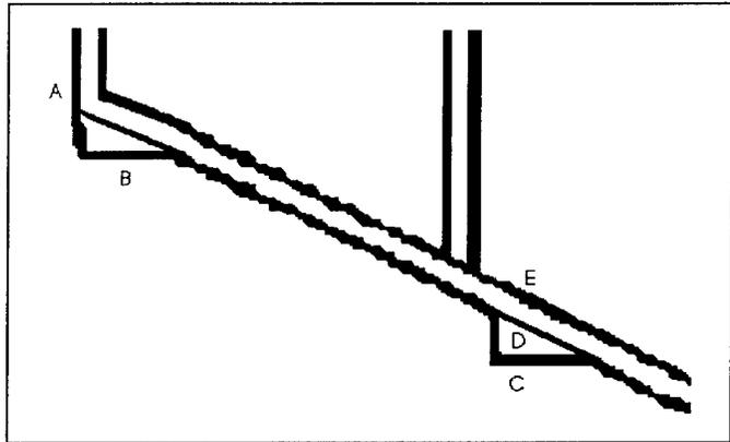
Figure 8: Thermocouple Locations
