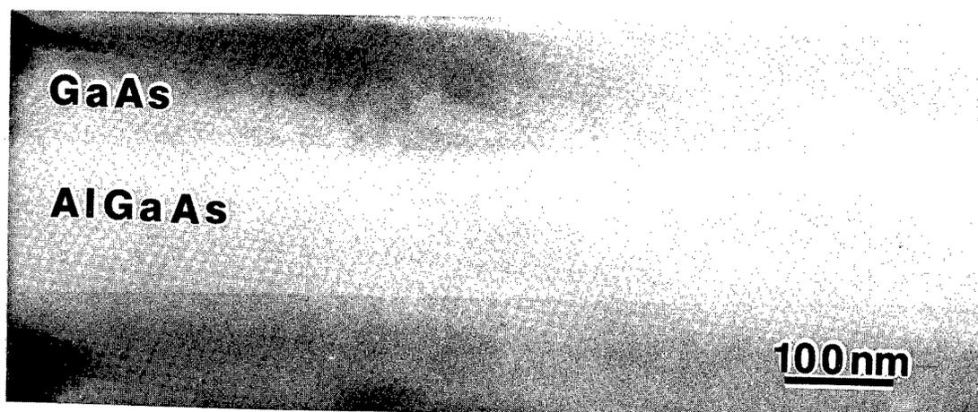
Figure 3. Bright field TEM micrograph showing inverted interface.
