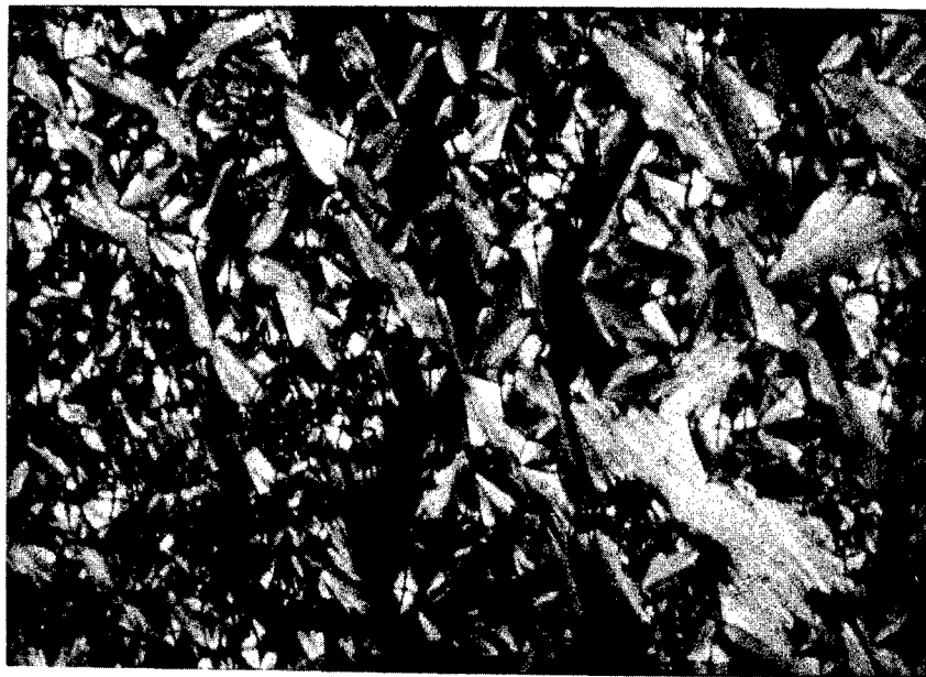
Figure 5. Optical micrograph of polymer II at 159°C. Crossed polarizers. Magnification 200X. Reference 11.
