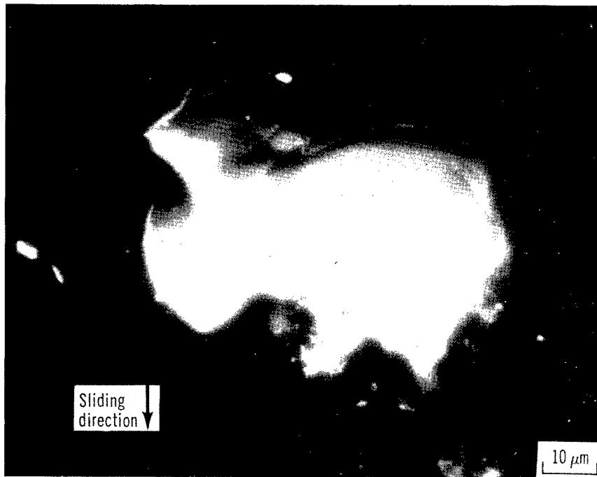
Figure 4. - Large fracture pit of single-crystal silicon carbide in contact with 8.12 atomic percent Ti-Fe alloy as a result of ten passes of rider in vacuum ( 10^{-8} Pa). A scanning electron micrograph of wear track on silicon carbide (0001) surface. Sliding velocity, 3 \times 10^{-3} meter per minute; load, 0.2 newton; room temperature.
