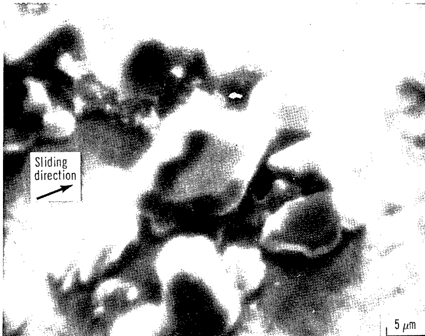
Figure 11. - Partially spherical wear particle and multiangular wear particles as result of ten passes of 1.02 atomic percent Ti-Fe alloy rider in vacuum ( 10^{-8} Pa). Scanning electron micrograph of wear scar on alloy rider. Sliding velocity, 3 \times 10^{-3} meter per minute; load, 0.2 newton; room temperature.
