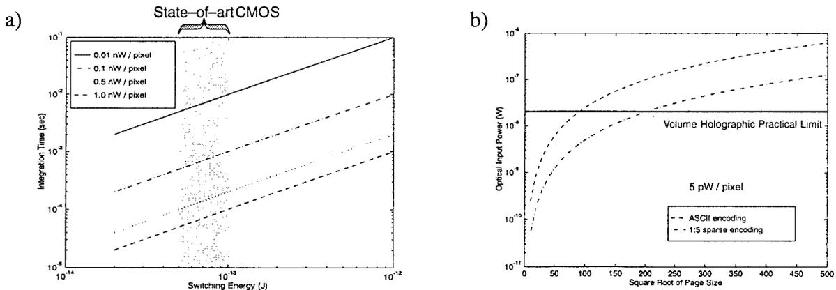
**Figure 28.** a) detector integration time vs. electrical switching energy
