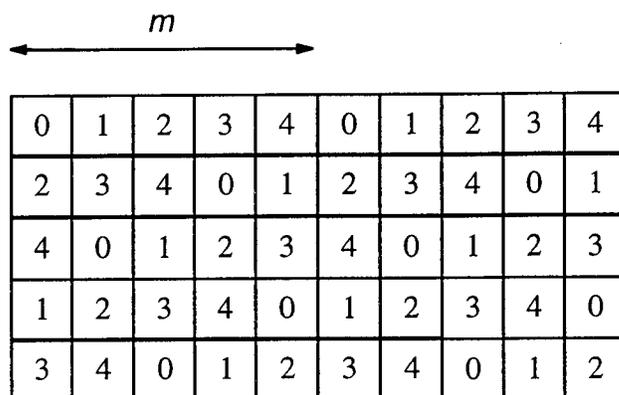
**Figure 13.** A 3-interleaved array with degree of interleaving 5.
