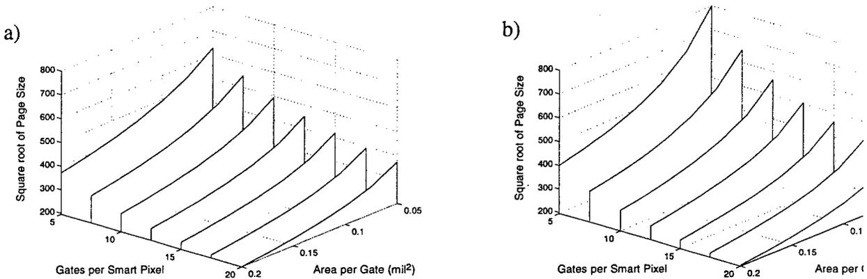
**Figure 27.** SPA page size vs. complexity vs. integration capability (SPA core area = 1 cm<sup>2</sup>)
