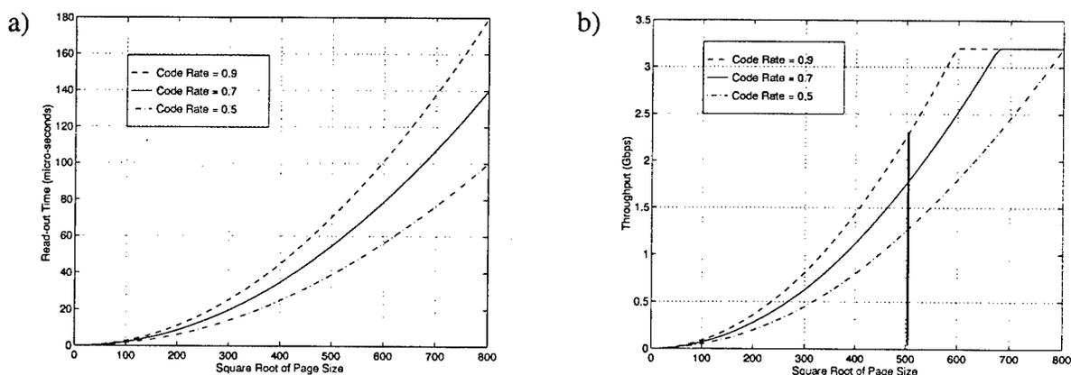
**Figure 30.** a) Array read-out time vs. page size
