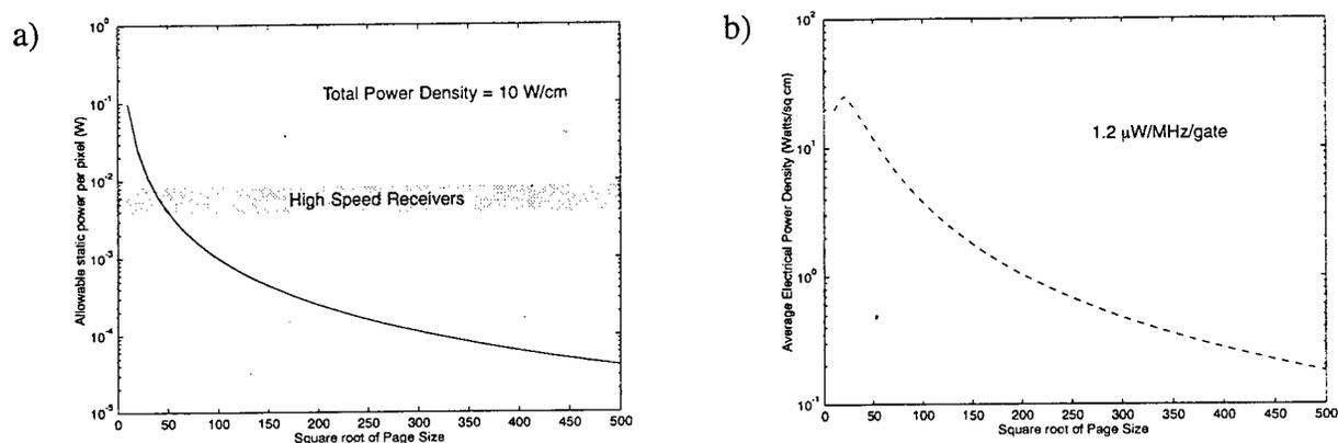
**Figure 29.** a) Static power per pixel vs. page size
