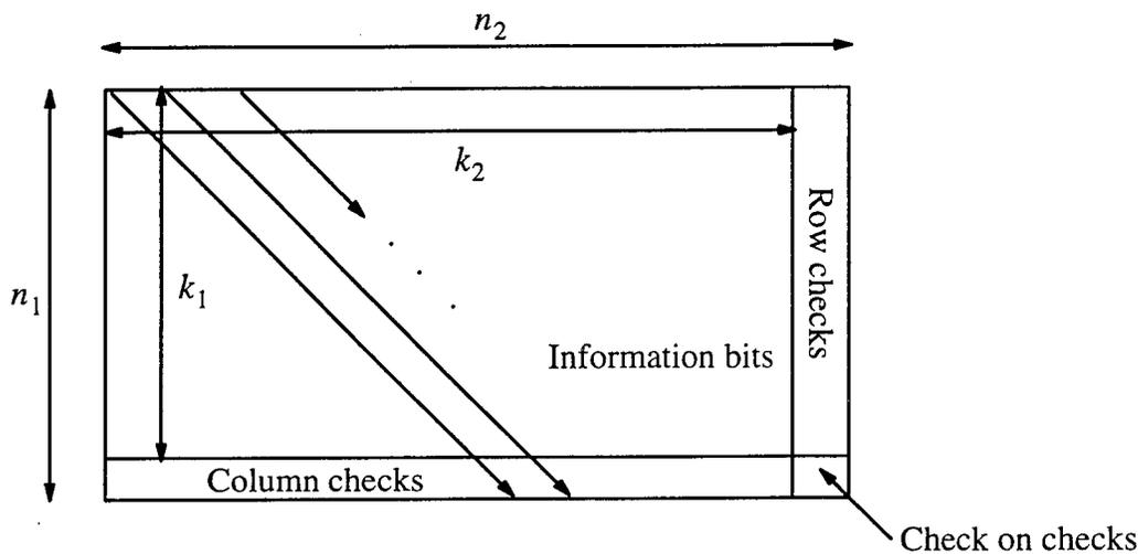
**Figure 10.** Single burst-correcting code and read-out pattern.
