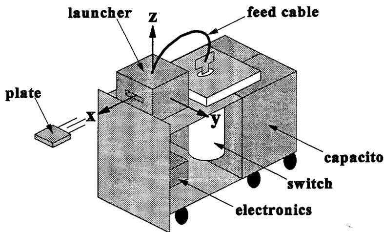
**Figure 7. The Test Stand Used in a Study of the EM Fields Generated by an Induction Launcher.**
