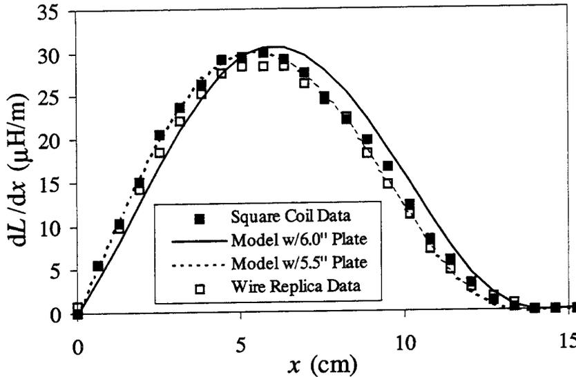
**Figure 5. Measured Inductance Gradient of a 6-in Square Pancake Coil Compared to the Results of Simulations Performed by the Program BFIELD10 (for Both the Actual 6-in Square Plate and a Hypothetical 5.5-in Square Plate). Also Included Are Data from a Narrow Gauge Wire Replica of the Coil.**
