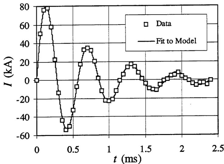
**Figure 2. A Typical Fit of Plate Launch Model Results to Measured Current Data.**
