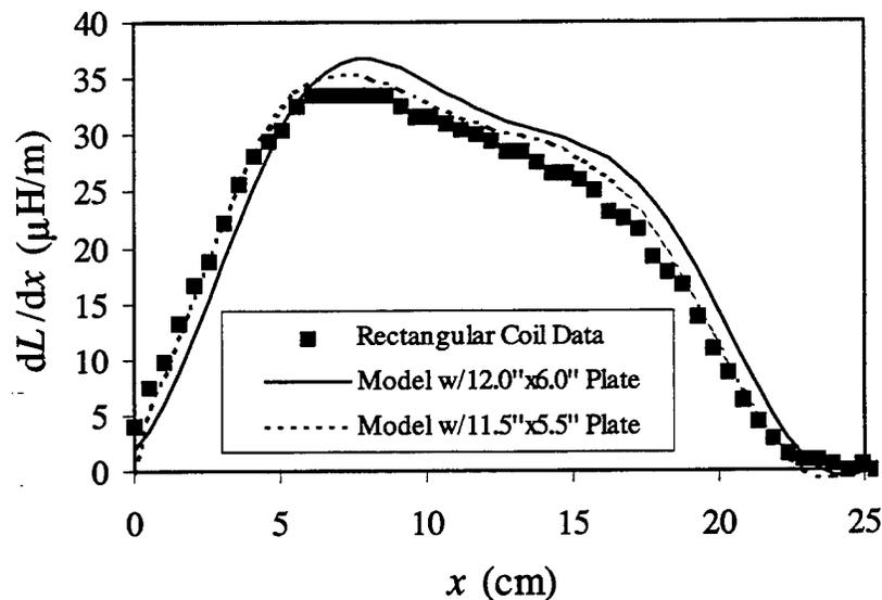
**Figure 6. Measured Inductance Gradient of a 10-in x 6-in Rectangular Pancake Coil Model Compared to the Results of Simulations (for Both the Actual 12-in x 6-in Plate and an 11.5-in x 5.5-in Plate).**
