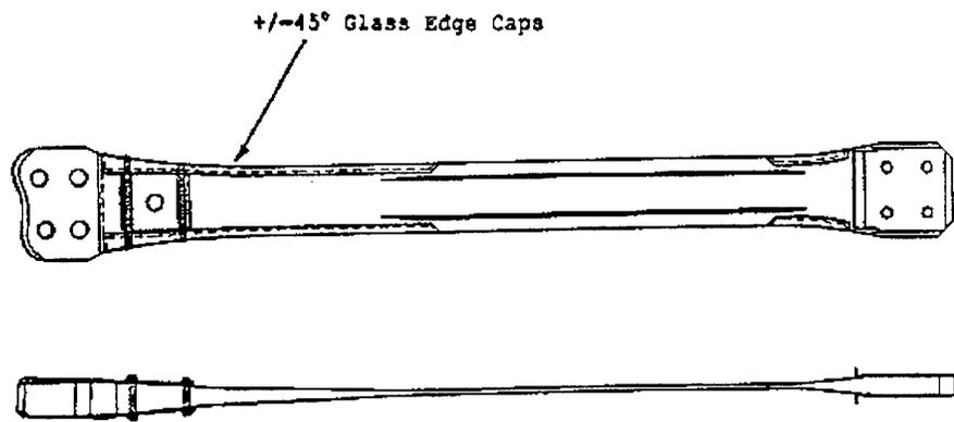
**Figure 3 RAH-66 COMANCHE Main Rotor Flexbeam Top and Side Views**
