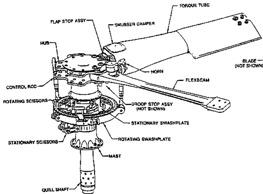
Figure 1 RAH-66 COMANCHE Main Rotor System
