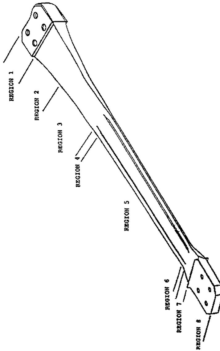
Figure 2 RAH-66 COMANCHE Main Rotor Flexbeam
