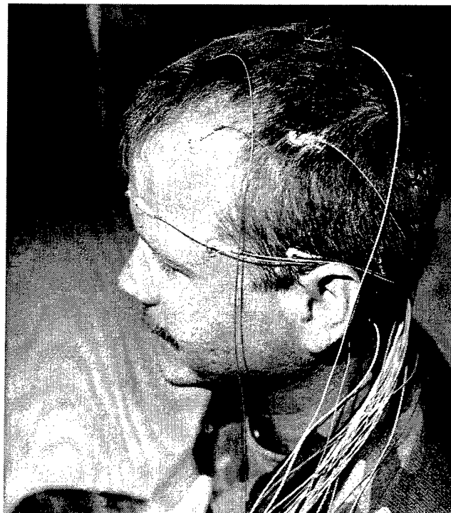
Figure 4. Electrode montage used for the collection of in-flight EEG data.
