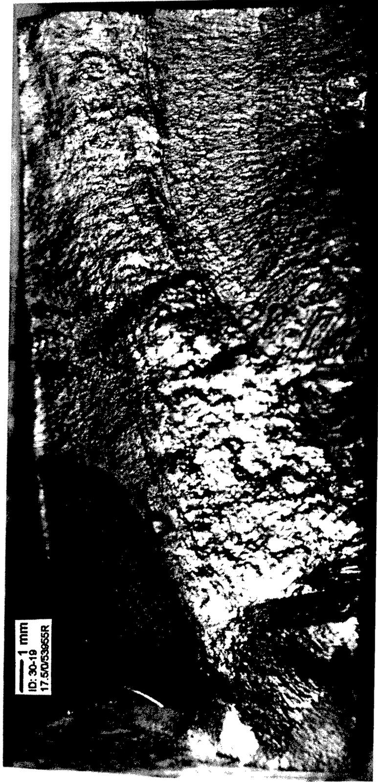
Figure A14. Fatigue fracture surface of the HSLA-80 but weld sample subjected to random loading:
