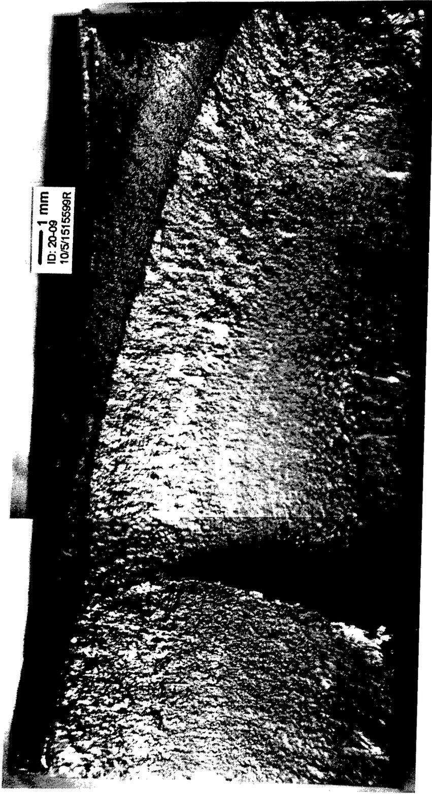
Figure A38. Fatigue fracture surface of the HSLA-80 but weld sample subjected to random loading:
