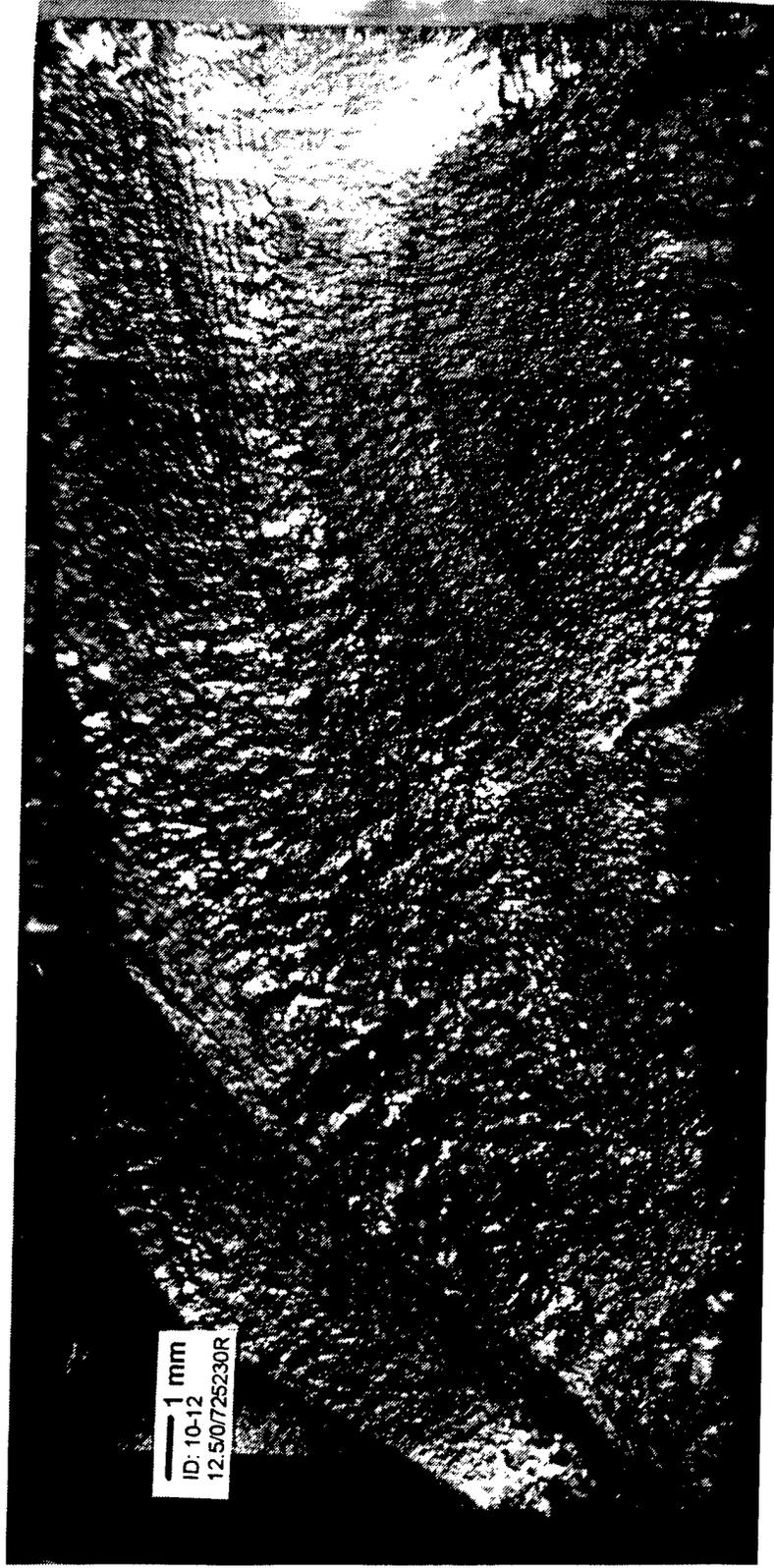
Figure A30. Fatigue fracture surface of the HSLA-80 but weld sample subjected to random loading:
