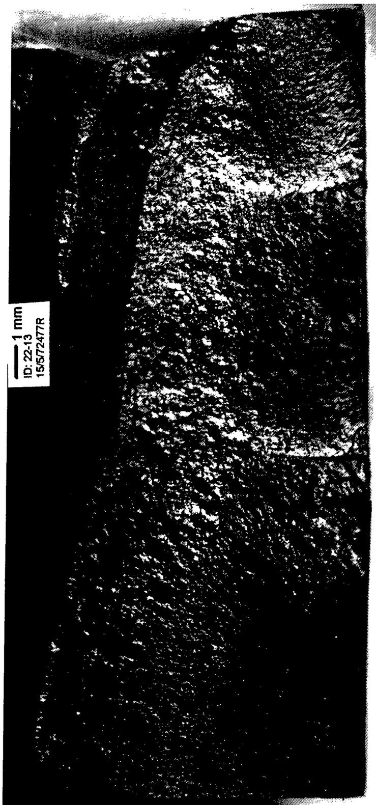
Figure A20. Fatigue fracture surface of the HSLA-80 but weld sample subjected to random loading:
