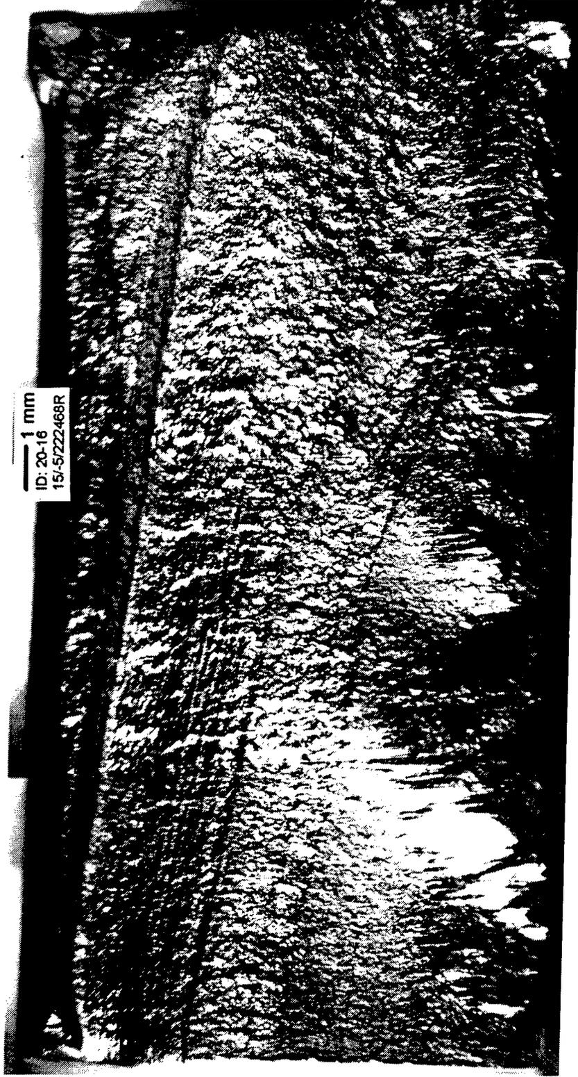
Figure A22. Fatigue fracture surface of the HSLA-80 but weld sample subjected to random loading:
