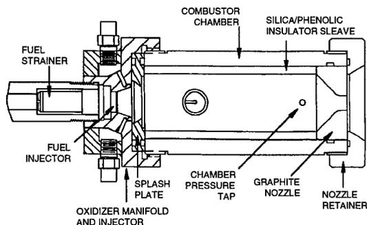
FIGURE 8. Line Drawing of Hypergolic Propellant Evaluation Thruster.
