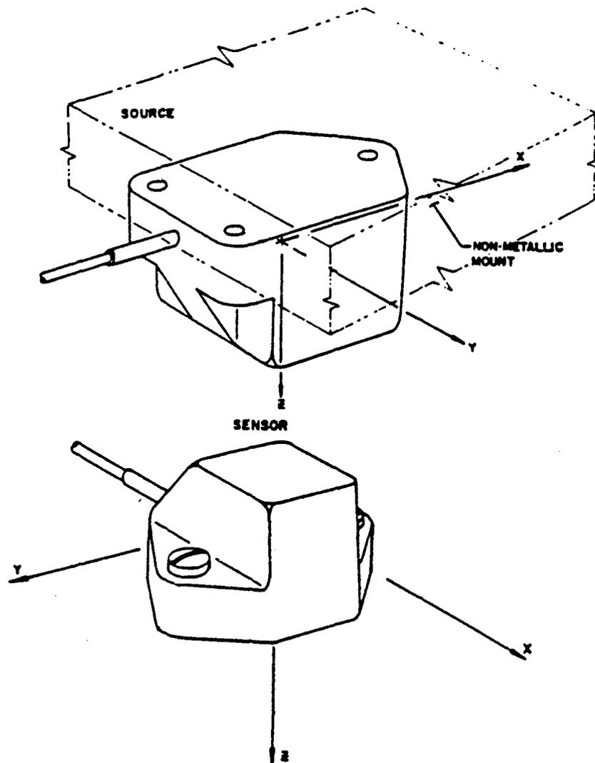
Figure 8.2. MAGNETRAK HMT Source and Sensor
