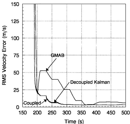
Figure 11. Velocity Errors for Frequent Data Loss.
