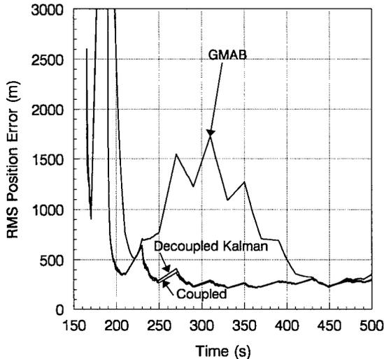
Figure 10. Position Errors for Frequent Data Loss.
