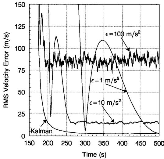
Figure 4. Velocity Errors for the Alpha-Beta Filter.
