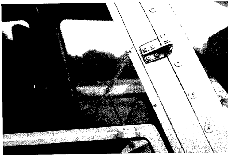
Fig. 3.3.2-4: Cracked cabin door window due to gun blast overpressure
