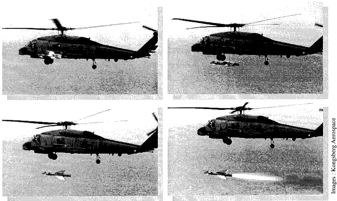
Figure 17 - Release Trials of Penguin ASuW Missile from Seahawk Helicopter
