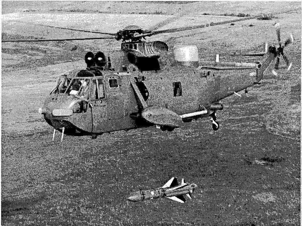
Figure 15 - Release Trials of Large ASuW Missile from Sea King Helicopter
