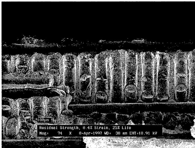
Figure 40. Fiber Failure, 0.4% Maximum Strain, 25% Expected Life
