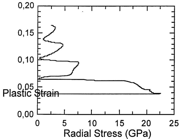
**Figure 19.** Accumulation of a total plastic strain in the middle cylindrical layer of a ceramic tube sample during 2.5  $\mu$ sec of cylindrical shock loading.
