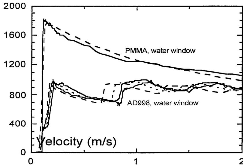
**Figure 17.** Comparison of measured and calculated velocity profiles of shock waves created in the PMMA and AD998 tube samples by cylindrical detonation. Measurements with water windows.
