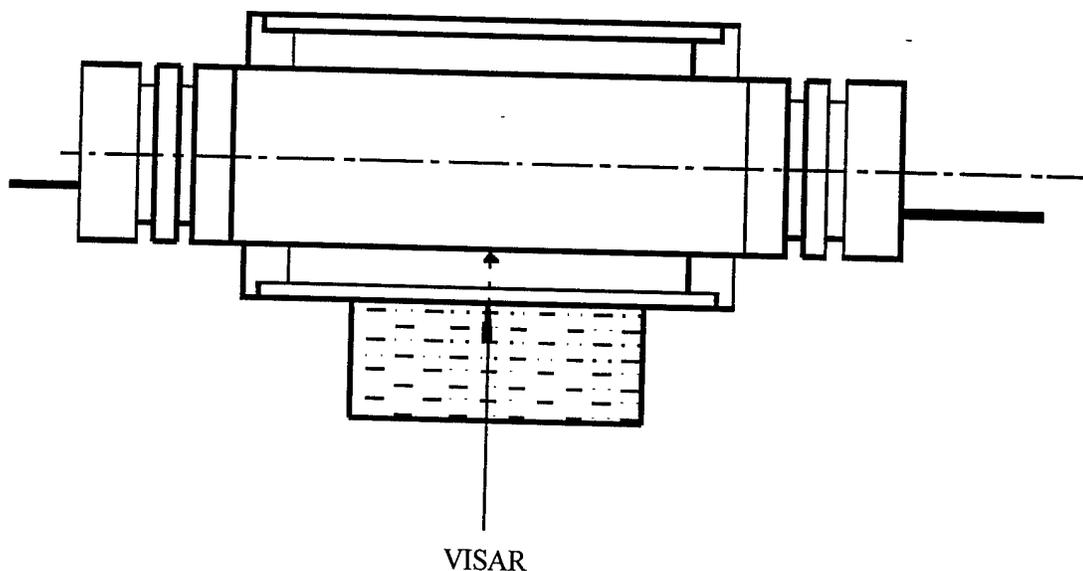
**Figure 1.** Scheme of recording of the free-surface velocity history or particle velocity history at the interface between the tube sample and LiF or water window. The cylindrical shock wave is created by detonation of an RDX charge initiated by an electrical explosion of a wire on the charge axis.
