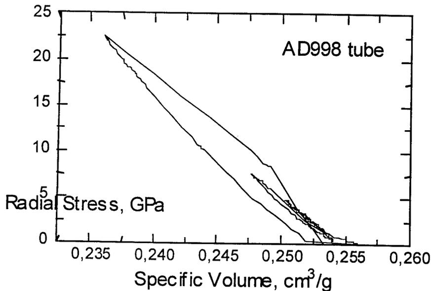
**Figure 18.** Trajectory of the changing state of a middle cylindrical layer of the ceramic tube sample. Results of computer simulation with large strain softening.
