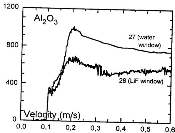
**Figure 16.** The particle velocity profiles for ceramic tubes at different window materials.
