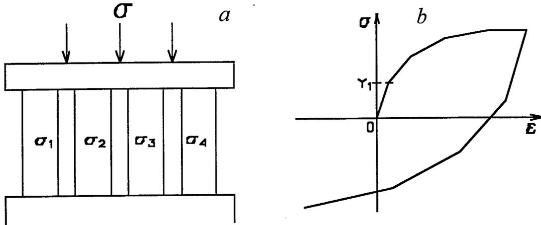
**Figure 2.** The structural multi-elements Marzing model (a) and its stress-strain diagram (b).
