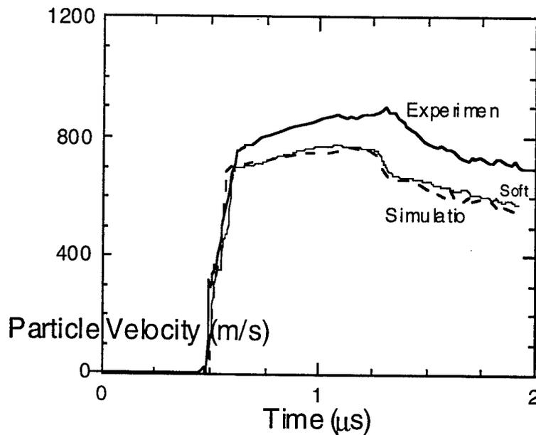
**Figure 20.** Measured and computed VISAR velocity profiles of the AD998 tube sample impacted by the stainless tube liner. Measurements with a water window.
