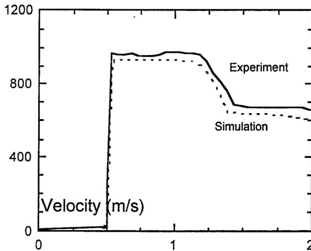
**Figure 14.** Impact of the stainless steel liner upon the aluminum tube target. The liner is 24 mm in the incident inside diameter and 30 mm in outside diameter. The target is 42 mm in outside diameter and 37 mm in inside diameter. The velocity of the target surface is measured with a water window.
