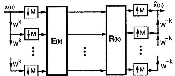
Fig. 3. Polyphase form of the cyclic filter bank.
