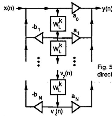
Fig. 5. The cyclic direct form structure.
