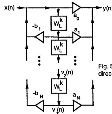
Fig. 5. The cyclic direct form structure.
