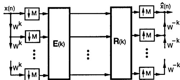
Fig. 3. Polyphase form of the cyclic filter bank.
