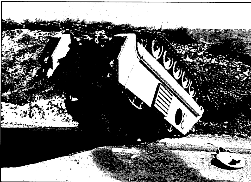
The driver of this M981 lost control as the vehicle was descending a 7° slope, turned to the left and ran upon an embankment. The vehicle overturned resulting in one fatality, three soldiers injured and vehicle damage.
