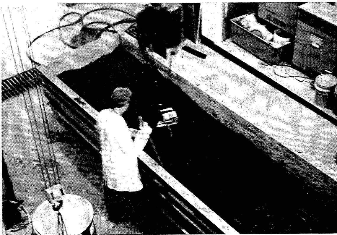
Figure 9. Mixing soils from LL2A in a soil lysimeter
