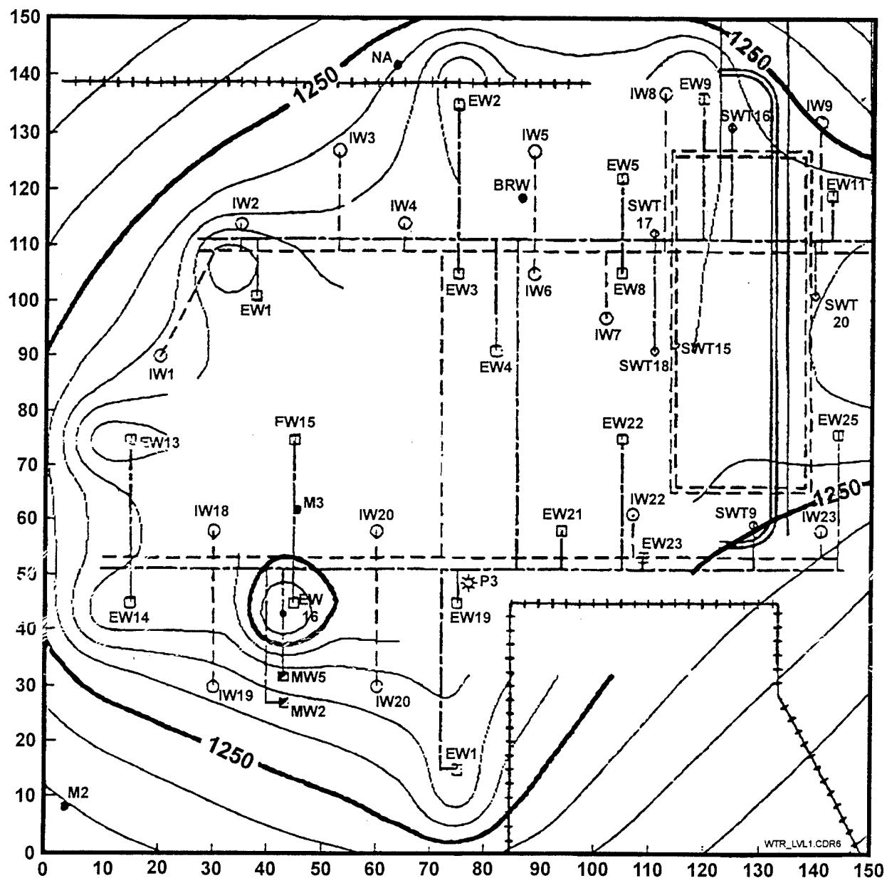
Figure 11. Map of Predicted Water Level After 35 Days of Pumping at 0.5 gpm/Well
