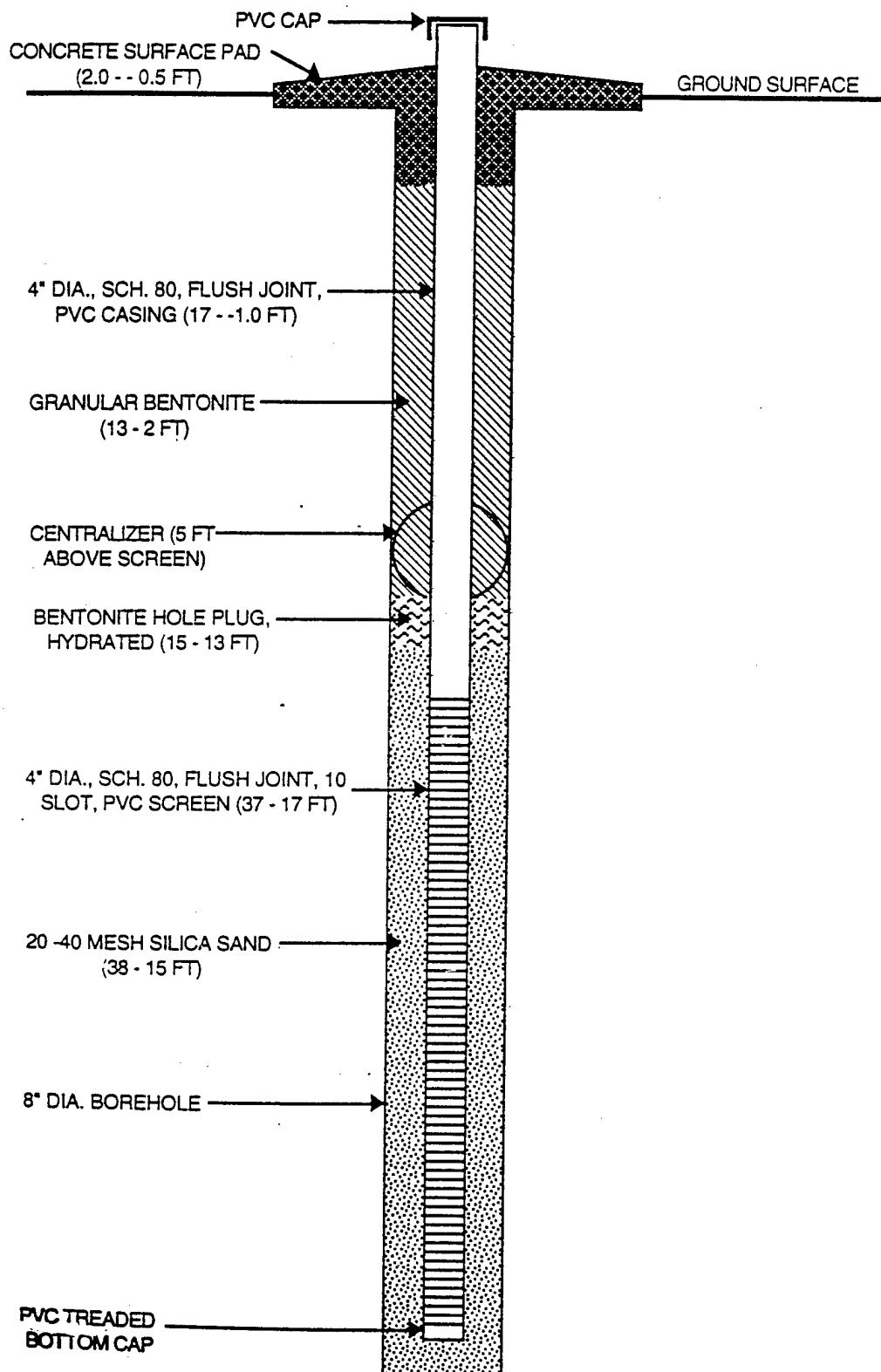
Figure 4. Schematic Diagram of a Typical Bioslurper Well
