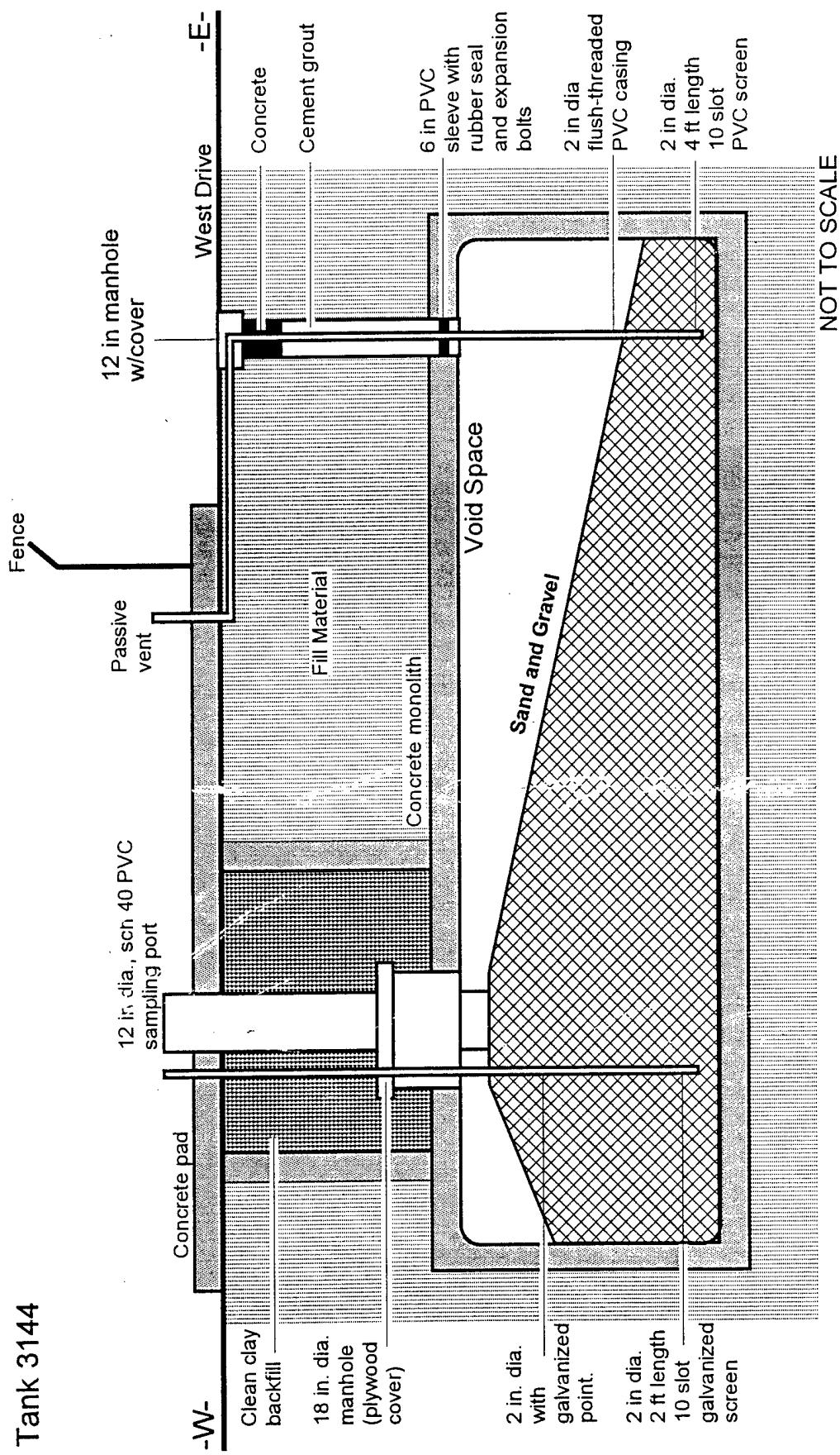
Figure 1. Cross Section of Tank 3144 Showing Construction Details of Installations
