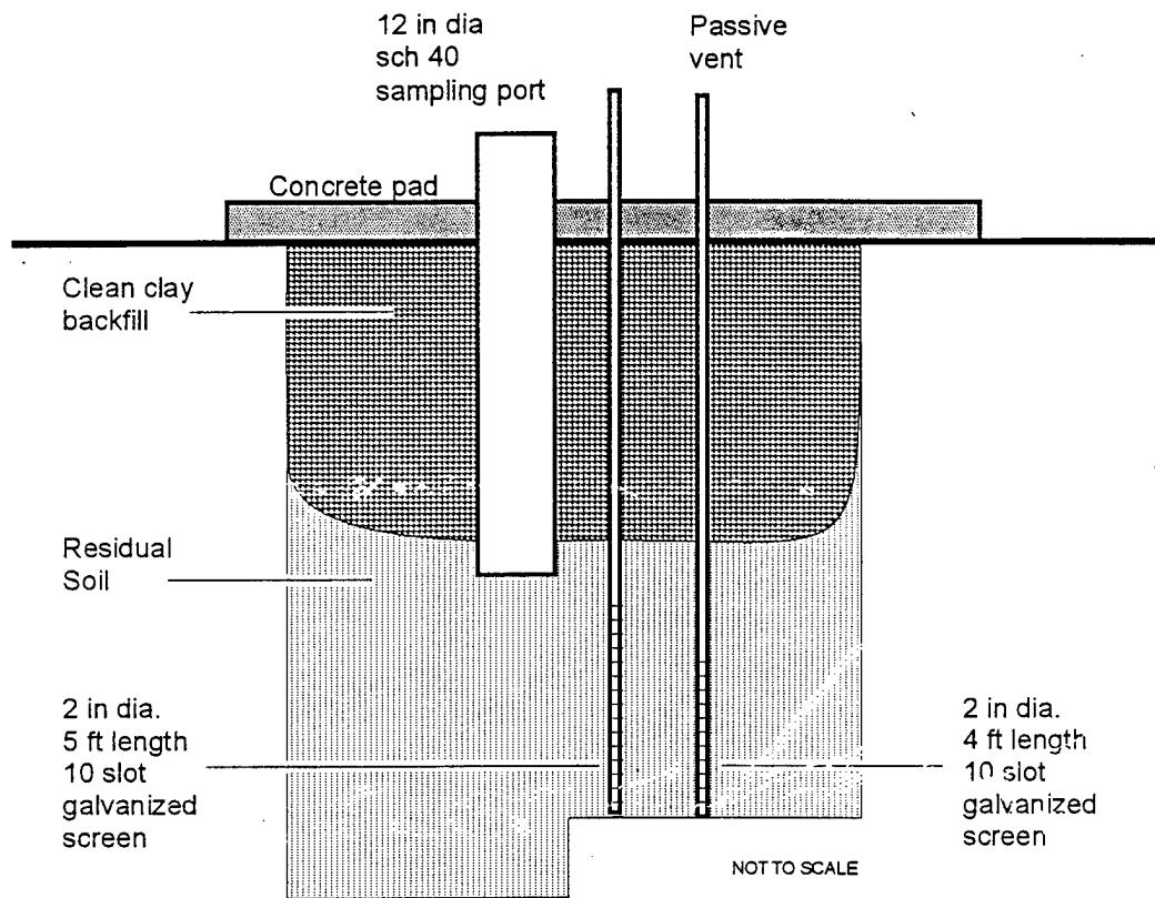
Figure 2. Cross Section of the Sump Area Showing Construction Details of Installations
