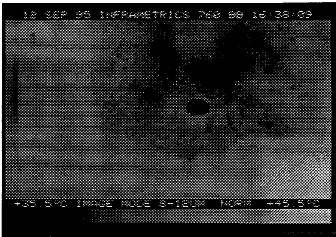
Figure 5-24. Thermal Image of Area B: taken at 1714 hours; ambient temp: 32.0°C; surface temp: 36.3°C; temp inside hole: 34.7°C; 1X telescope lens
