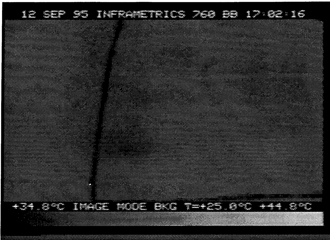
Figure 5-26. Thermal Image of Area E: taken at 1738 hours; ambient temp: 32.6°C; surface temp: 36.3°C; 1X telescope
