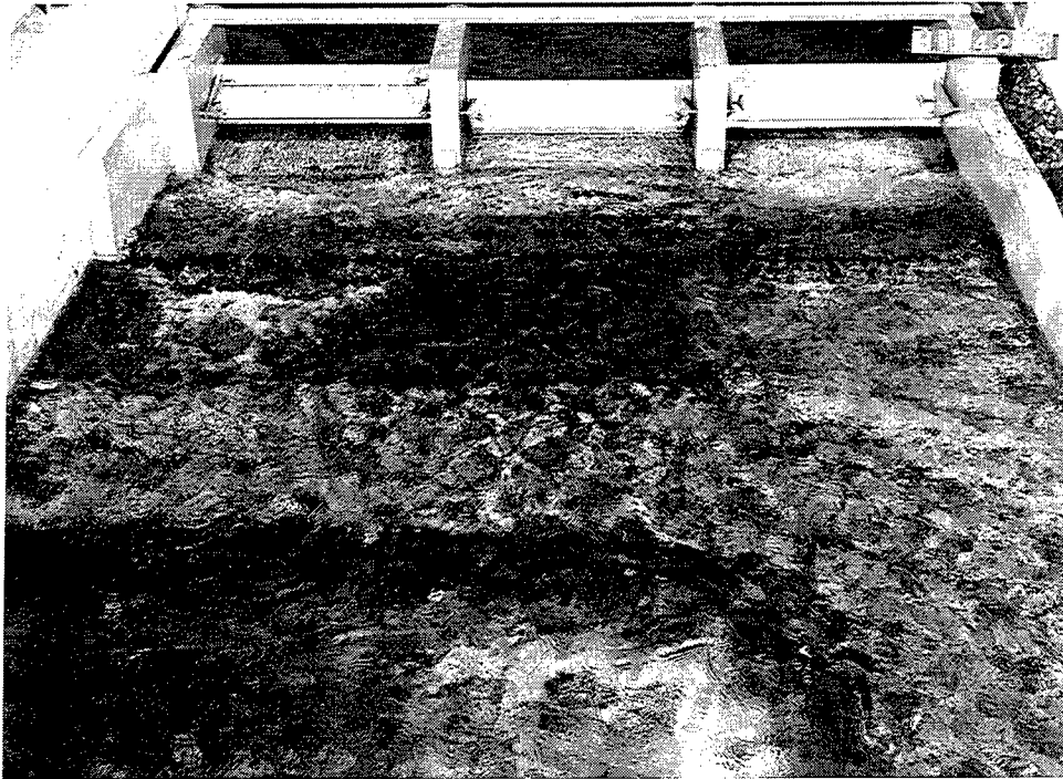
Photo 24. Type 3 riprap/rock apron, configuration 2; Q = 538 cu m/sec (19,200 cfs); G_3 = 1.8 m (6 ft), G_4 = 0 , G_5 = 1.2 m (4 ft); upper pool el 743.5; tailwater el 728.9
