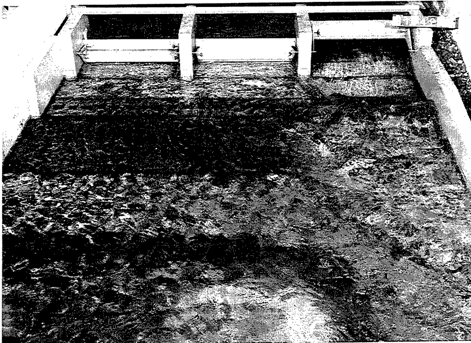
Photo 25. Type 3 riprap/rock apron, configuration 2; Q = 574 cu m/sec (20,500 cfs); G_3 = 0 , G_4 = 0 , G_5 = \text{full} ; upper pool el 743.5; tailwater el 729.0
