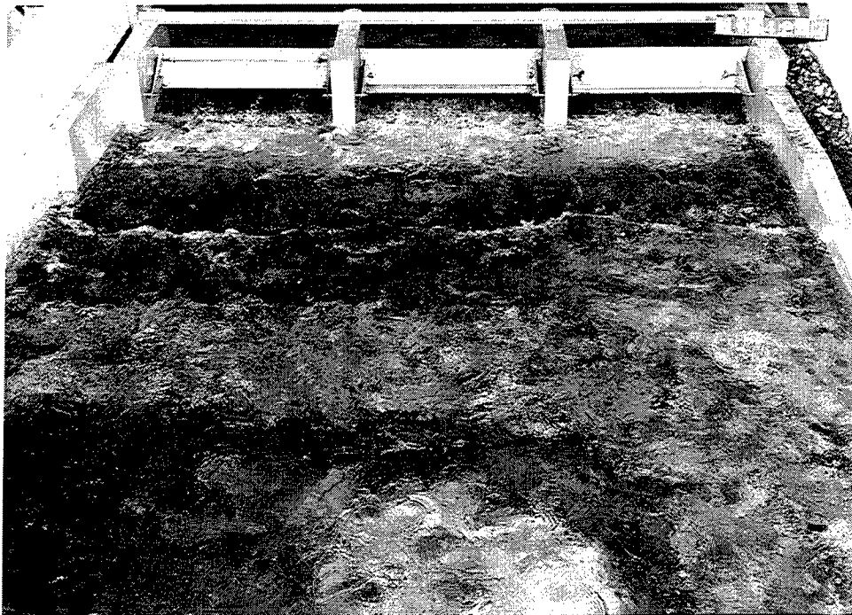
Photo 33. Type 3 riprap/rock apron, configuration 2; Q = 1,366 cu m/sec (48,800 cfs); G_3 = 3.6 m (12 ft), G_4 = 3.0 m (10 ft), G_5 = 3.0 m (10 ft); upper pool el 743.5; tailwater el 737.1
