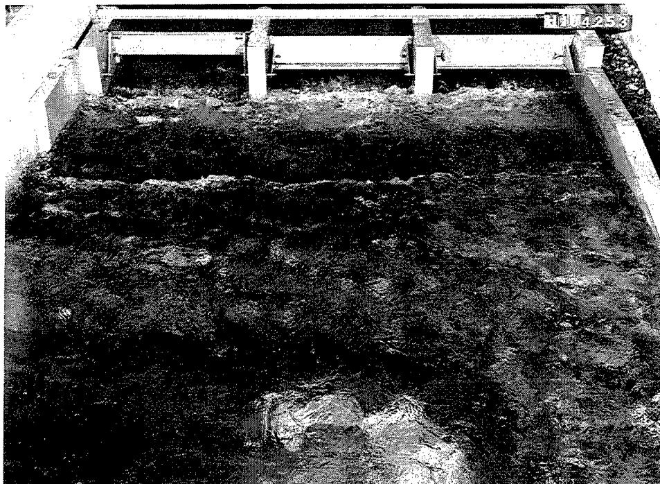
Photo 34. Type 3 riprap/rock apron, configuration 2; Q = 1,537 cu m/sec (54,900 cfs); G_3 = \text{full} , G_4 = 3.6 m (12 ft), G_5 = 3.6 m (12 ft); upper pool el 743.5; tailwater el 739.0
